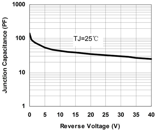
Fig.1-Typical Junction Capacitance
