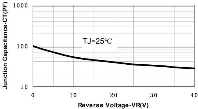
Fig.1-Typical Junction Capacitance
