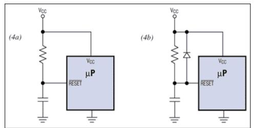
Figure 4. The discrete R/C POR (Figure 4a) is not reliable enough for most applications. In some cases,
