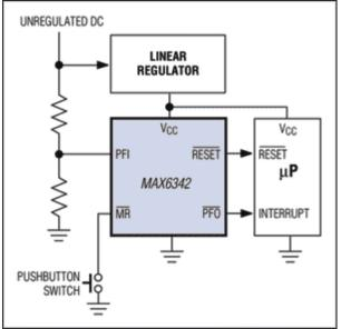
Figure 5. The power-fail comparator within the MAX6342 generates the power-fail signal (PFO-bar) by monitoring whether the unregulated DC supply has dropped.
