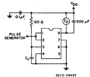
Fig. 7 — Power-dissipation test circuit for CD40107BE.
