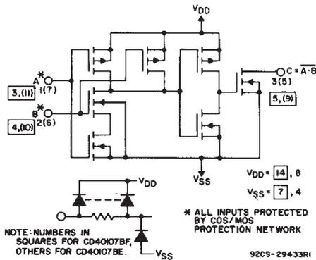
Fig.1 – Schematic diagram of CD40107B (one of 2 gates)
