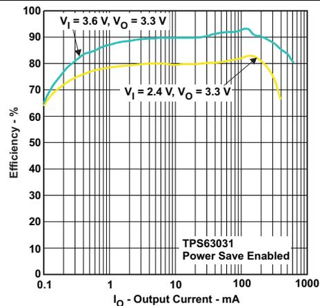
Figure 9. Efficiency versus Output Current, TPS63031, Power-Save Enabled
