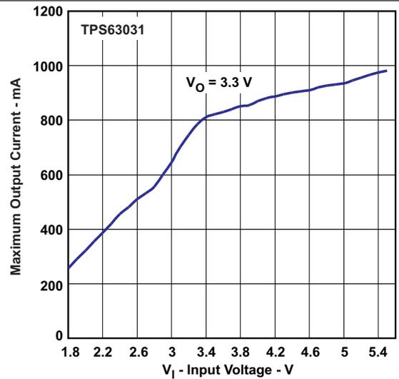
Figure 2. Maximum Output Current versus Input Voltage, TPS63031
