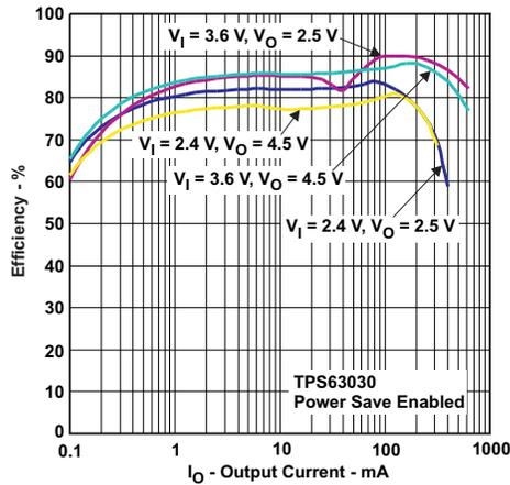
Figure 7. Efficiency versus Output Current, TPS63030, Power-Save Enabled
