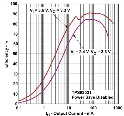
Figure 10. Efficiency versus Output Current, TPS63031, Power-Save Disabled
