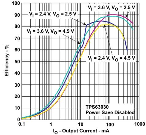
Figure 8. Efficiency versus Output Current, TPS63030, Power-Save Disabled
