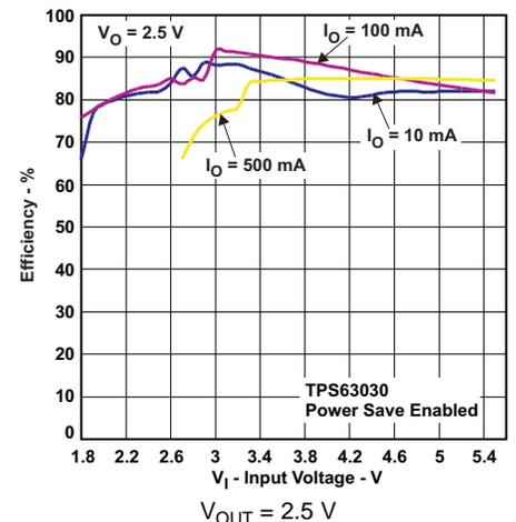
Figure 11. Efficiency versus Input Voltage, TPS63030, Power-Save Enabled
