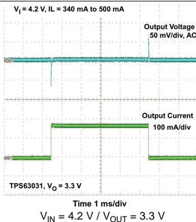
Figure 21. Load Transient Response, TPS63031
