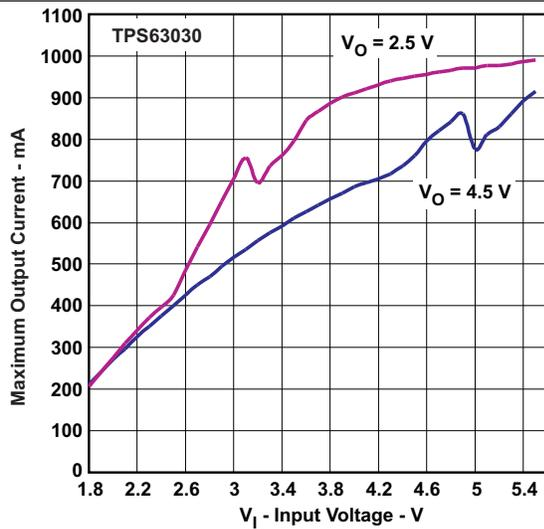
Figure 1. Maximum Output Current versus Input Voltage, TPS63030
