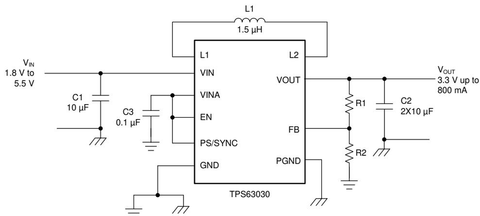
**Figure 5. Typical Application Circuit for Adjustable Output Voltage**
