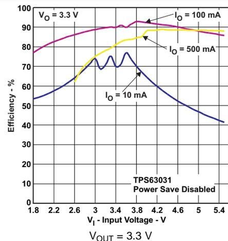
Figure 16. Efficiency versus Input Voltage, TPS63031, Power-Save Disabled
