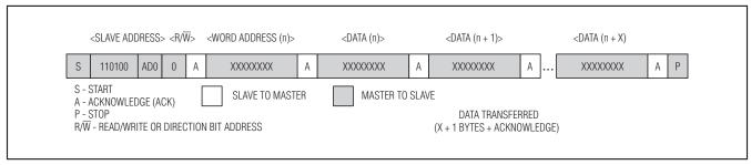
Figure 6. Data Write—Slave Receiver Mode
