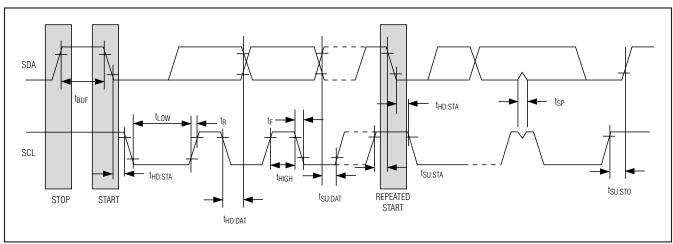
Figure 4. Data Transfer on I<sup>2</sup>C Serial Bus
