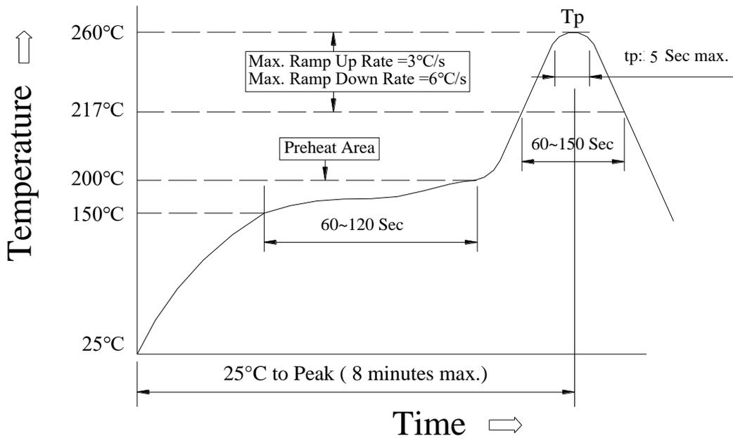
**Reflow Soldering Method:**
