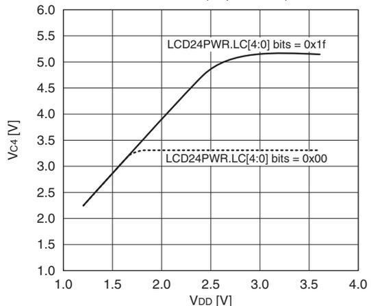
**LCD drive voltage-supply voltage characteristic (1/3 bias,  $V_{c1}$  reference voltage)**
