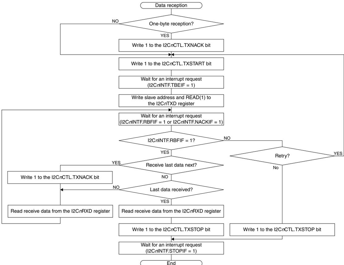
Figure 14.4.3.2 Master Mode Data Reception Flowchart
