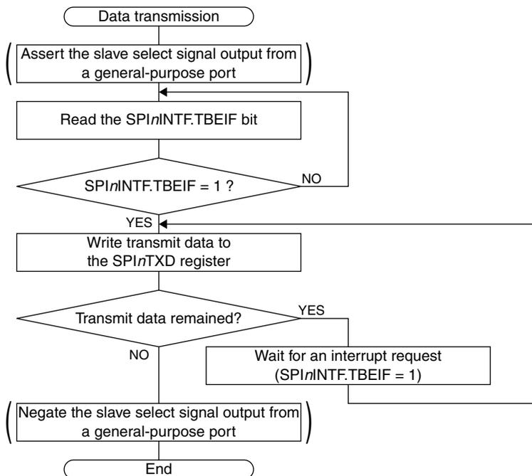
Figure 13.5.2.2 Data Transmission Flowchart in Master Mode
