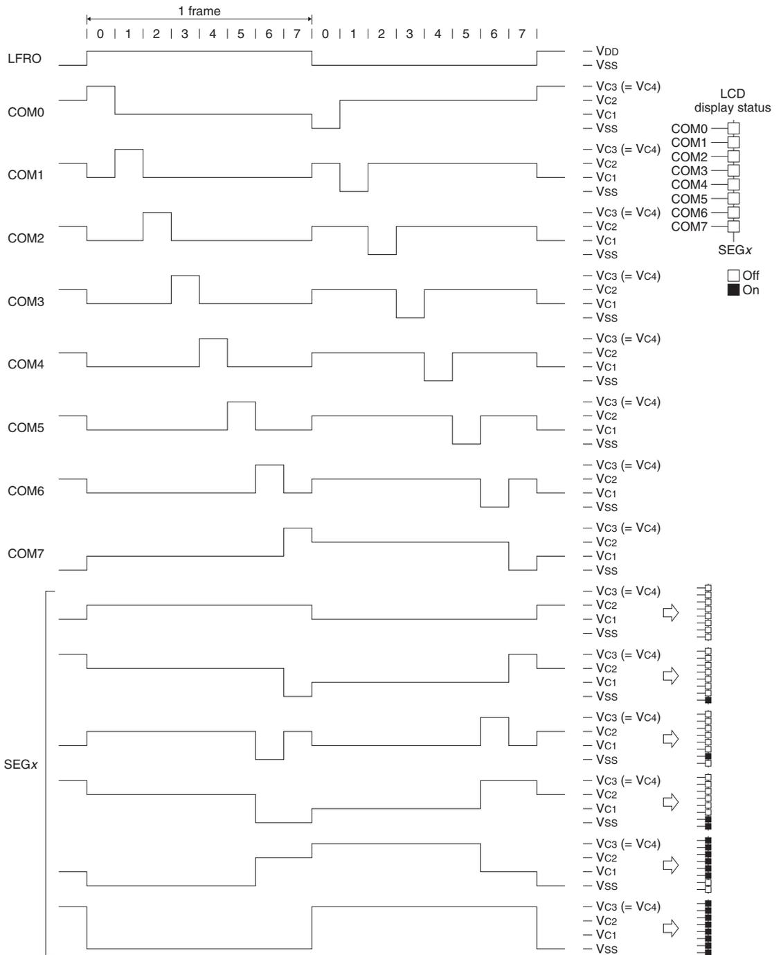
Figure 18.5.5.2 1/8 Duty Drive Waveform (1/3 bias)
