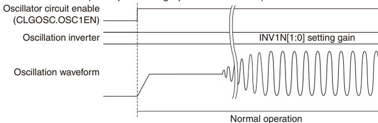
(2) CLGOSC1.OSC1BUP bit = 1 (startup boosting operation enabled)
