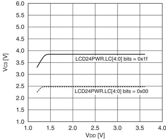
**LCD drive voltage-supply voltage characteristic (1/4 bias,  $V_{c1}$  reference voltage)**
