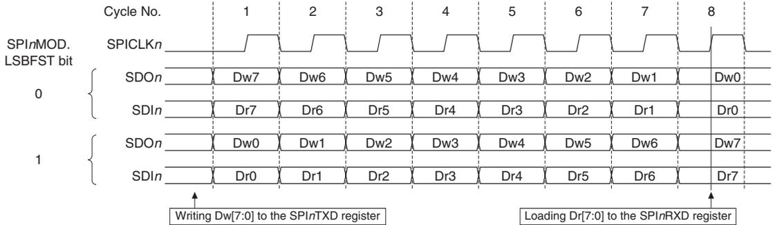
Figure 13.4.1 Data Format Selection Using the `SPInMOD.LSBFST` Bit
