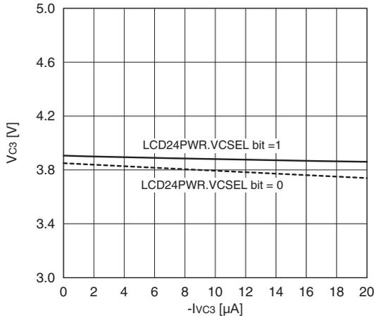
**LCD drive voltage-load characteristic (1/4 bias)**
