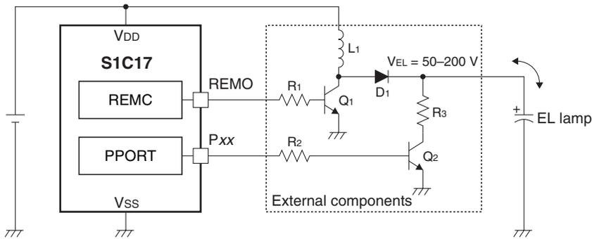
Figure 17.6.1 Example of EL Lamp Drive Circuit
