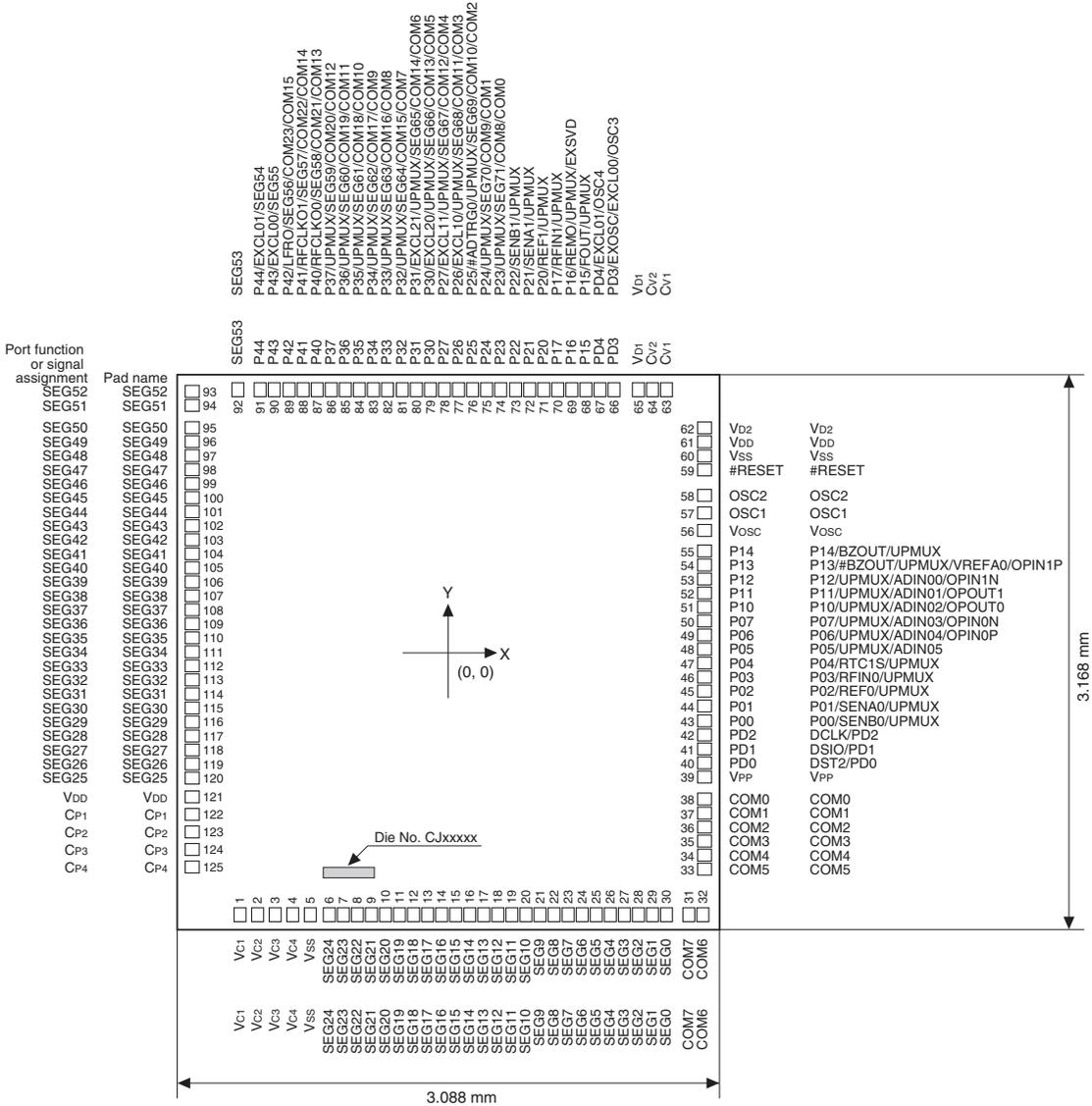
Pad opening No. 1–32, 63–92: X = 68 μm, Y = 80 μm
