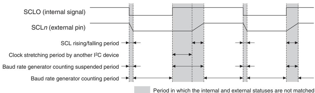
Figure 14.3.3.1 Baud Rate Generator Output Clock and SCL<sub>n</sub> Output Waveform
