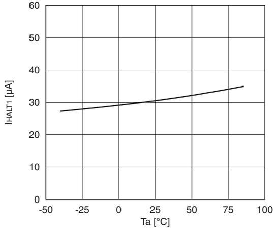
**Current consumption-temperature characteristic in HALT mode (OSC1 operation)**
