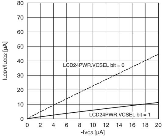
**LCD circuit current-load characteristic (1/4 bias)**
