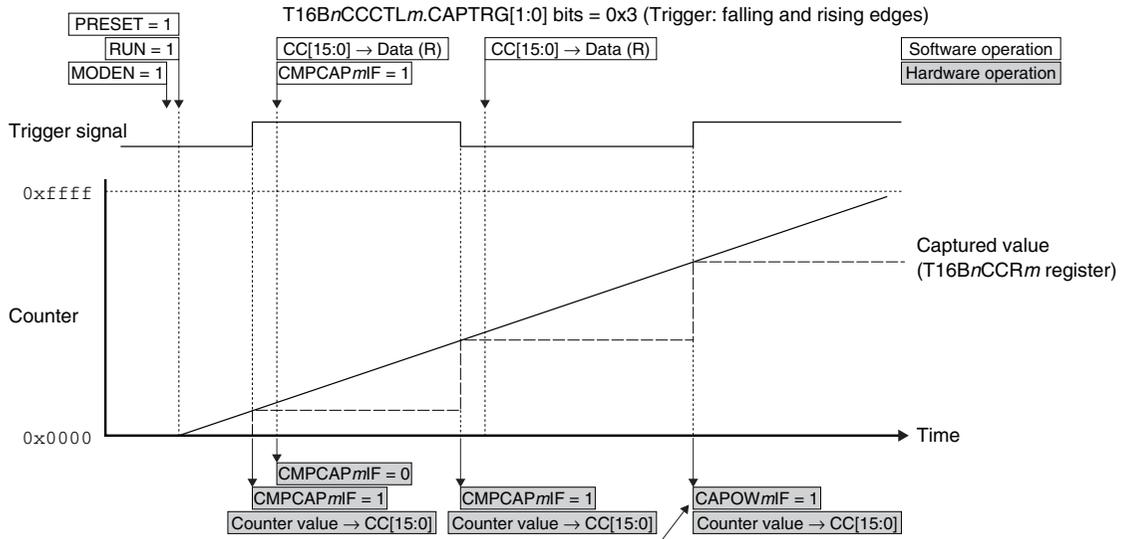
An overwrite error occurs as the T16BnINTF.CMPCAPmIF bit has not been cleared.
