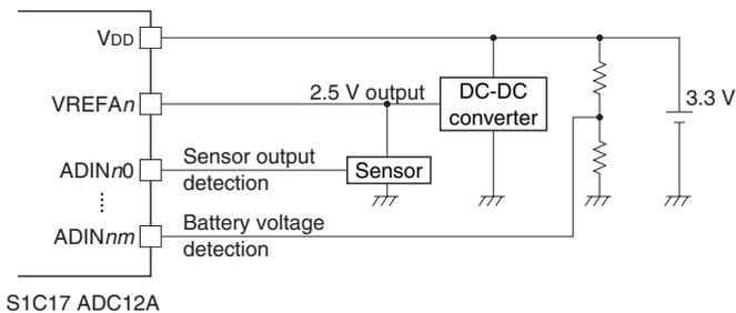
Figure 20.2.2.1 Connections between ADC12A and External Devices
