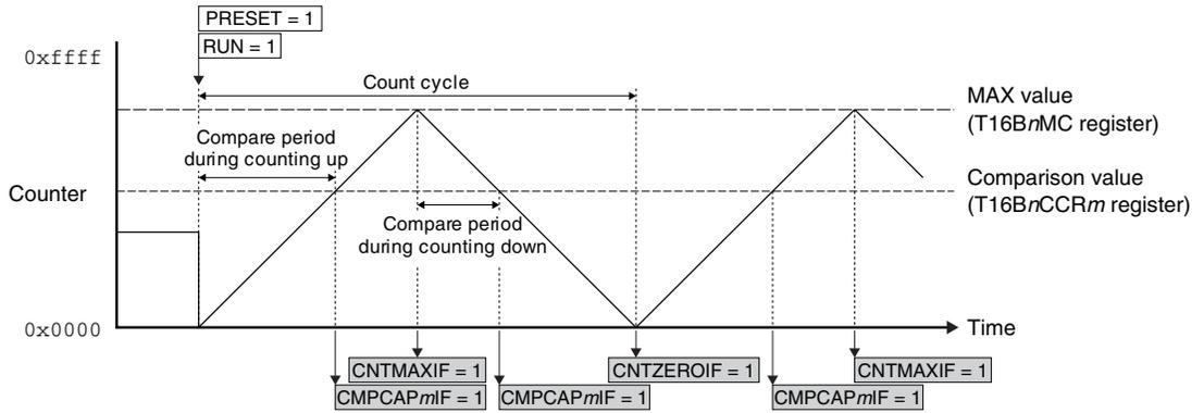
(Note that the T16BnINTF.CMPCAPmIF/CNTMAXIF/CNTZEROIF bit clearing operations via software are omitted from the figure.)
