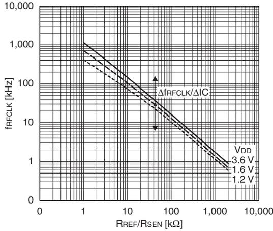
**RFC reference/sensor oscillation frequency-capacitance characteristic**
