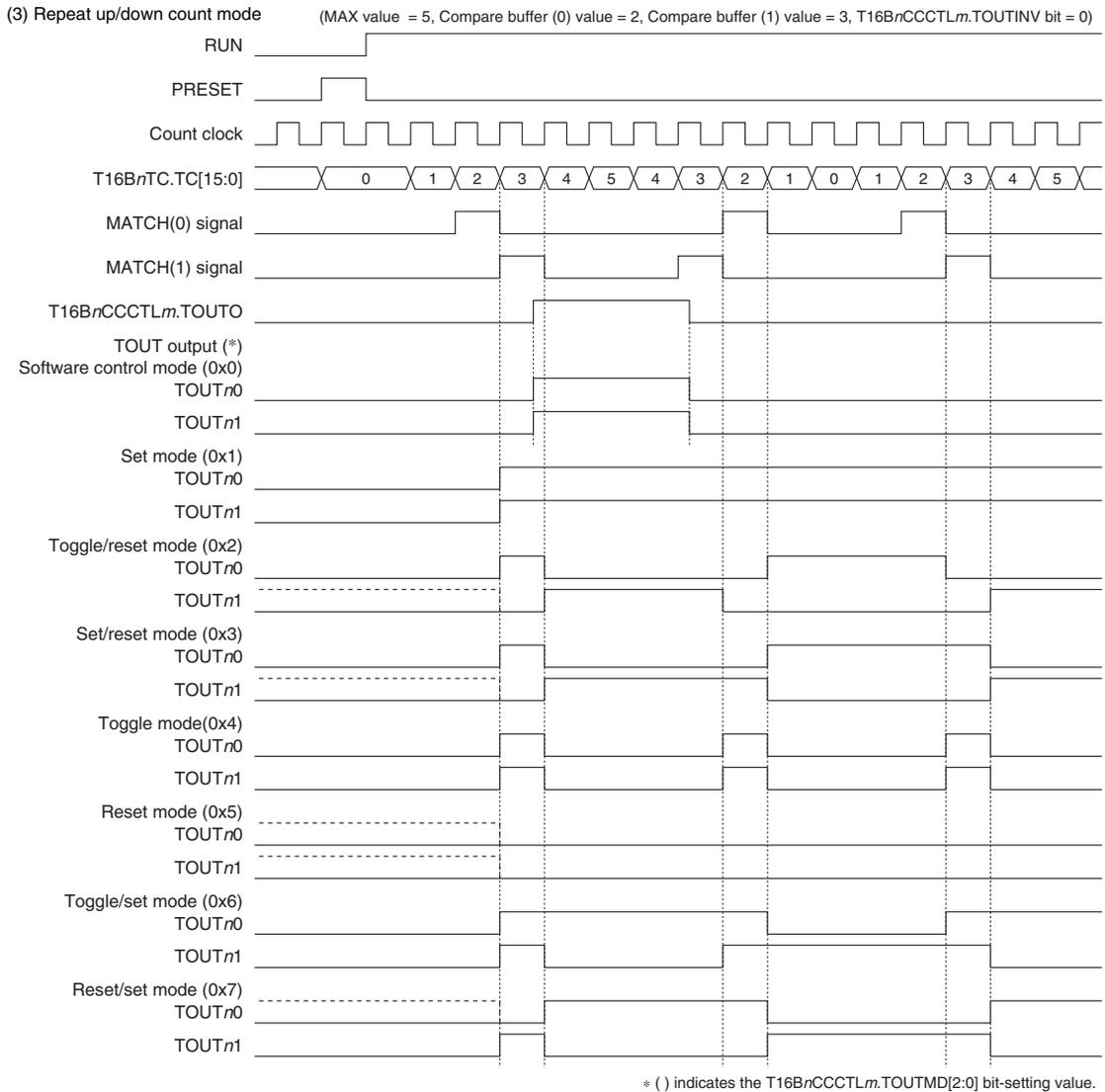
Figure 15.4.4.3 TOUT Output Waveform (T16BnCCCTL0.TOUTMT bit = 1, T16BnCCCTL1.TOUTMT bit = 0)
