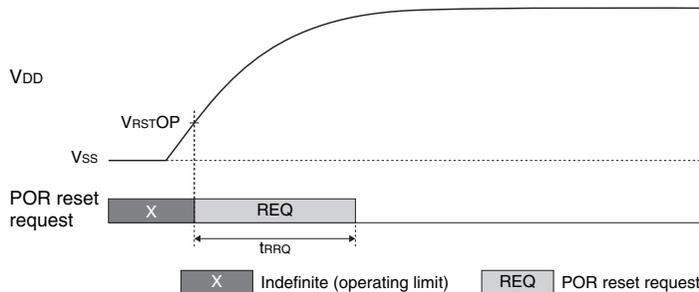
**Note:** When performing a power-on-reset again after the power is turned off, decrease the  $V_{DD}$  voltage to  $V_{RSTOP}$  or less.
