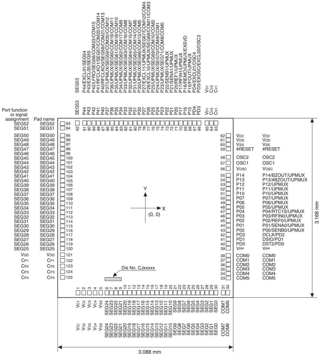
Figure 1.3.2.1 S1C17W22 Pad Configuration Diagram (Chip)
