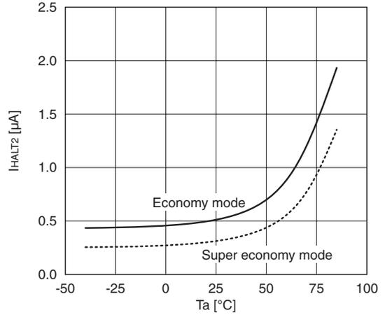
**Current consumption-temperature characteristic in RUN mode (IOSC operation)**
