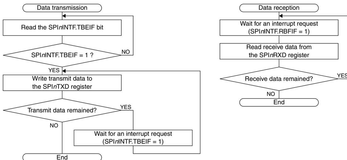
Figure 13.5.5.2 Data Transfer Flowcharts in Slave Mode
