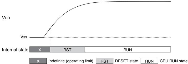
Figure 2.2.3.1 Example of Internal Reset by POR
