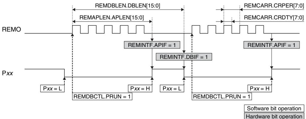
Figure 17.6.2 Example of Generated Drive Waveform
