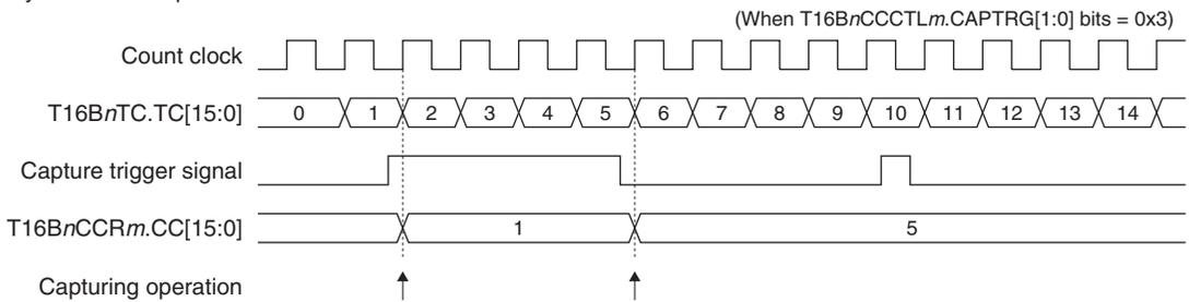
(2) Asynchronous capture mode
