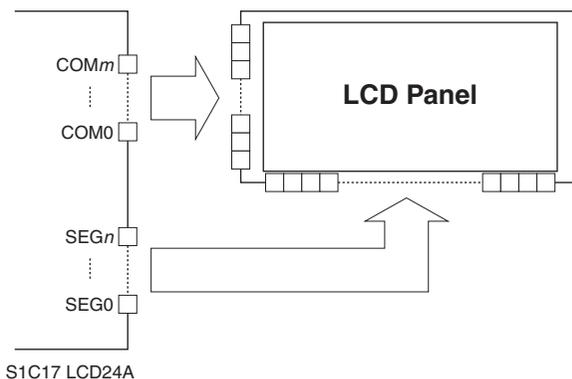
Figure 18.2.2.1 Connections between LCD24A and an LCD Panel
