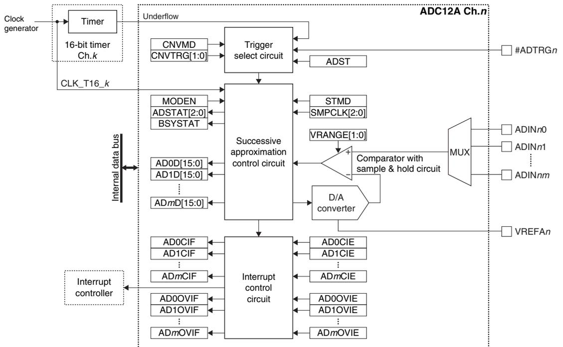
Figure 20.1.1 ADC12A Configuration
