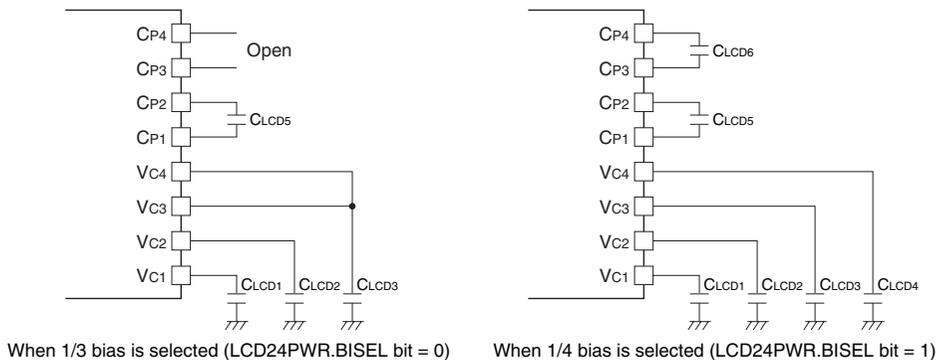
Figure 18.4.1.1 External Connection Example for Internal Generation Mode
