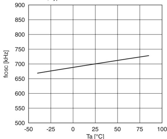
**OSC1 oscillator circuit characteristics**Unless otherwise specified: V<sub>DD</sub> = 1.2 to 3.6 V, V<sub>SS</sub> = 0 V, Ta = 25 °C
