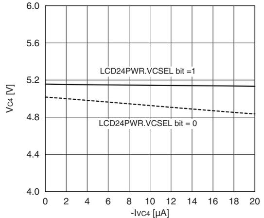
**LCD circuit current-load characteristic (1/3 bias)**
