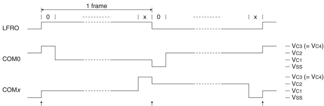
Figure 18.7.1 Frame Interrupt Timings (1/x duty, 1/3 bias)
