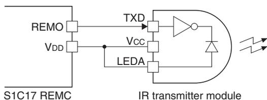
Figure 17.2.2.1 Connection Example Between REMC and External Infrared Module
