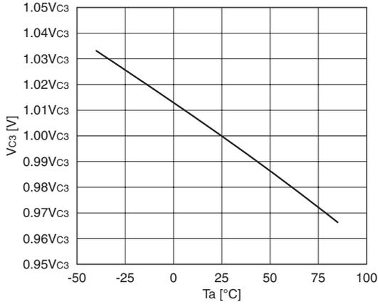
**LCD drive voltage-temperature characteristic (1/4 bias,  $V_{c1}/V_{c2}$  reference voltage)**
