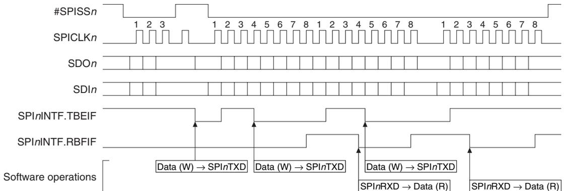
Figure 13.5.5.1 Example of Data Transfer Operations in Slave Mode ( $SPI_nMOD.CHLN[3:0]$  bits = 0x7)
