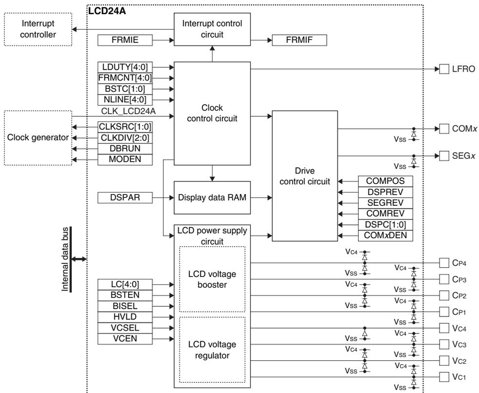
Figure 18.1.1 LCD24A Configuration
