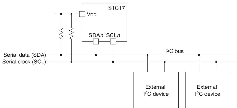
Figure 14.2.2.1 Connections between I<sup>2</sup>C and External I<sup>2</sup>C Devices
