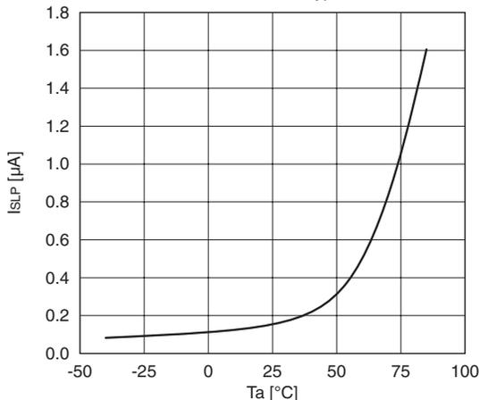
**Current consumption-temperature characteristic in HALT mode (IOSC operation)**
