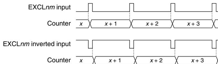
Figure 15.3.4.1 Count Timing (During Count Up Operation)
