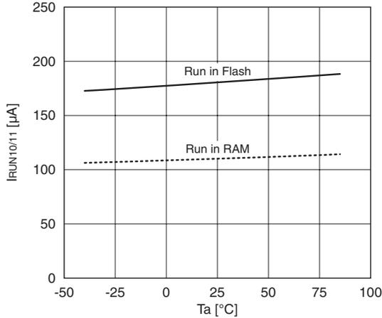
**Current consumption-temperature characteristic in RUN mode (OSC1 operation)**
