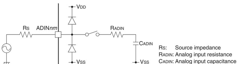
Figure 20.3.2.1 Equivalent Circuit of Analog Input Portion
