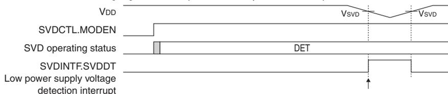
(2) When the SVDCTL.SVDMMD[1:0] bits  $\neq$  0x0 (intermittent operation mode)
