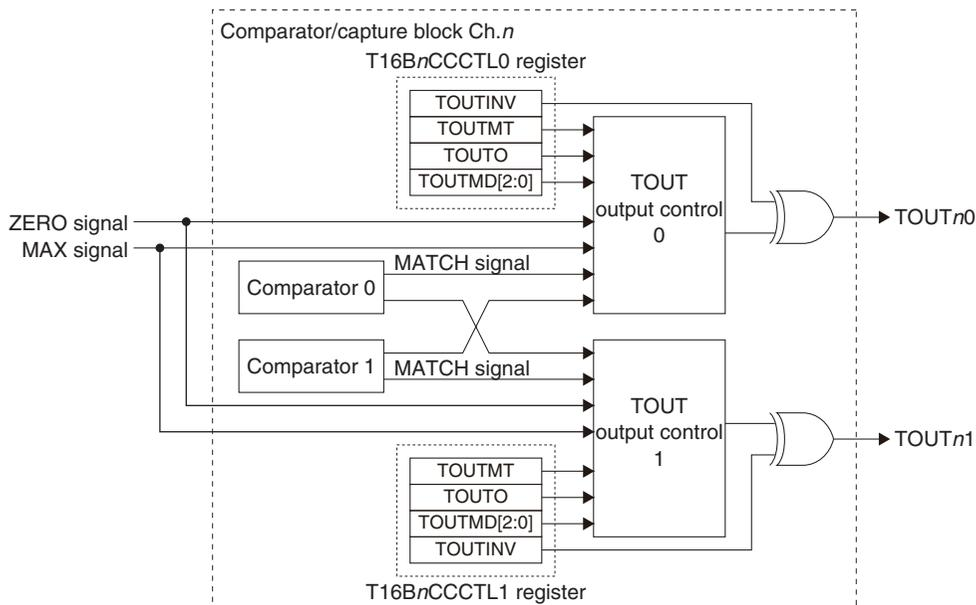
Figure 15.4.4.1 TOUT Output Circuits (Circuits 0 and 1)
