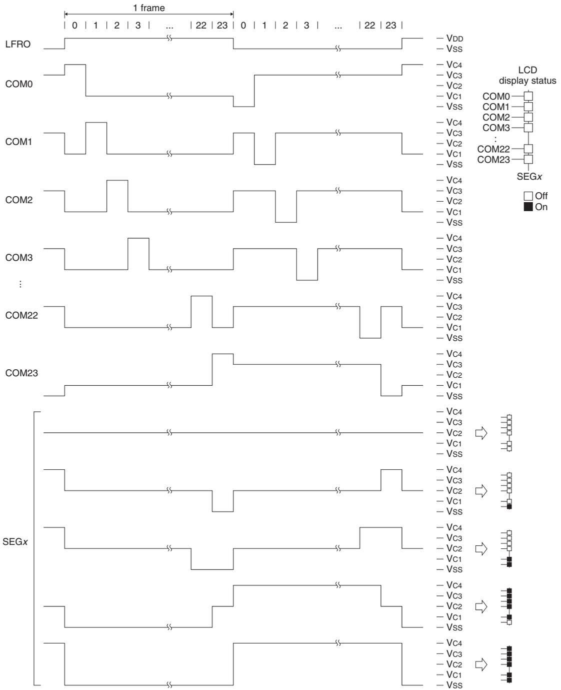
Figure 18.5.5.1 1/24 Duty Drive Waveform (1/4 bias)
