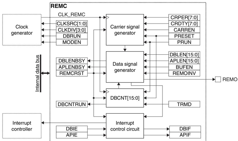
Figure 17.1.1 REMC Configuration
