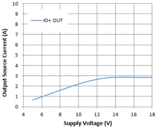
**Figure 12.** Output Source Current vs. Supply Voltage
