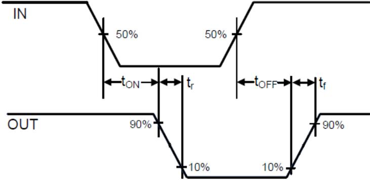
**Figure 1.** Switching Time Waveform Definitions
