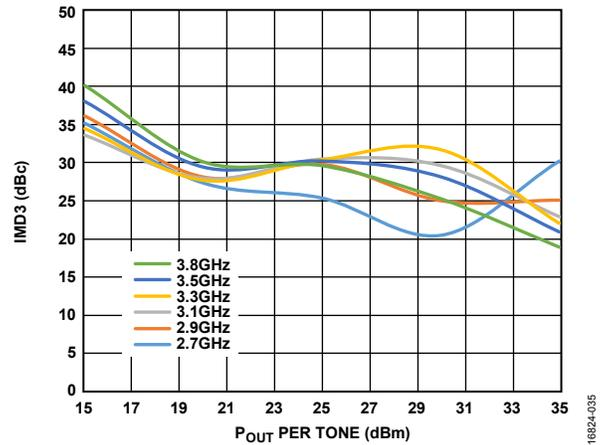
Figure 35. IMD3 vs.  $P_{OUT}$  per Tone,  $V_{DD} = 28 V$
