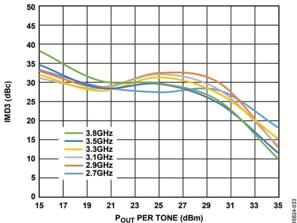
Figure 33. IMD3 vs.  $P_{OUT}$  per Tone,  $V_{DD} = 32 V$
