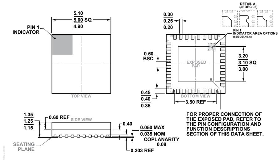
Figure 53. 32-Lead Lead Frame Chip Scale Package, Premolded Cavity [LFCSP\_CAV]
