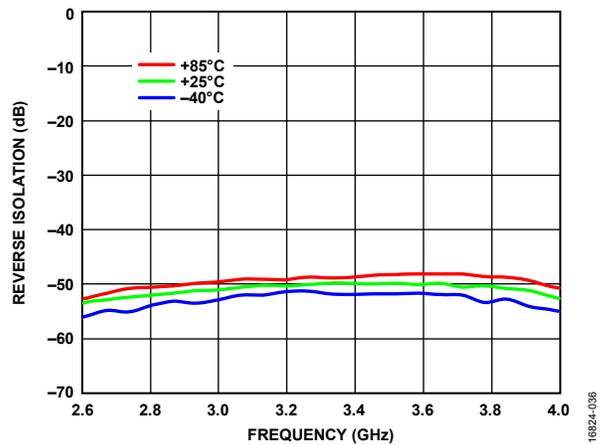
Figure 36. Reverse Isolation vs. Frequency at Various Temperatures
