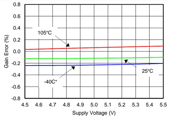
Figure 7. Gain Error vs Supply Voltage (Current Channel)
