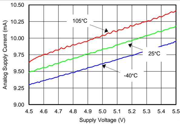
Figure 4. Analog Supply Current vs Supply Voltage
