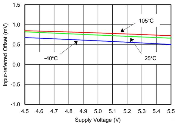
Figure 14. Input-Referred Offset  $V_{supply}$  Voltage (Voltage Channel)
