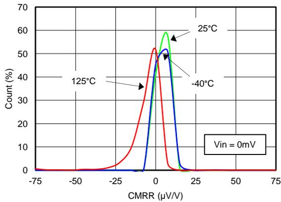
Figure 12. Common-Mode Rejection Ratio Distribution (Current Channel)
