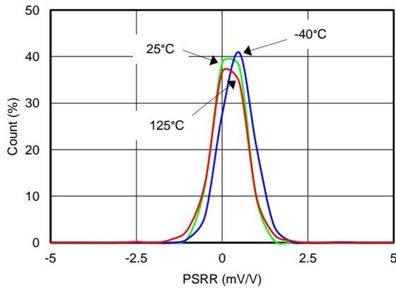
Figure 18. Power Supply Rejection Ratio Distribution (Voltage Channel)
