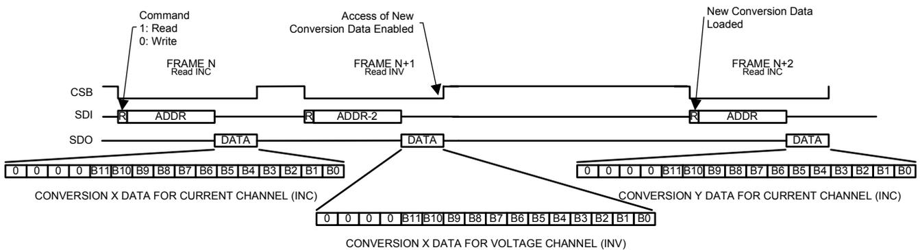
Figure 21. Timing Diagram With Word Read Frames
