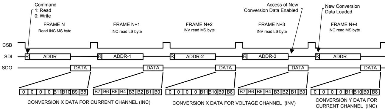
Figure 20. Timing Diagram With Byte Read Frames
