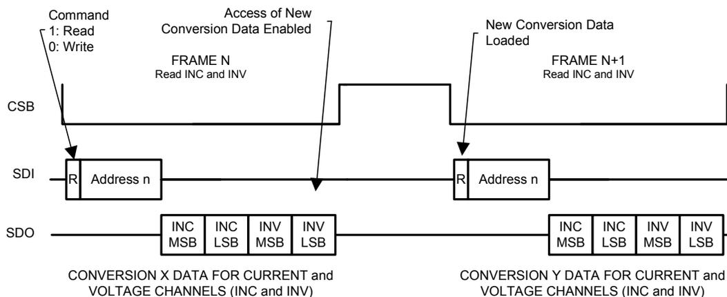
Figure 22. Timing Diagram With All Data Read Frames
