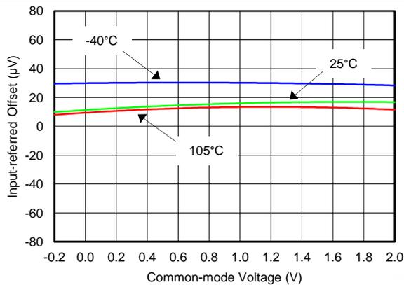
Figure 6. Input-Referred Offset vs Common-Mode Voltage (Current Channel)
