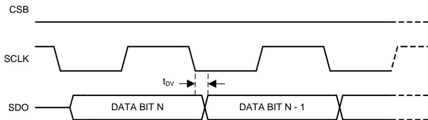
Figure 2. Serial Control Port Timing – Read
