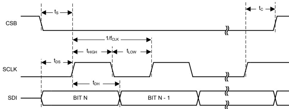
Figure 1. Serial Control Port Timing – Write
