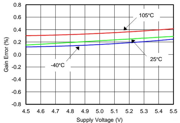
Figure 15. Gain Error vs Supply Voltage (Voltage Channel)
