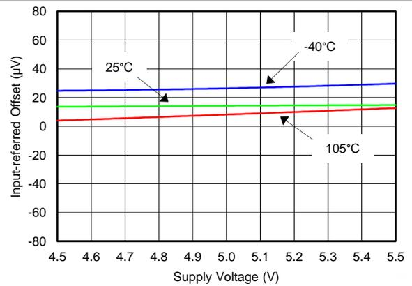
Figure 5. Input-Referred Offset vs Supply Voltage (Current Channel)
