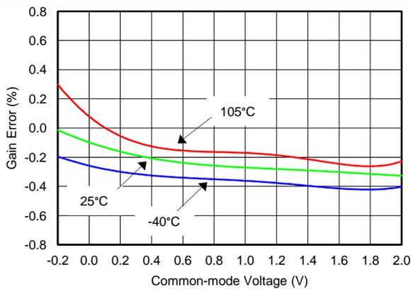
Figure 8. Gain Error vs Common-Mode Voltage (Current Channel)
