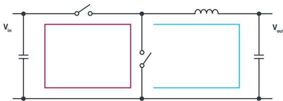
Figure 1. Paths with continuous current shown in blue and switched current shown in red.
