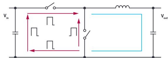
Figure 2. Different paths with different directions of current flow in a hot loop.
