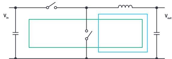
Figure 3. Real current loops leading to a so-called hot loop.
