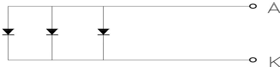
LED CIRCUIT DIAGAM(LED 1X3=3 dies)
