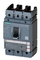
circuit breaker 3VA5 UL frame 250 breaking capacity class C 100kA @ 480V 3-pole, line protection TM230, FTAM, In=80A overload protection Ir=80A fixed short-circuit protection Ii=5...10 x In UL 489 SB (naval), 50 °C without connection
