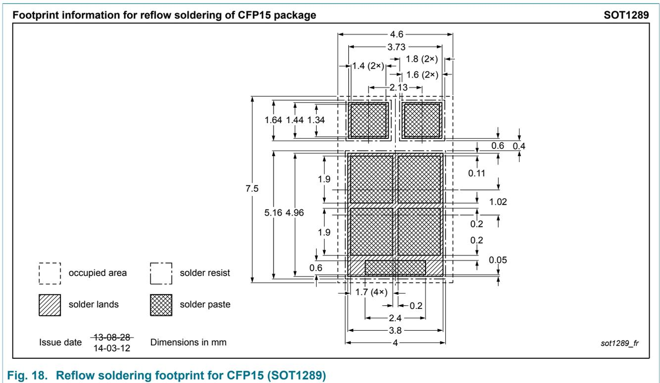
Fig. 18. Reflow soldering footprint for CFP15 (SOT1289)
