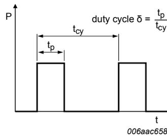
Fig. 16. Duty cycle definition
