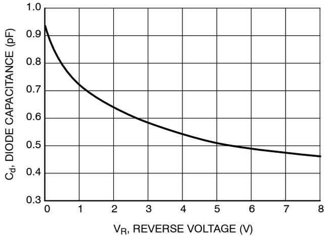
Figure 4. Diode Capacitance
