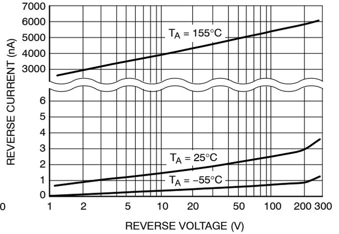
Figure 3. Reverse Leakage
