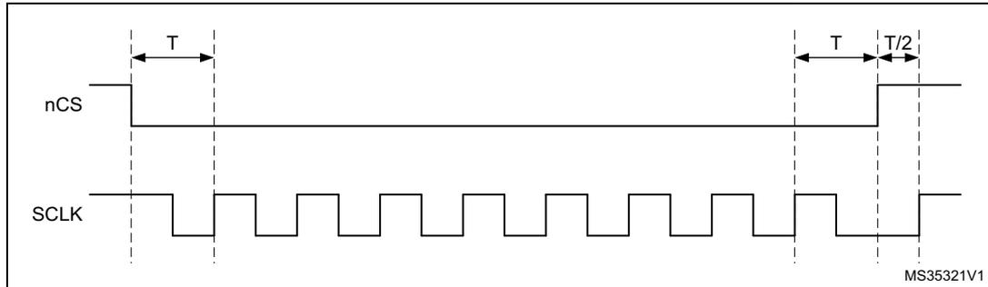
When the FIFO stays full in a read operation or if the FIFO stays empty in a write operation, the operation stalls and CLK stays low until firmware services the FIFO. If an abort occurs when an operation is stalled, nCS rises just after the abort is requested and then CLK rises one half of a CLK cycle later, as shown in *Figure 69*.
