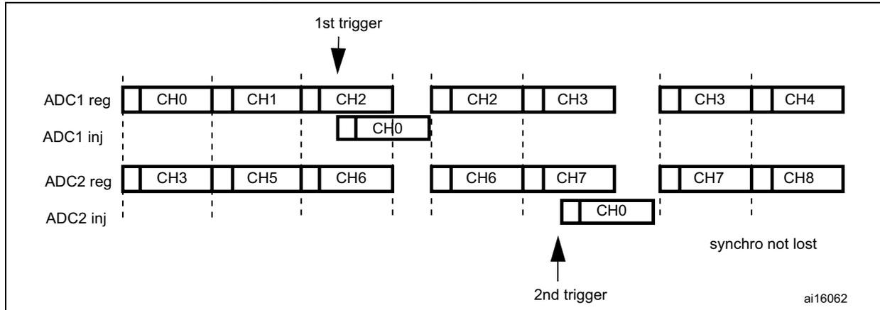
If a trigger occurs during an injected conversion that has interrupted a regular conversion, it is ignored. Figure 91 shows the behavior in this case (2nd trigger is ignored).
