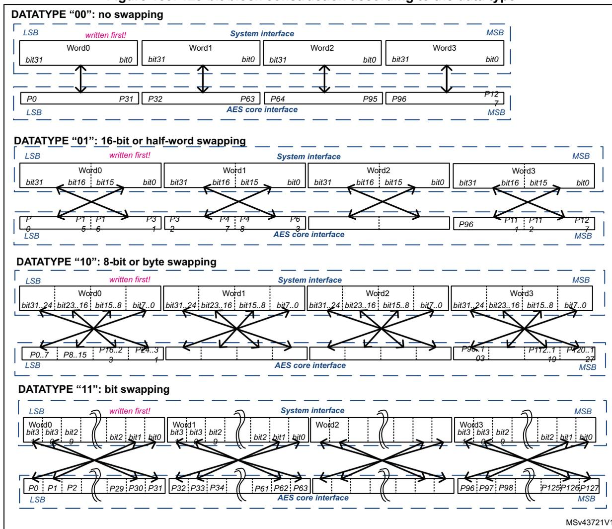
Note: The swapping operation concerns only the CRYP\_DOUT and CRYP\_DIN registers. The CRYP\_KxL/KxR and CRYP\_IVxL/IVxR registers are not sensitive to the swap mode selected. They have a fixed little-endian configuration (refer to Section 23.3.17 and Section 23.3.18).
