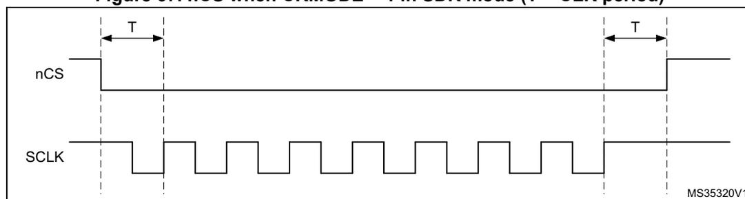
When CKMODE = 1 (“mode3”) and DDRM = 1 (DDR mode), nCS falls one CLK cycle before an operation first rising CLK edge, and nCS rises one CLK cycle after the operation final active rising CLK edge, as shown in *Figure 68*. Because DDR operations must finish with a falling edge, CLK is low when nCS rises, and CLK rises back up one half of a CLK cycle afterwards.
