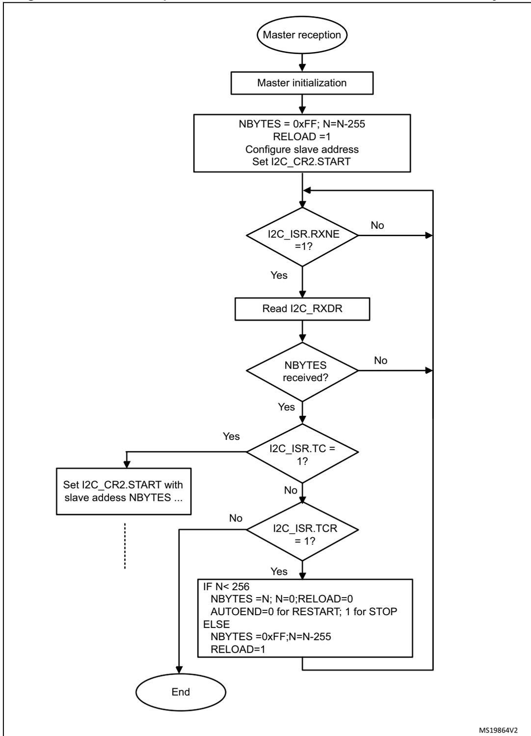
Figure 371. Transfer bus diagrams for I2C master receiver
