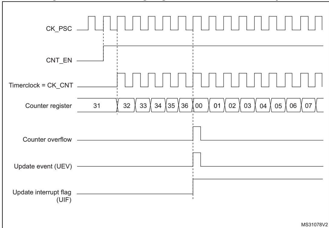
**Figure 199. Counter timing diagram, internal clock divided by 2**
