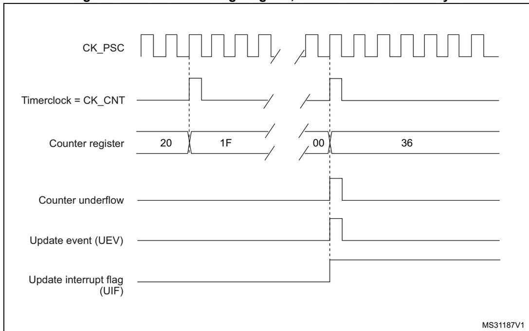
**Figure 208. Counter timing diagram, update event when repetition counter is not used**
