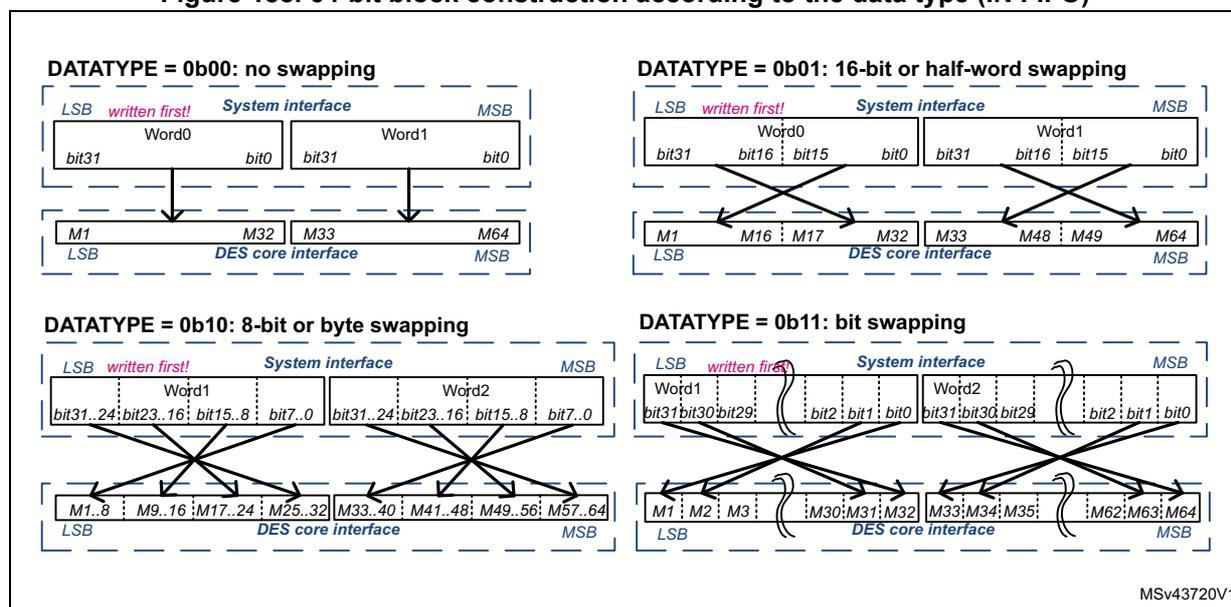
Note: The CRYP Key registers (CRYP\_Kx(L/R)) and initialization registers (CRYP\_IVx(L/R)) are not sensitive to the swap mode selected. They have a fixed little-endian configuration (refer to Section 23.3.17 and Section 23.3.18, respectively).
