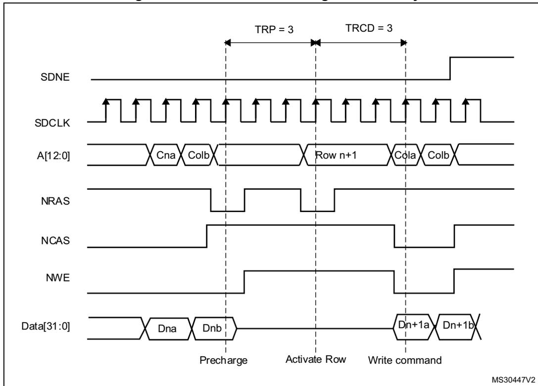
If the next access is sequential and the current access crosses a bank boundary, the SDRAM controller activates the first row in the next bank and initiates a new read/write command. Two cases are possible:
