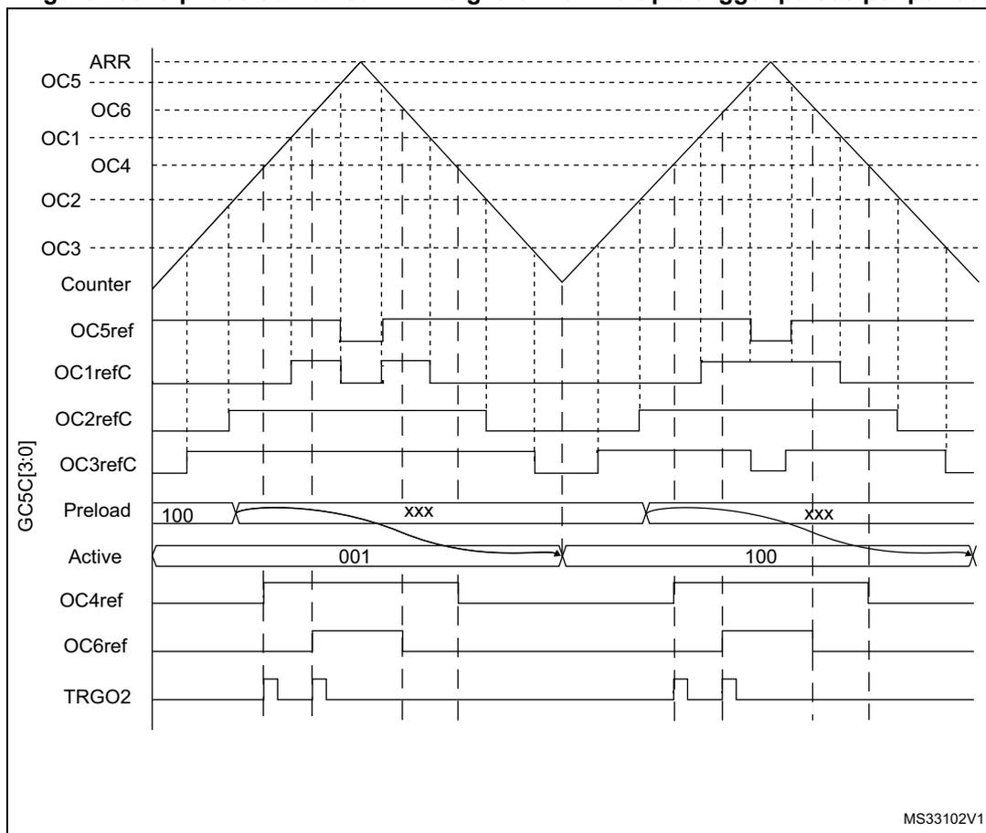
The TRGO2 waveform shows how the ADC can be synchronized on given 3-phase PWM signals. Refer to [Section 25.3.26: ADC synchronization](#) for more details.
