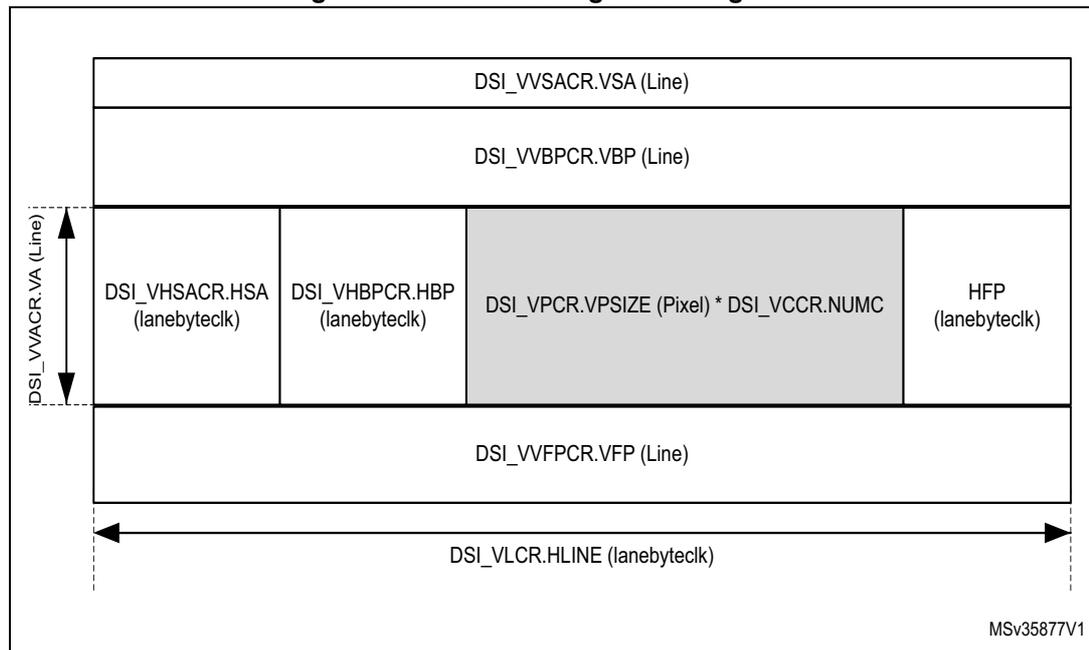
Note: The number of pixels of payload is restricted to a multiple of a value provided in [Table 133](#).
