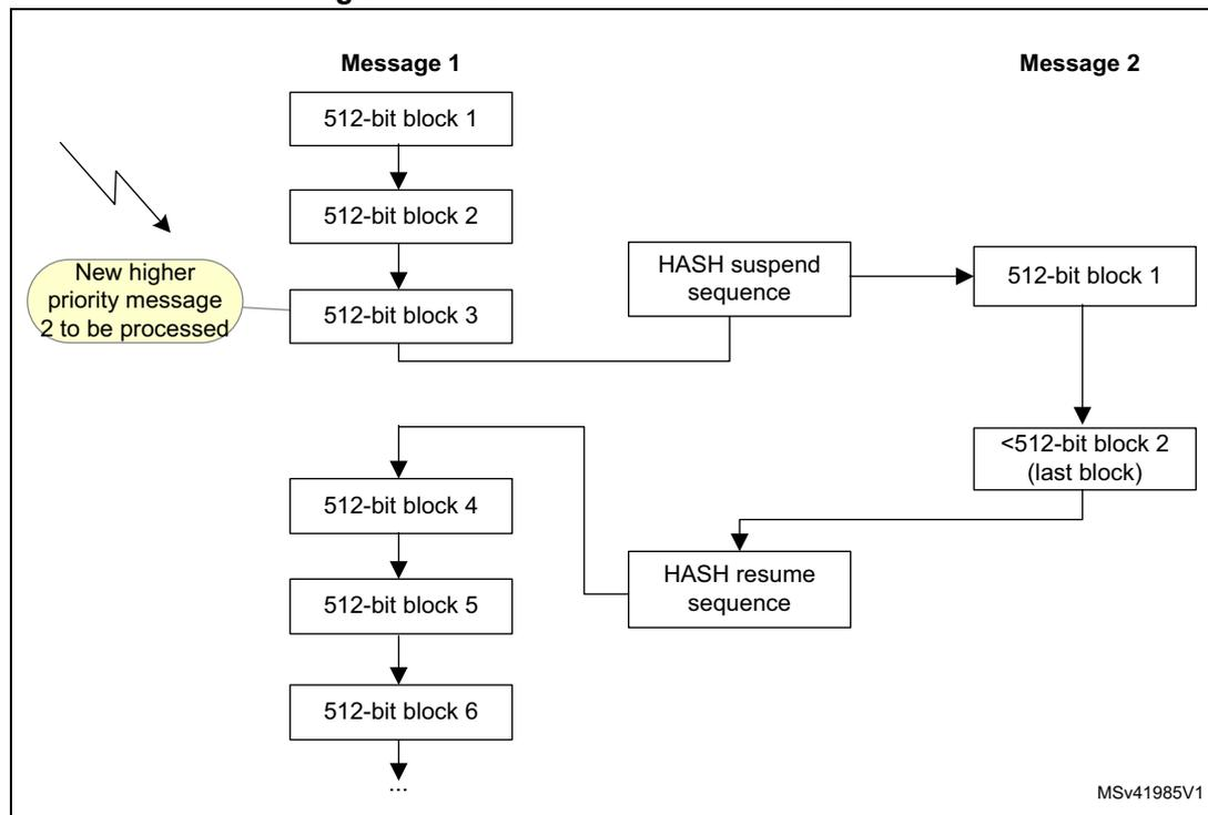
To do so, the context of the interrupted task must be saved from the HASH registers to memory, and then be restored from memory to the HASH registers.
