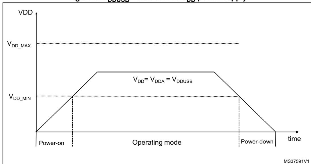
Figure 7.  $V_{DDUSB}$  connected to external independent power supply
