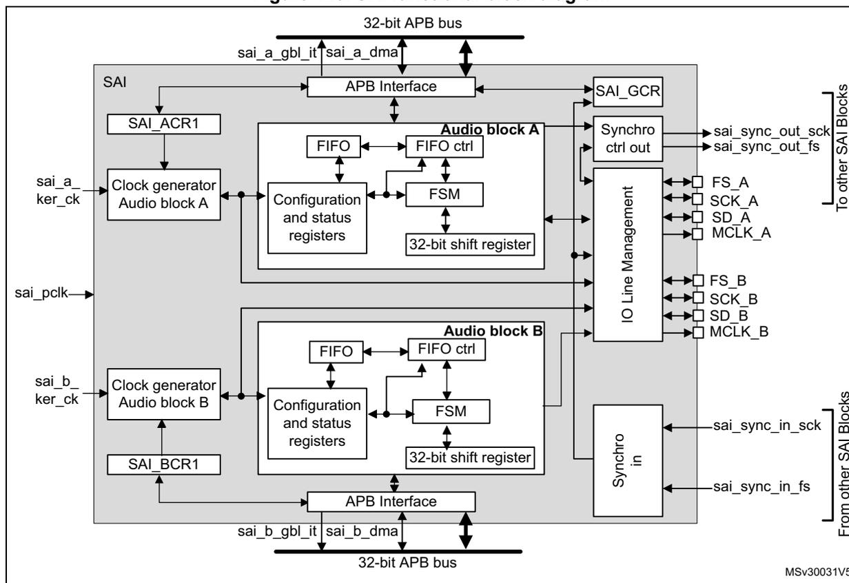
The SAI is mainly composed of two audio sub-blocks with their own clock generator. Each audio block integrates a 32-bit shift register controlled by their own functional state machine. Data are stored or read from the dedicated FIFO. FIFO may be accessed by the CPU, or by DMA in order to leave the CPU free during the communication. Each audio block is independent. They can be synchronous with each other.
