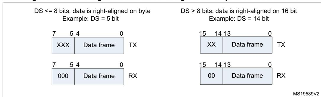
**Note:** The minimum data length is 4 bits. If a data length of less than 4 bits is selected, it is forced to an 8-bit data frame size.
