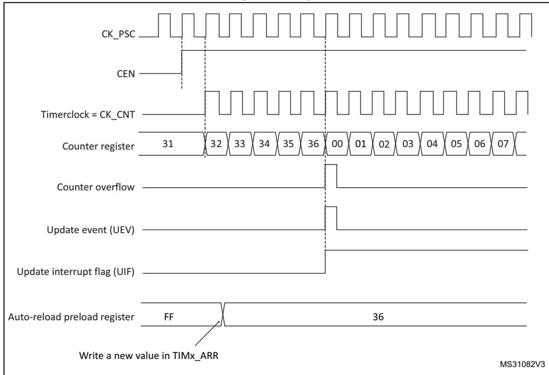
**Figure 203. Counter timing diagram, update event when ARPE=1 (TIMx\_ARR preloaded)**
