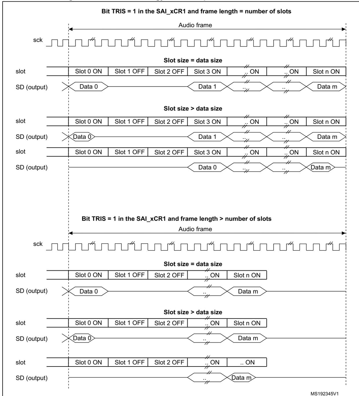
When the selected audio protocol uses the FS signal as a start of frame and a channel side identification (bit FSDEF = 1 in the SAI\_xFRCR register), the tristate mode is managed according to [Figure 456](#) (where bit TRIS in the SAI\_xCR1 register = 1, and FSDEF=1, and half frame length is higher than number of slots/2, and NBSLOT=6).
