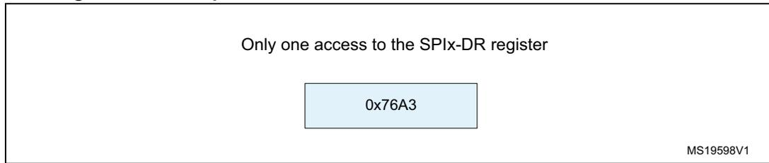
In transmission mode, when a TXE event occurs, the application has to write the data to be transmitted (in this case 0x76A3). The 0x000 field is transmitted first (extension on 32-bit). The TXE flag is set again as soon as the effective data (0x76A3) is sent on SD.
