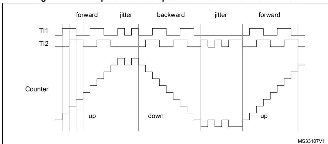
Figure 246 gives an example of counter behavior when TI1FP1 polarity is inverted (same configuration as above except CC1P='1').
