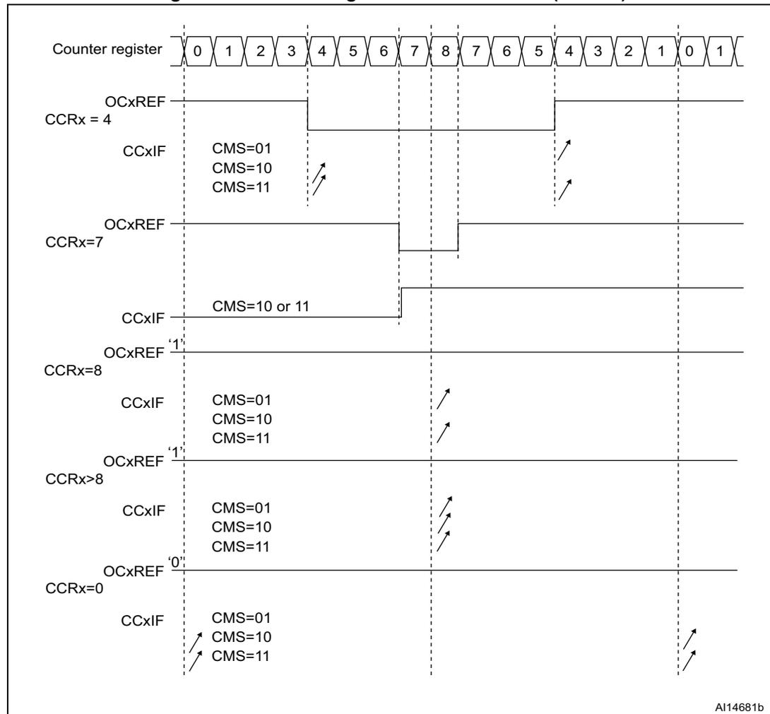
Hints on using center-aligned mode
