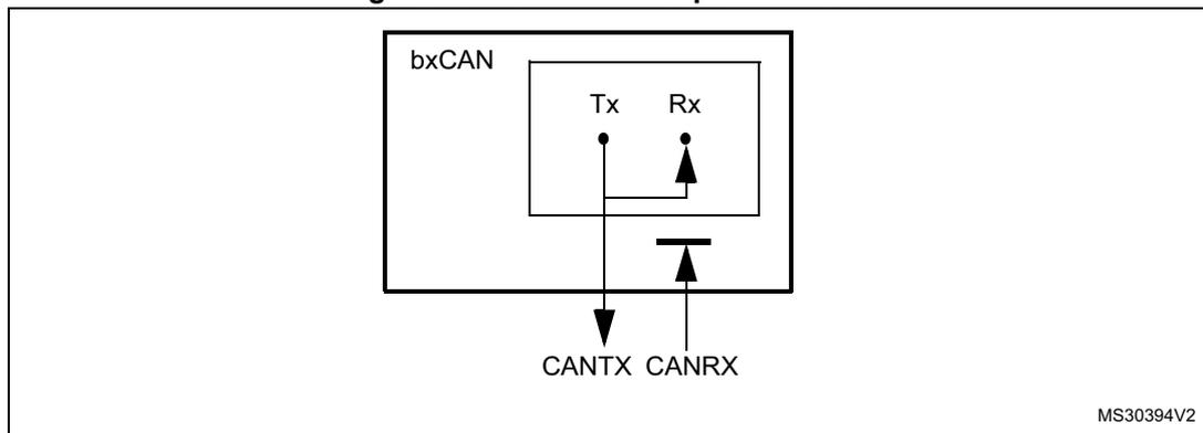
This mode is provided for self-test functions. To be independent of external events, the CAN Core ignores acknowledge errors (no dominant bit sampled in the acknowledge slot of a data / remote frame) in Loop Back Mode. In this mode, the bxCAN performs an internal feedback from its Tx output to its Rx input. The actual value of the CANRX input pin is disregarded by the bxCAN. The transmitted messages can be monitored on the CANTX pin.
