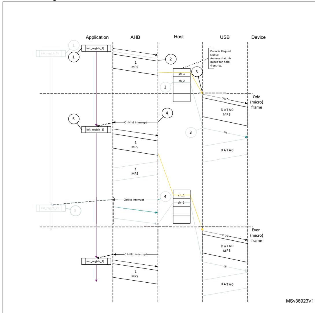
• **Isochronous IN transactions in DMA mode**
