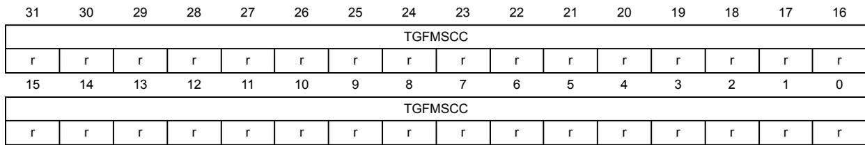
Bits 31:0 **TGMSCC**: Transmitted good frames more single collision counter
