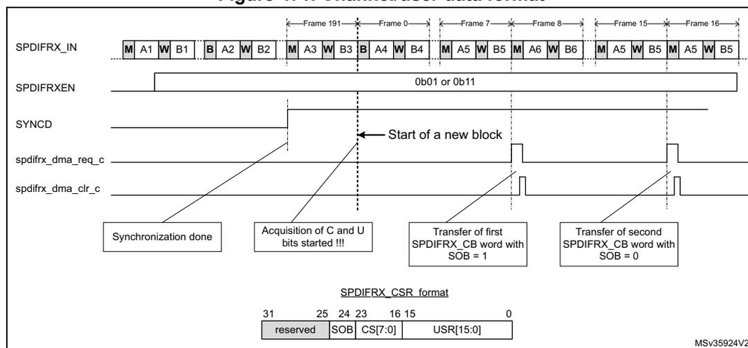
Note: Once the first start of block is detected (B preamble), the SPDIFRX is checking the preamble type every 8 frames.
