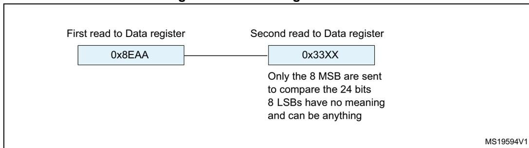
**Figure 427. I<sup>2</sup>S Philips standard (16-bit extended to 32-bit packet frame)**
