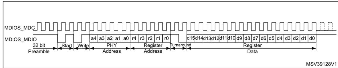
**Figure 477. MDIO protocol read frame waveform**
