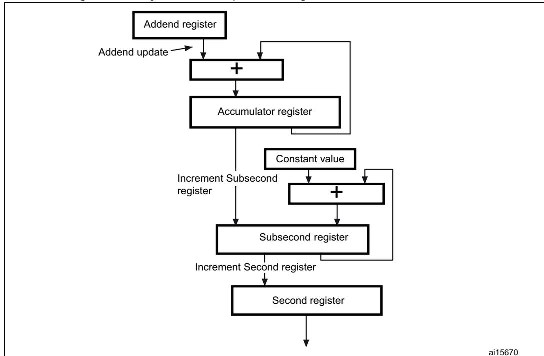
The system time update logic requires a 50 MHz clock frequency to achieve 20 ns accuracy. The frequency division is the ratio of the reference clock frequency to the required clock frequency. Hence, if the reference clock (HCLK) is, let us say, 66 MHz, the ratio is calculated as 66 MHz/50 MHz = 1.32. Hence, the default addend value to be set in the register is  $2^{32}/1.32$ , which is equal to 0xC1F0 7C1F.
