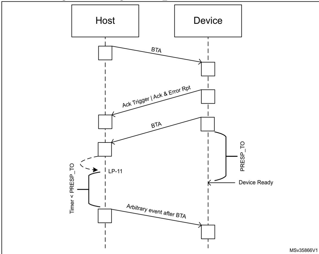
Figure 136. Timing of PRESP\_TO after a read request (HS or LP)
