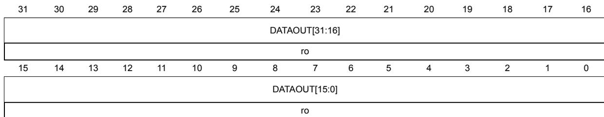
Bits 31: 0 **DATAOUT[31:0]**: Data output FIFO
