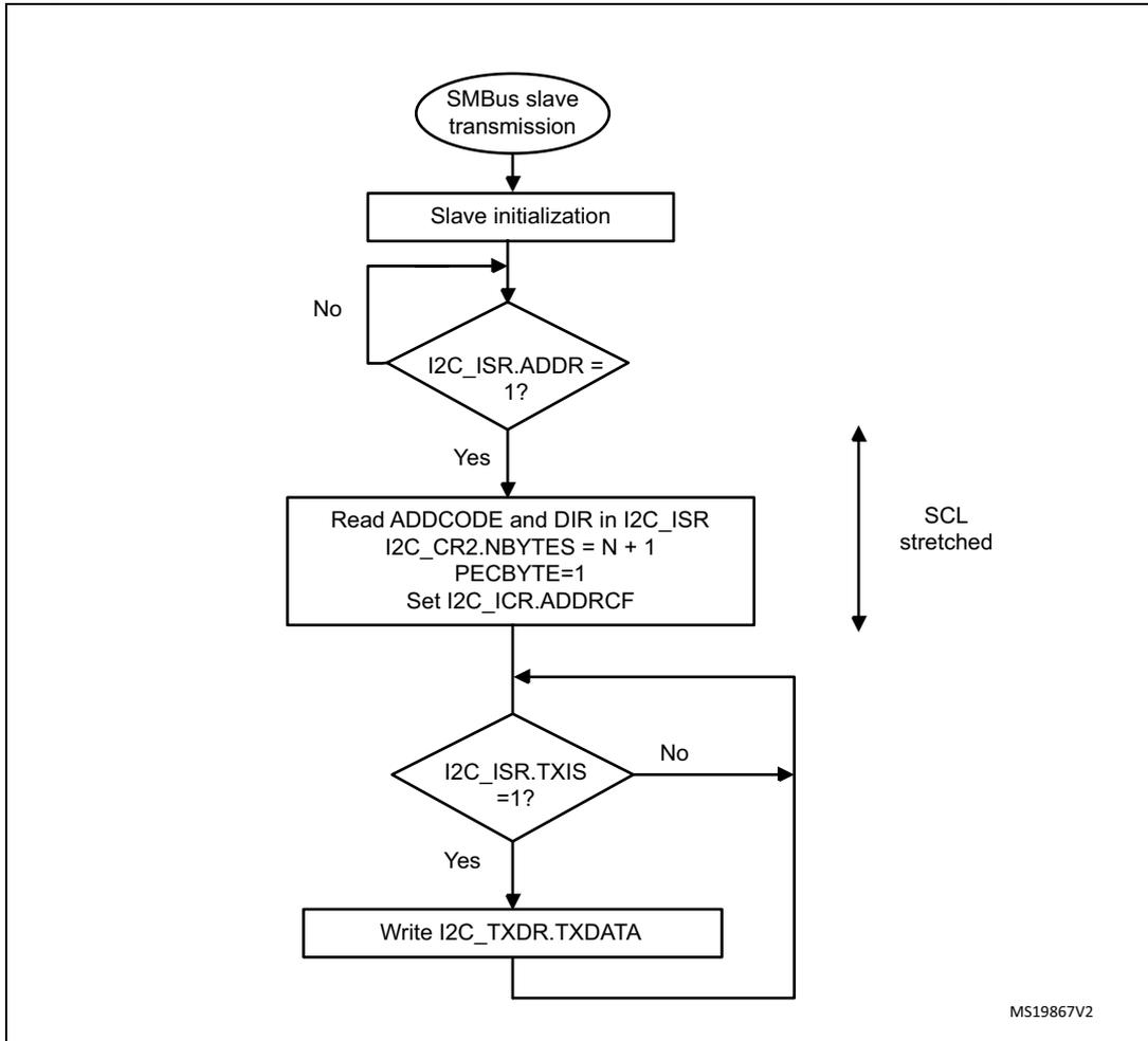
**Figure 374. Transfer bus diagrams for SMBus slave transmitter (SBC=1)**
