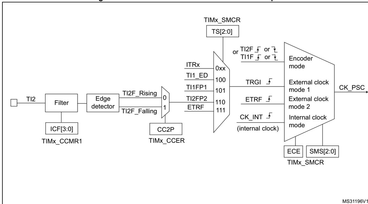
For example, to configure the upcounter to count in response to a rising edge on the TI2 input, use the following procedure:
