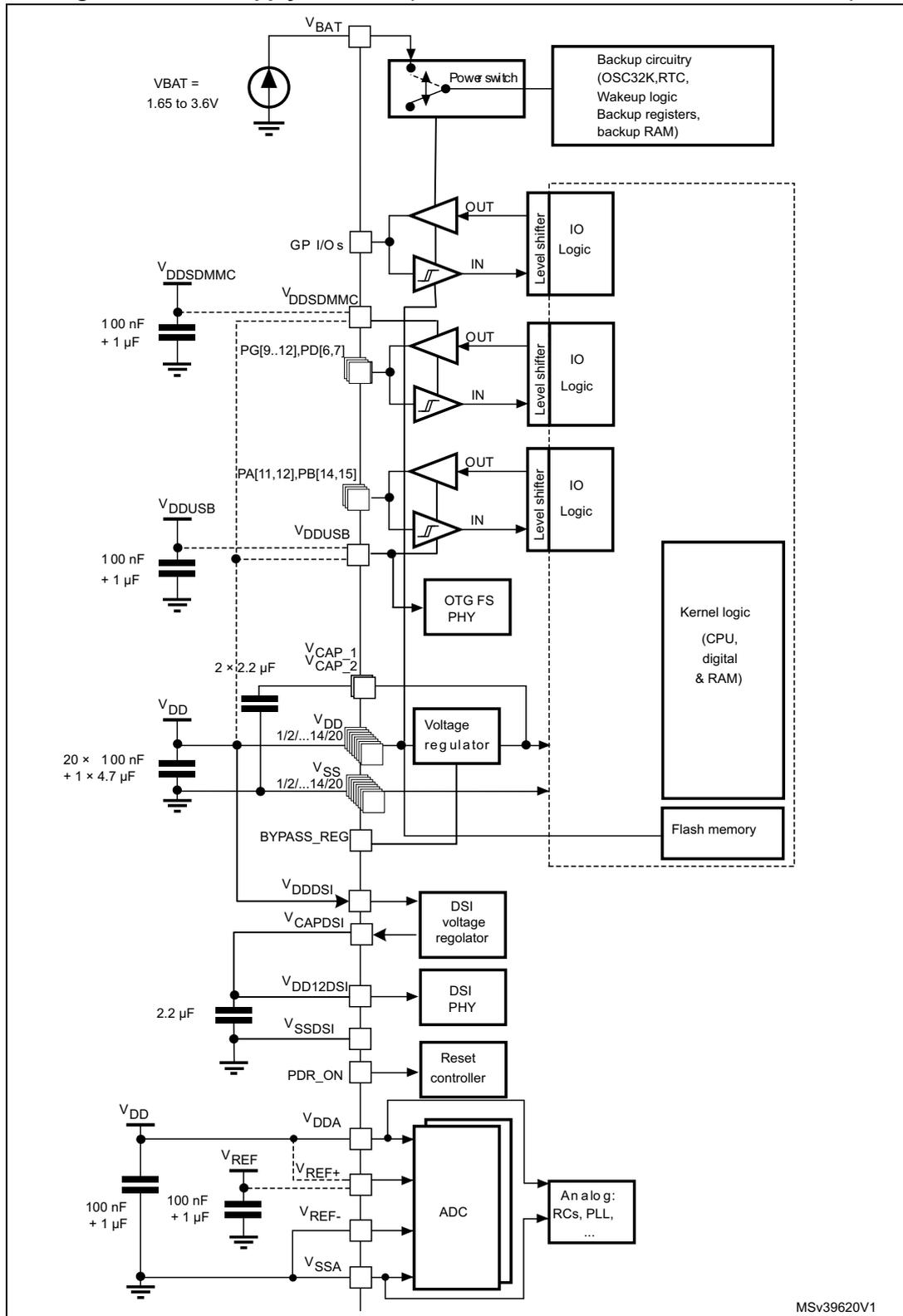
1.  $V_{DDA}$  and  $V_{SSA}$  must be connected to  $V_{DD}$  and  $V_{SS}$ , respectively.
