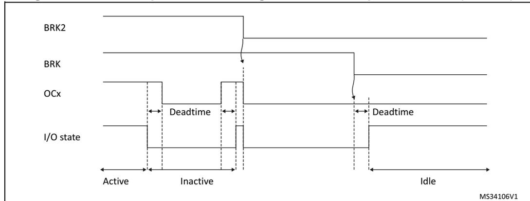
Figure 240. PWM output state following BRK assertion (OSSI=0)
