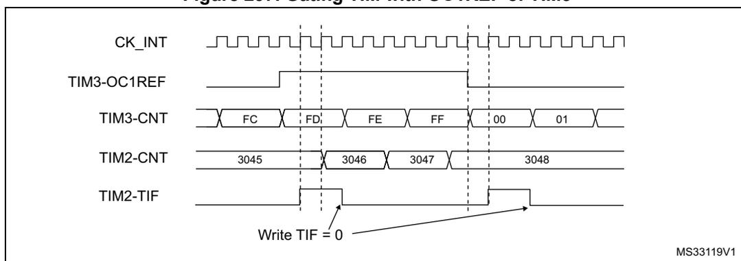
In the example in [Figure 297](#), the TIM counter and prescaler are not initialized before being started. So they start counting from their current value. It is possible to start from a given
