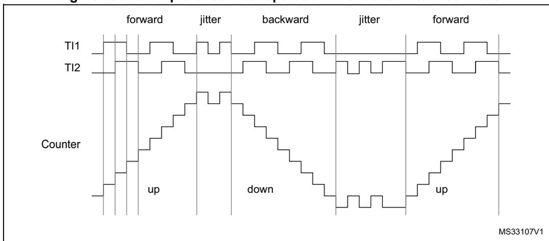
Figure 291 gives an example of counter behavior when TI1FP1 polarity is inverted (same configuration as above except CC1P=1).
