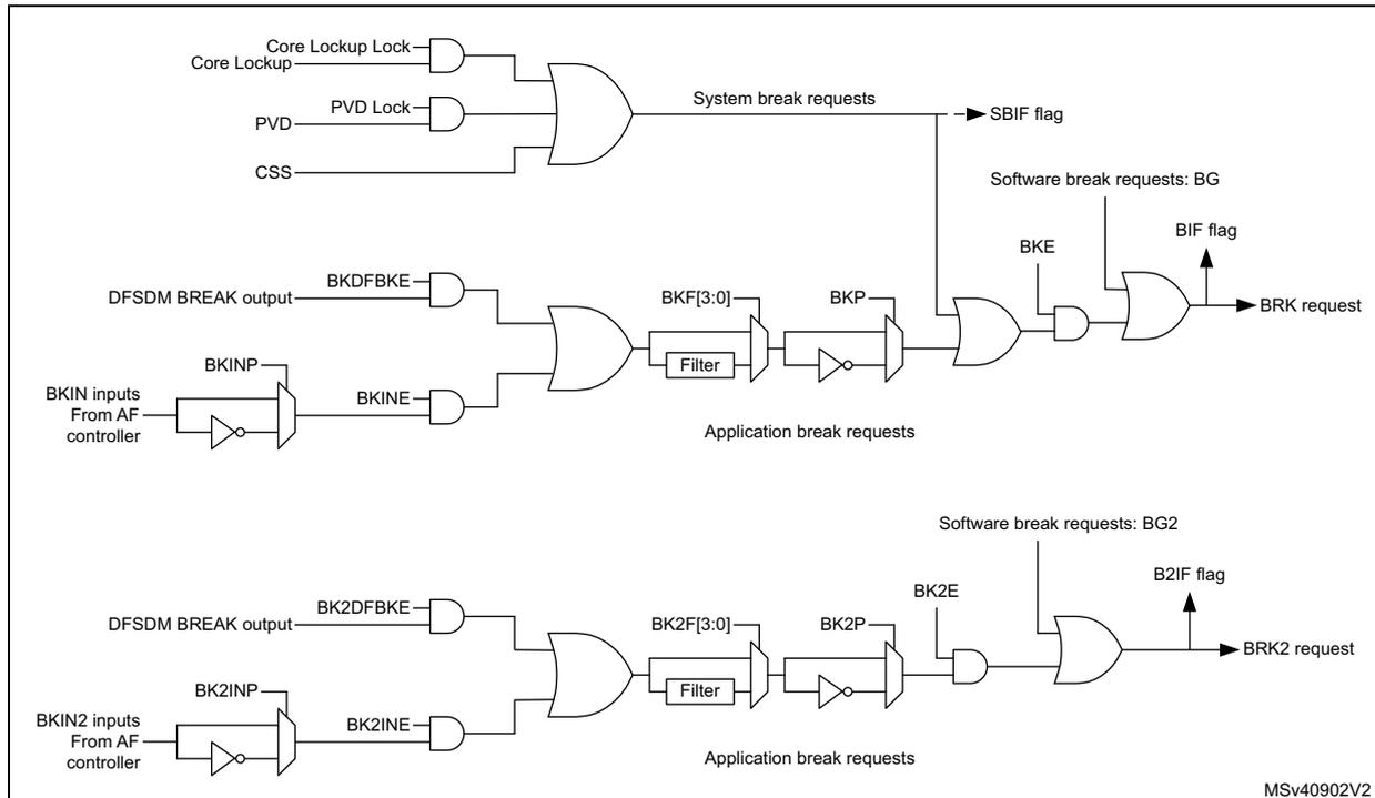
**Note:** An asynchronous (clockless) operation is only guaranteed when the programmable filter is disabled. If it is enabled, a fail safe clock mode (for example by using the internal PLL and/or the CSS) must be used to guarantee that break events are handled.
