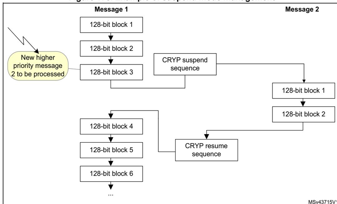
A detailed description of suspend/resume operations can be found in each AES mode section.
