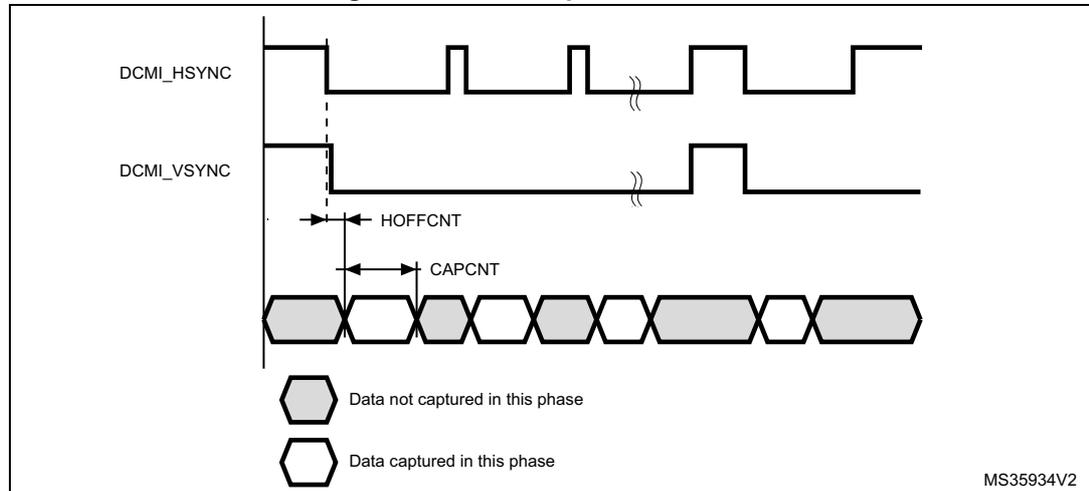
1. Here, the active state of DCMI\_HSYNC and DCMI\_VSYNC is 1.
