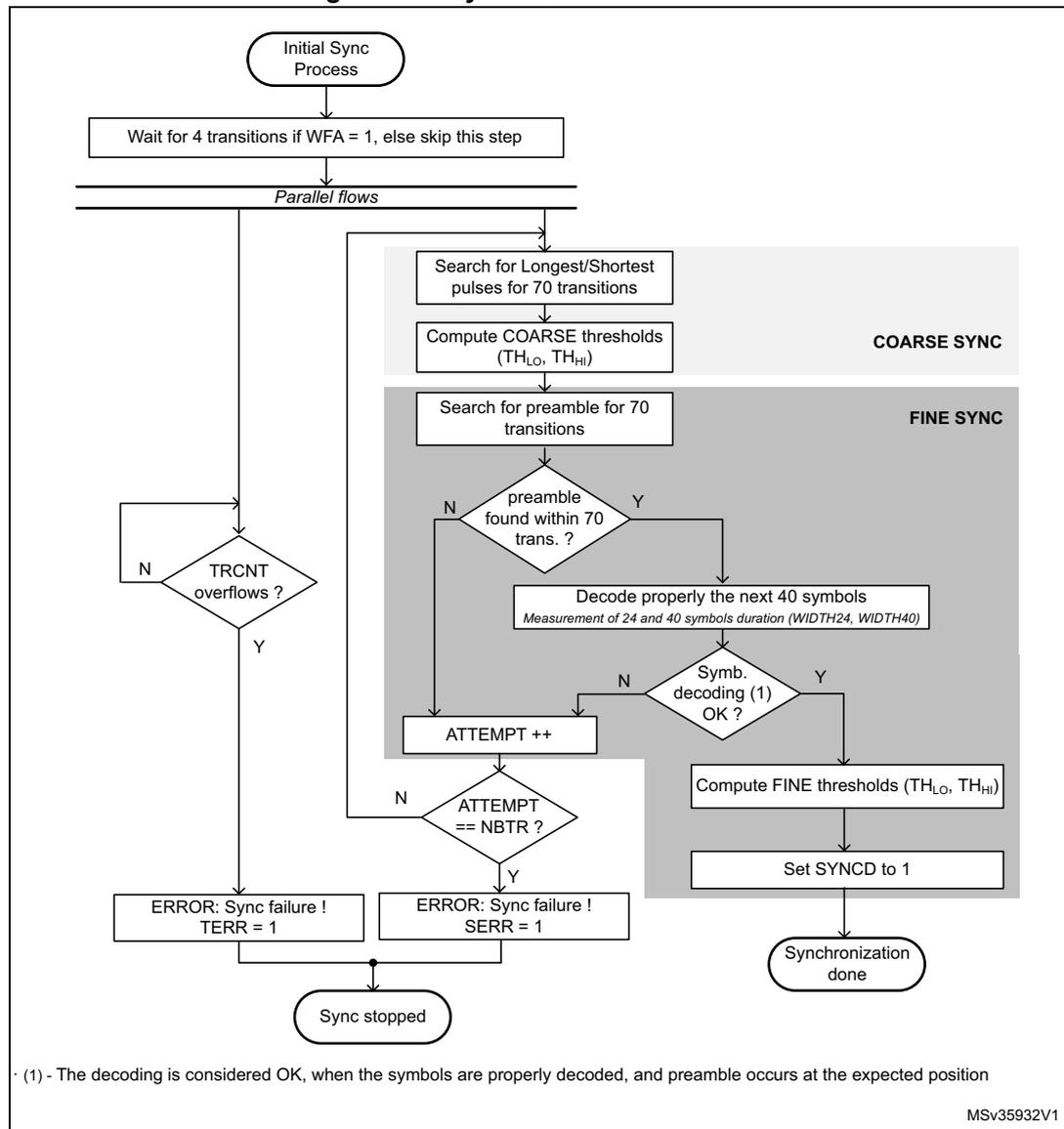
Refer to [Frame structure and synchronization error](#) for additional information concerning TRCNT overflow.
