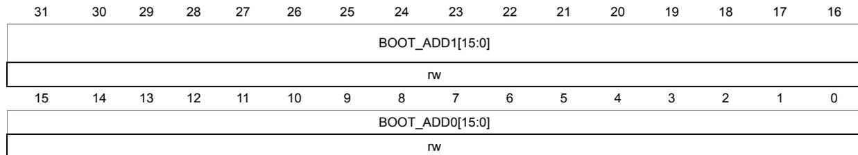
Bits 31:16 **BOOT\_ADD1[15:0]**: Boot base address when Boot pin =1
