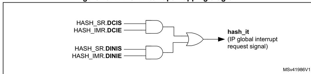
The above interrupt sources can be enabled or disabled individually by changing the mask bits in the HASH\_IMR register. Setting the appropriate mask bit to 1 enables the interrupt.
