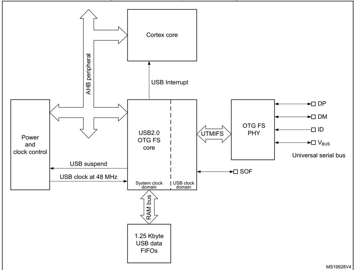
Figure 510. OTG high-speed block diagram
