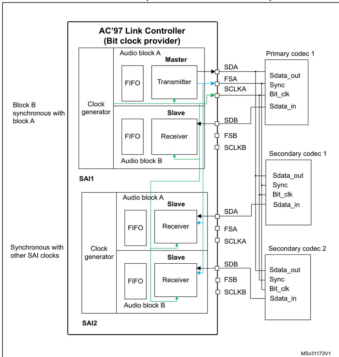
In receiver mode, the SAI acting as an AC'97 link controller requires no FIFO request and so no data storage in the FIFO when the Codec ready bit in the slot 0 is decoded low. If bit CNRDYIE is enabled in the SAI\_xIM register, flag CNRDY will be set in the SAI\_xSR register and an interrupt is generated. This flag is dedicated to the AC'97 protocol.
