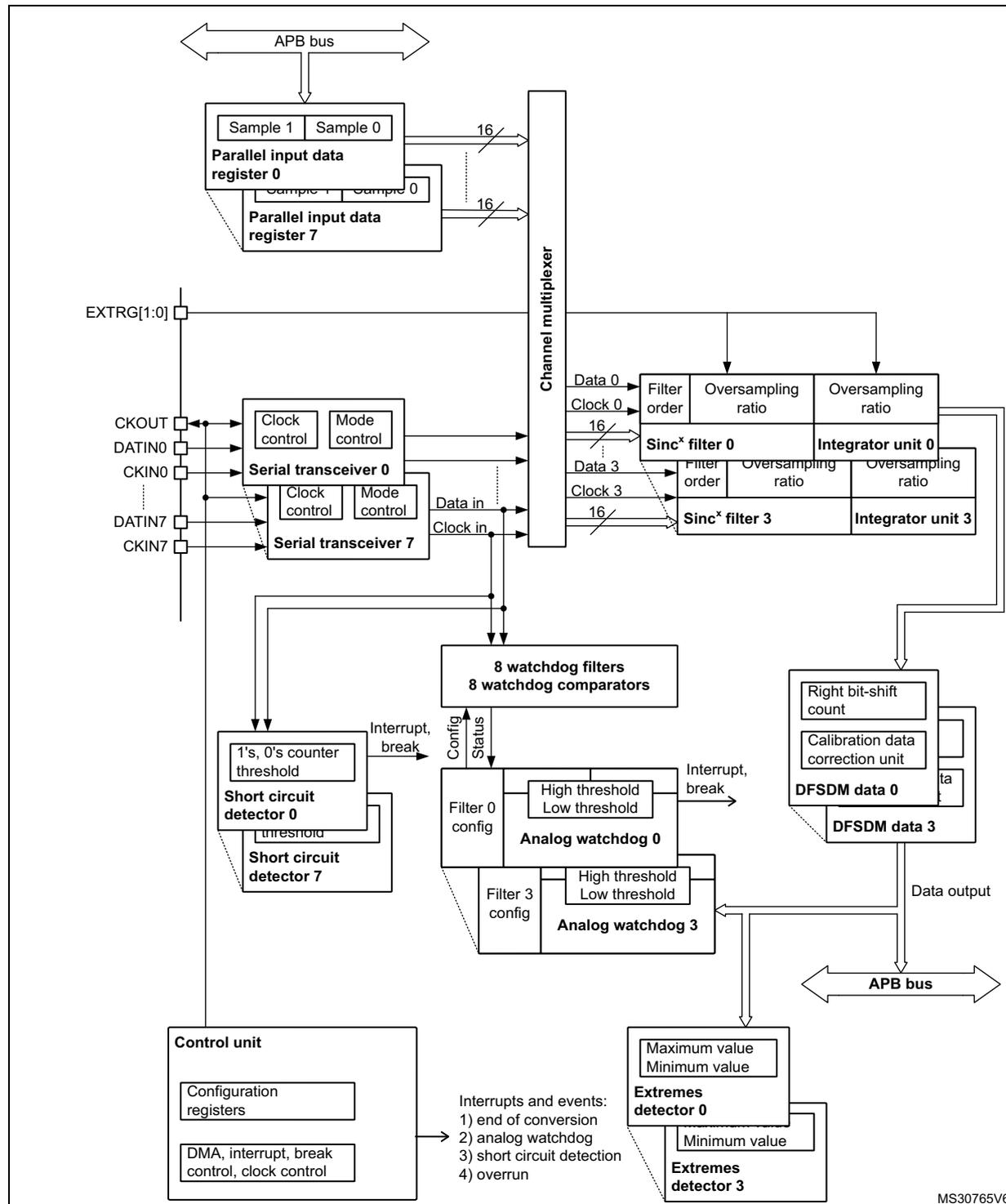
1. This example shows 4 DFSDM filters and 8 input channels (max. configuration).
