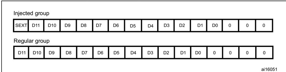
Special case: when left-aligned, the data are aligned on a half-word basis except when the resolution is set to 6-bit. In that case, the data are aligned on a byte basis as shown in [Figure 79](#).
