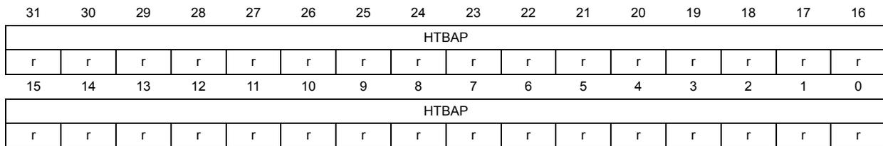
Bits 31:0 **HTBAP**: Host transmit buffer address pointer
