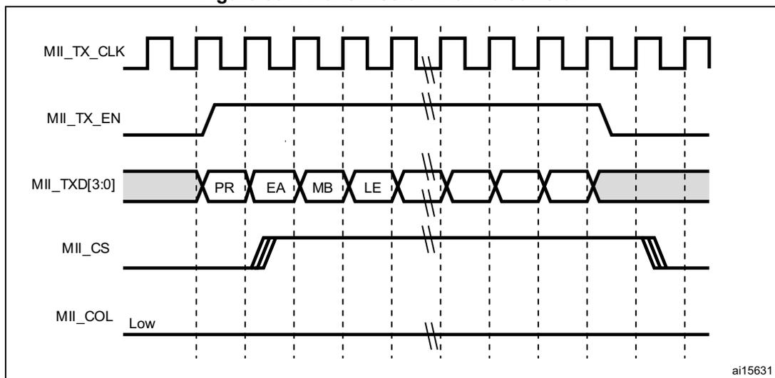
Figure 555. Transmission with collision
