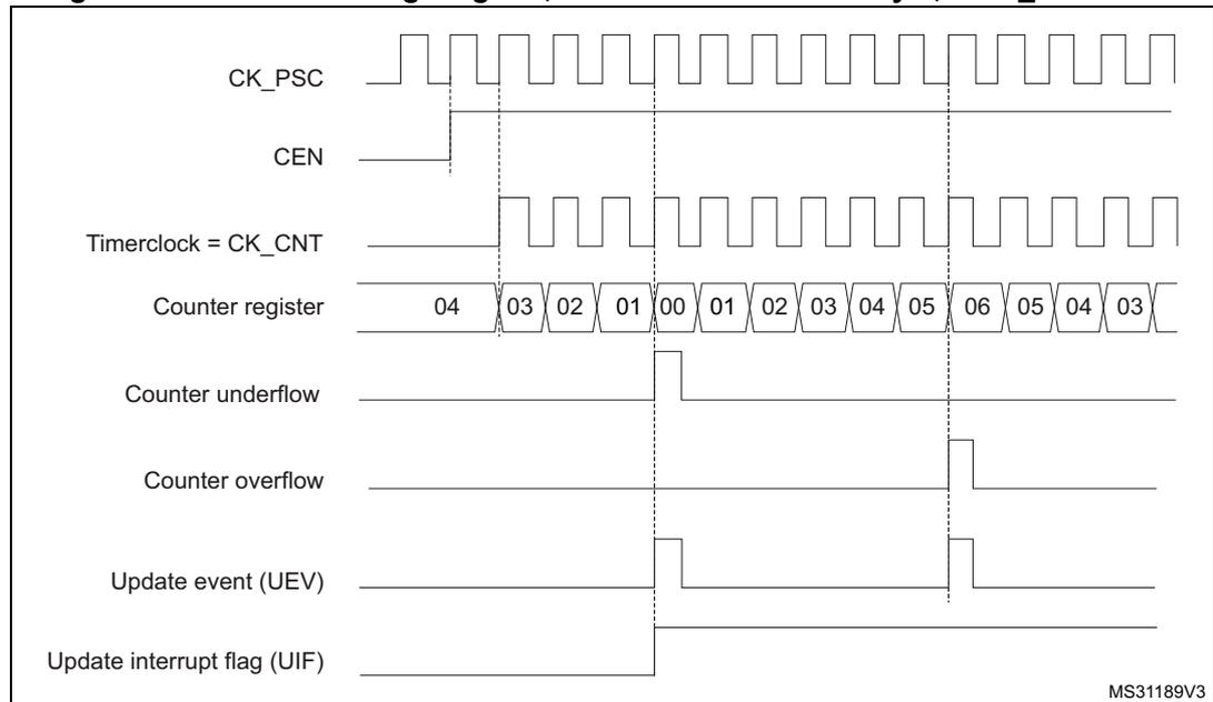
1. Here, center-aligned mode 1 is used (for more details refer to [Section 25.4: TIM1/TIM8 registers](#)).
