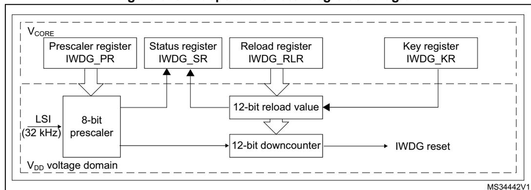
1. The watchdog function is implemented in the  $V_{CORE}$  voltage domain that is still functional in Stop and Standby modes.
