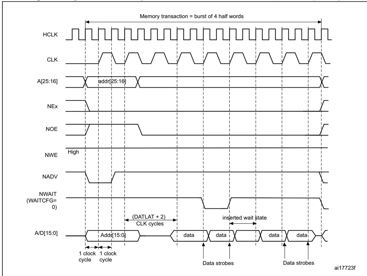
1. Byte lane outputs (NBL are not shown; for NOR access, they are held high, and, for PSRAM (CRAM) access, they are held low.
