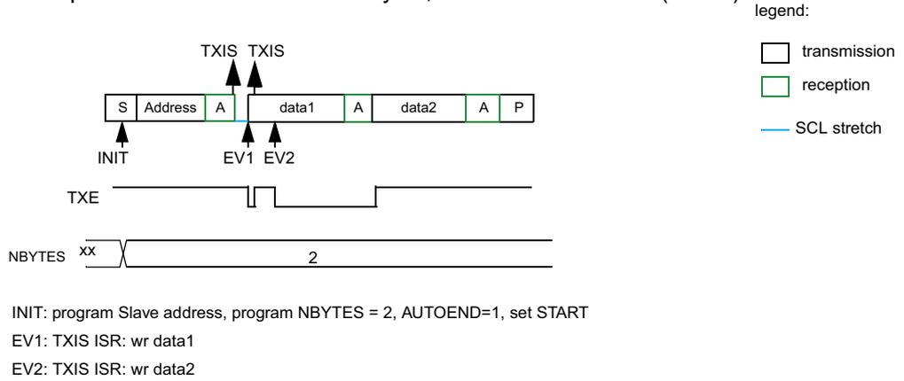
Example I2C master transmitter 2 bytes, software end mode (RESTART)
