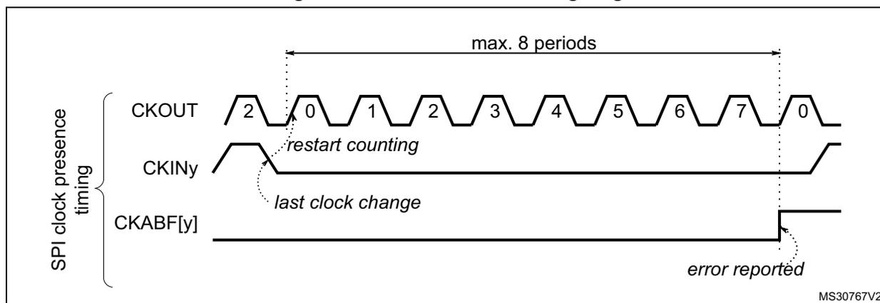
If Manchester data format is used, then the clock absence means that the clock recovery is unable to perform from Manchester coded signal. For a correct clock recovery, it is first necessary to receive data with 1 to 0 or 0 to 1 transition (see [Figure 107](#) for Manchester synchronization).
