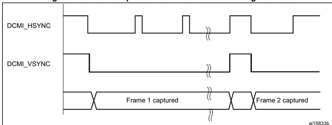
1. Here, the active state of DCMI\_HSYNC and DCMI\_VSYNC is 1.
