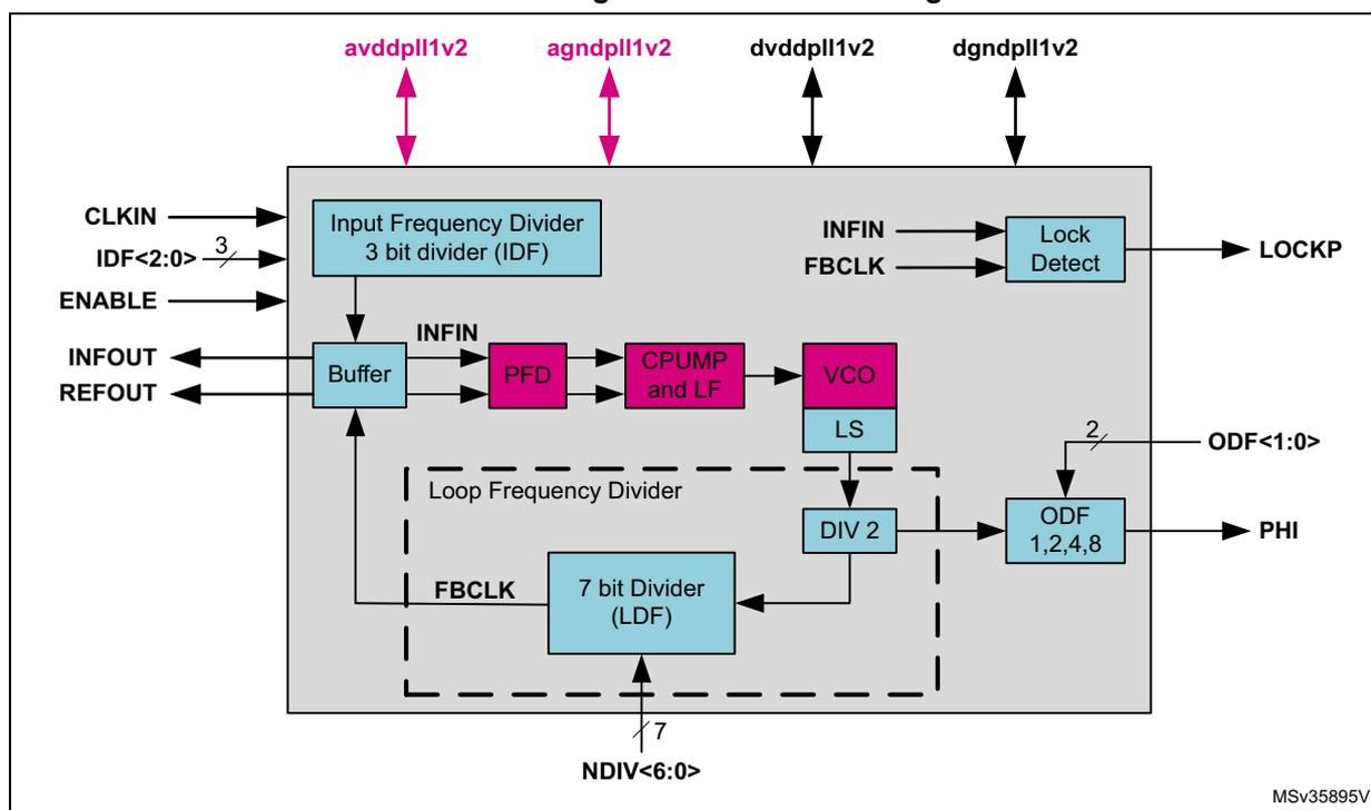
The PLL output frequency is configured through the DSI\_WRPCR register fields. The VCO frequency and the PLL output frequency are calculated as follows:
