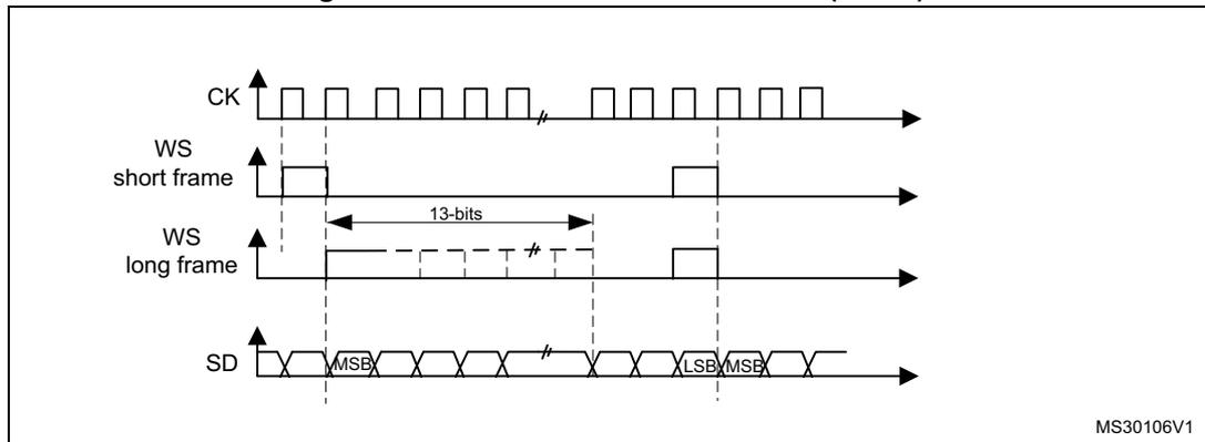
For long frame synchronization, the WS signal assertion time is fixed to 13 bits in master mode.
