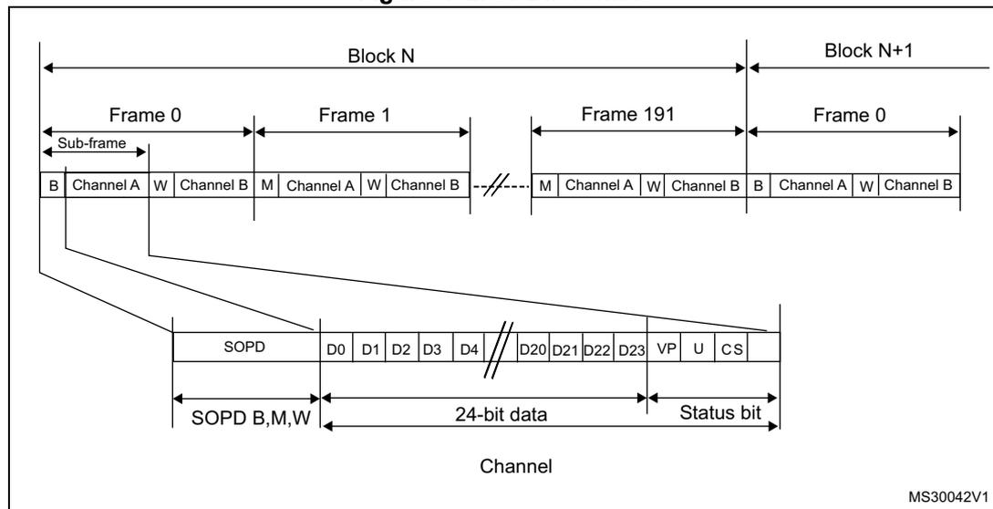
A SPDIF block contains 192 frames. Each frame is composed of two 32-bit sub-frames, generally one for the left channel and one for the right channel. Each sub-frame is composed of a SOPD pattern (4-bit) to specify if the sub-frame is the start of a block (and so is identifying a channel A) or if it is identifying a channel A somewhere in the block, or if it is referring to channel B (see [Table 236](#)). The next 28 bits of channel information are composed of 24 bits data + 4 status bits.
