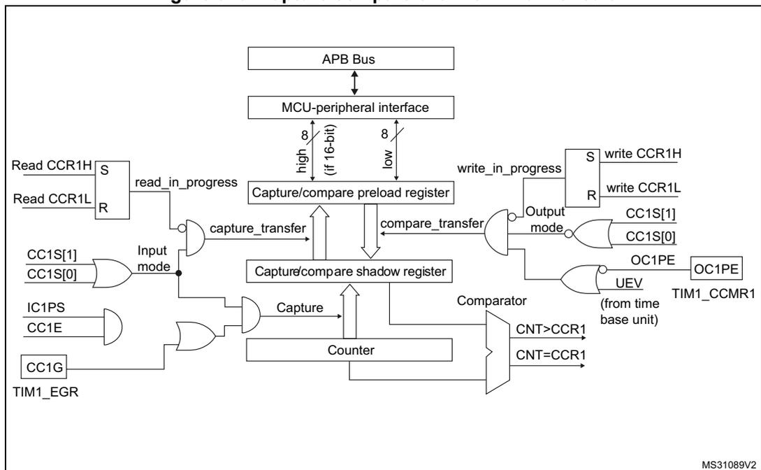
Figure 317. Output stage of capture/compare channel (channel 1)
