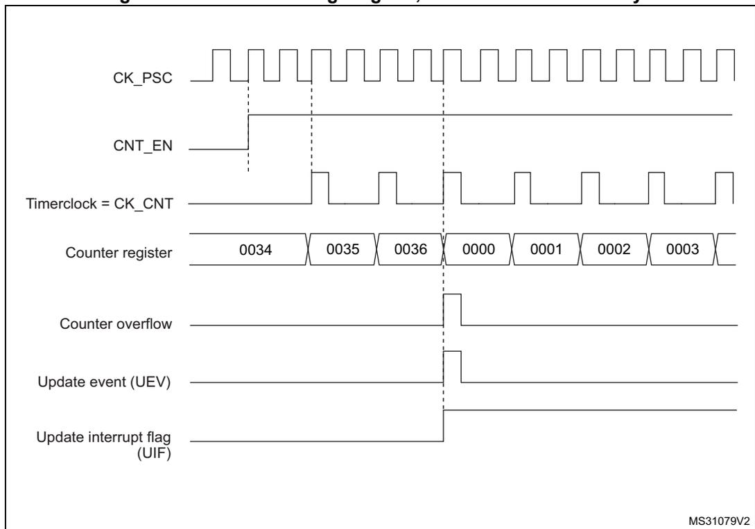
Figure 200. Counter timing diagram, internal clock divided by 4
