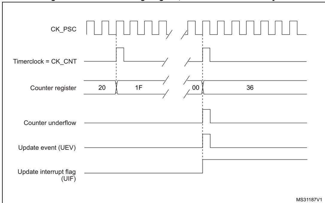
**Figure 266. Counter timing diagram, Update event when repetition counter is not used**
