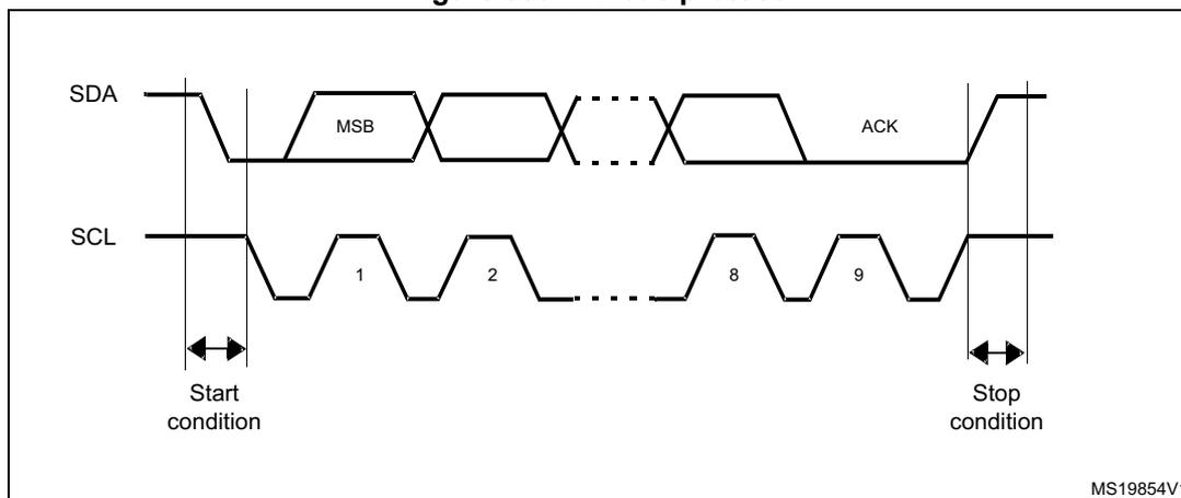
Acknowledge can be enabled or disabled by software. The I2C interface addresses can be selected by software.
