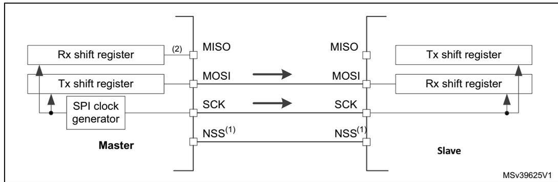
1. The NSS pins can be used to provide a hardware control flow between master and slave. Optionally, the pins can be left unused by the peripheral. Then the flow has to be handled internally for both master and slave. For more details see [Section 35.5.5: Slave select \(NSS\) pin management](#).
