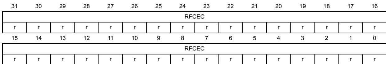
Bits 31:0 **RFCEC**: Received frames CRC error counter
