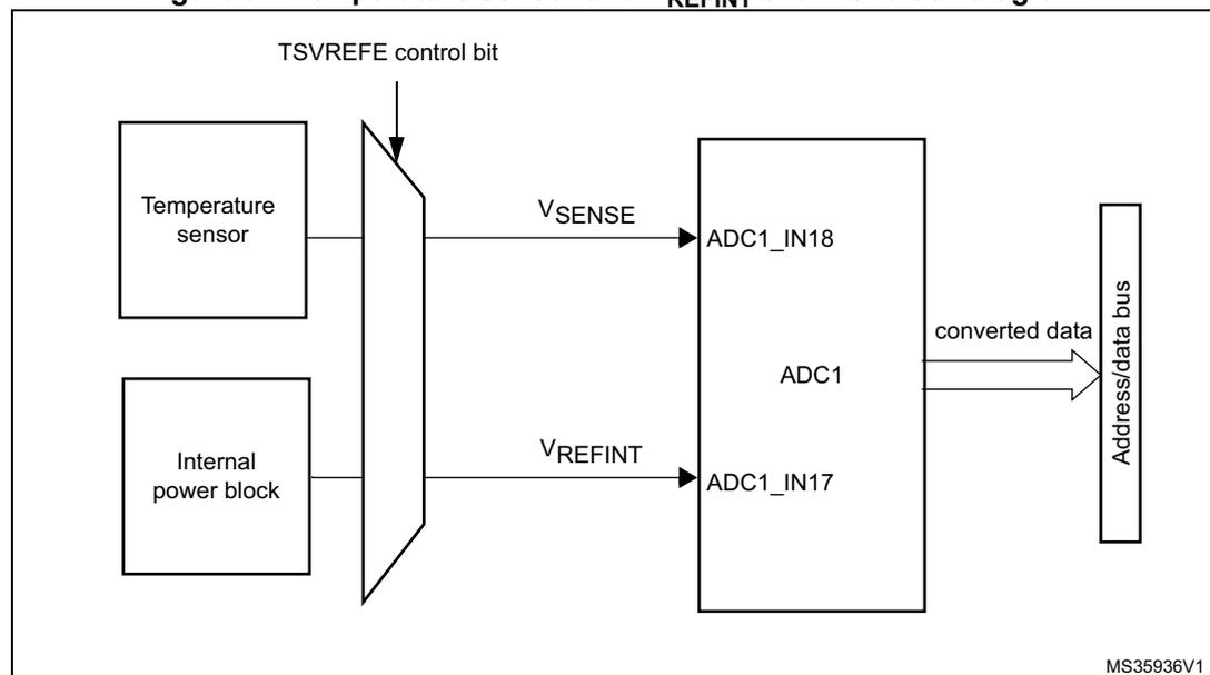
1.  $V_{SENSE}$  is input to *ADC1\_IN18*.
