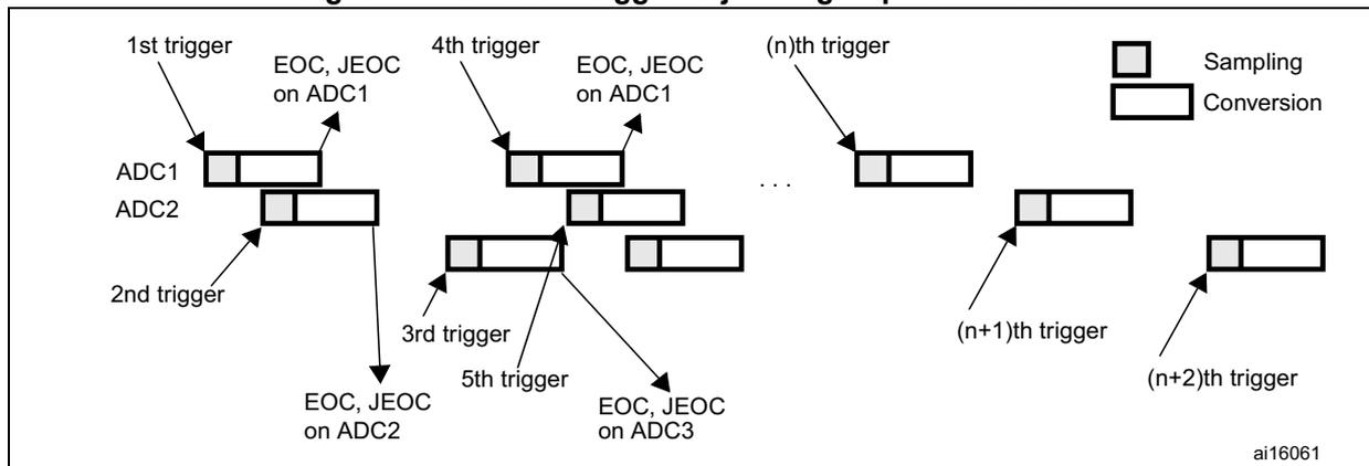
**15.9.5 Combined regular/injected simultaneous mode**
