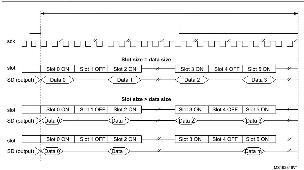
If the TRIS bit in the SAI\_xCR2 register is cleared, all the High impedance states on the SD output line on [Figure 455](#) and [Figure 456](#) are replaced by a drive with a value of 0.
