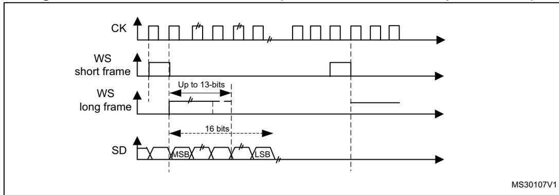
*Note:* For both modes (master and slave) and for both synchronizations (short and long), the number of bits between two consecutive pieces of data (and so two synchronization signals) needs to be specified (DATLEN and CHLEN bits in the SPIx\_I2SCFGR register) even in slave mode.
