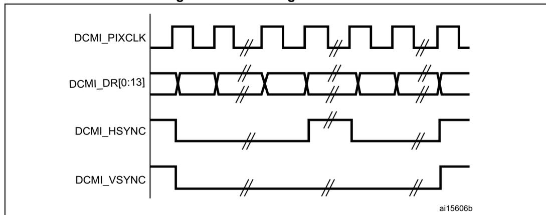
1. The capture edge of DCMI\_PIXCLK is the falling edge, the active state of DCMI\_HSYNC and DCMI\_VSYNC is 1.
