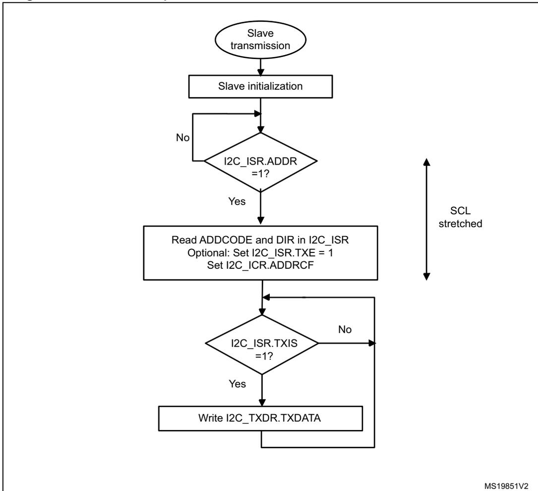
Figure 357. Transfer sequence flowchart for I2C slave transmitter, NOSTRETCH=1
