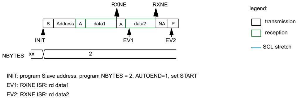
Example I2C master receiver 2 bytes, software end mode (RESTART)
