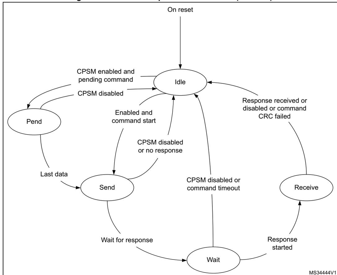
When the Wait state is entered, the command timer starts running. If the timeout is reached before the CPSM moves to the Receive state, the timeout flag is set and the Idle state is entered.
