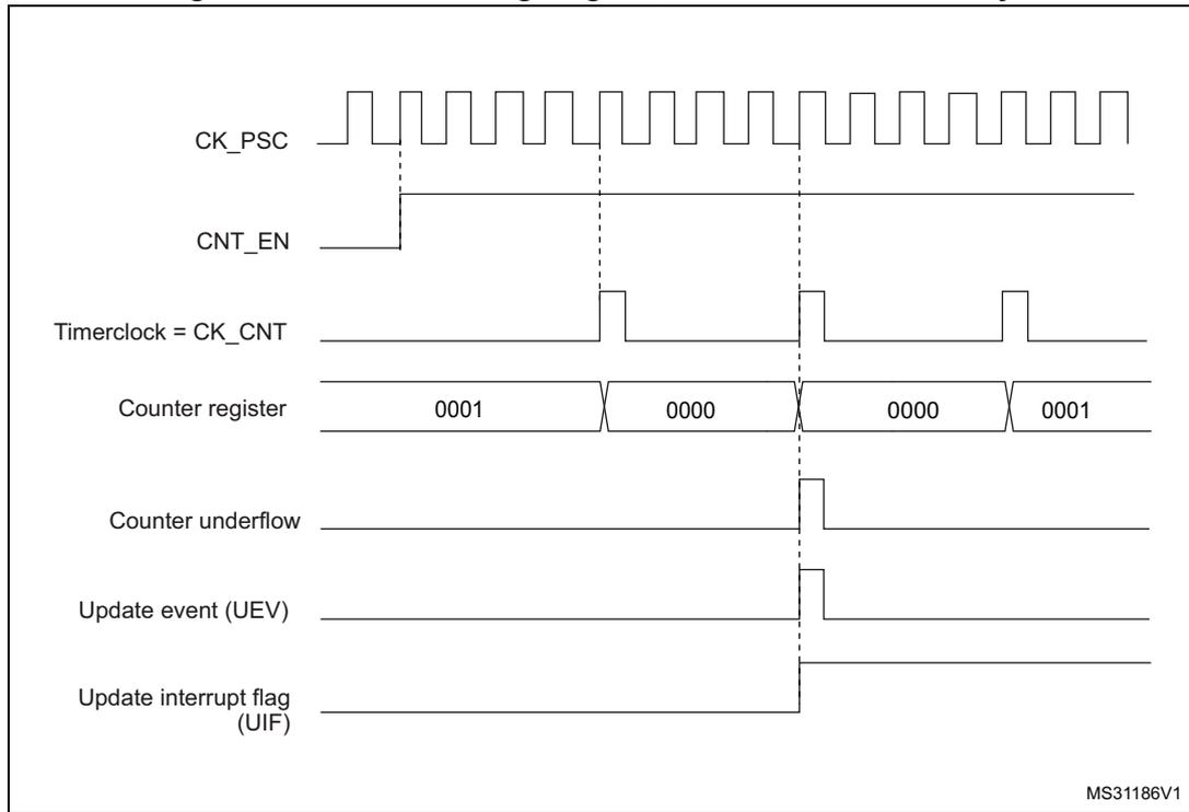
Figure 207. Counter timing diagram, internal clock divided by N
