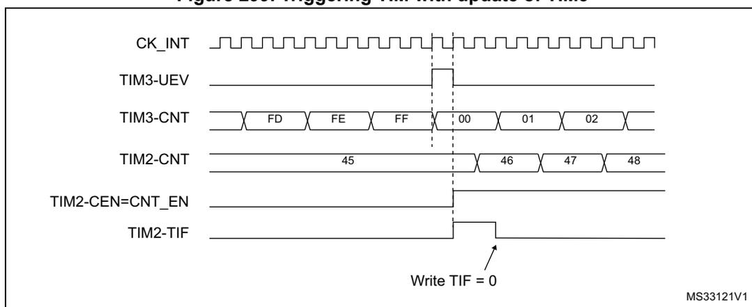
As in the previous example, you can initialize both counters before starting counting. [Figure 300](#) shows the behavior with the same configuration as in [Figure 299](#) but in trigger mode instead of gated mode (SMS=110 in the TIM\_SMCR register).
