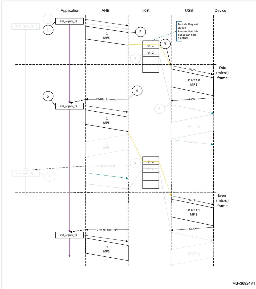
• **Interrupt IN transactions in DMA mode**
