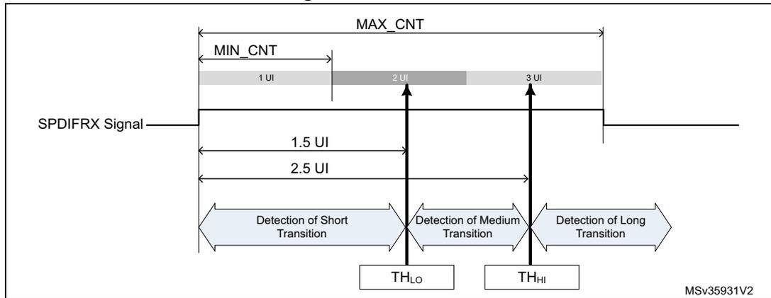
The preamble detector checks four consecutive transitions of a specific sequence to determine if they form the part of preamble. Let us say TRANS0, TRANS1, TRANS2 and TRANS3 represent four consecutive transitions encoded as mentioned above. [Table 241](#) shows the values of these four transitions to form a preamble. Absence of this pattern indicates that these transitions form part of the data in the sub frame and bi-phase decoder will decode them.
