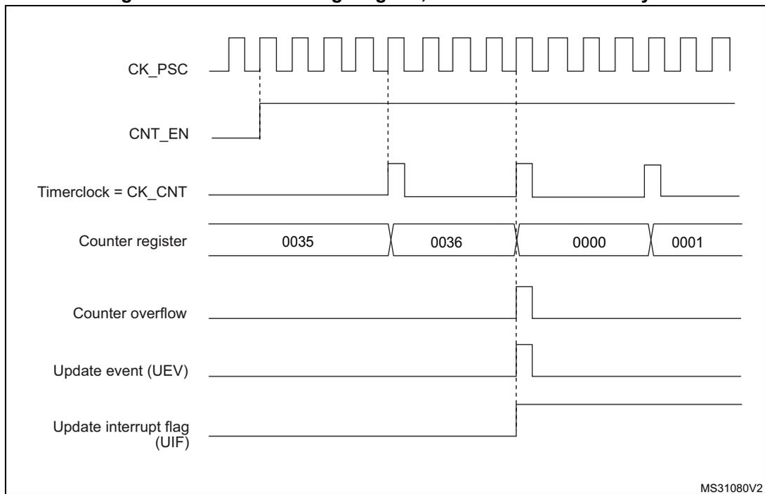
Figure 309. Counter timing diagram, internal clock divided by N
