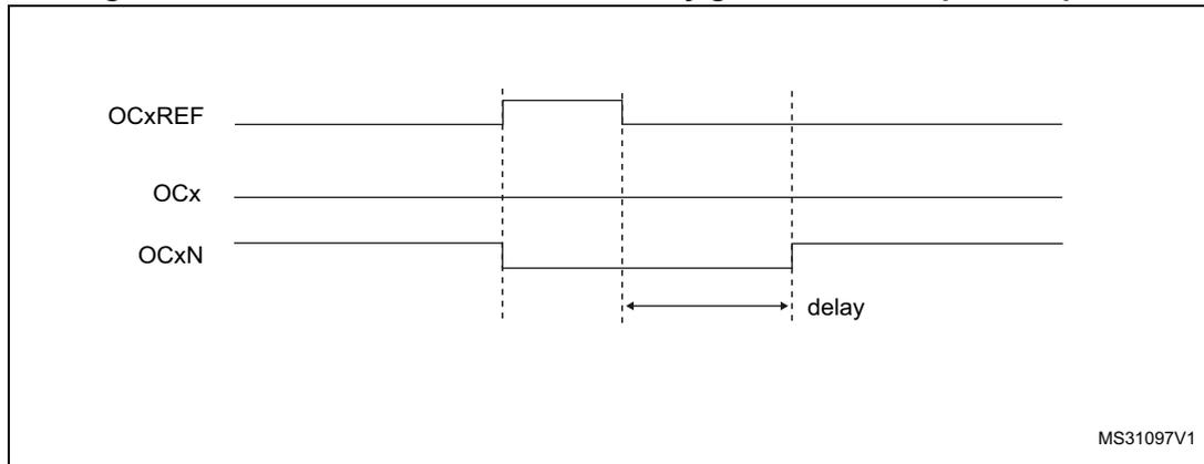
The dead-time delay is the same for each of the channels and is programmable with the DTG bits in the TIMx\_BDTR register. Refer to [Section 25.4.18: TIM1/TIM8 break and dead-time register \(TIMx\\_BDTR\)](#) for delay calculation.
