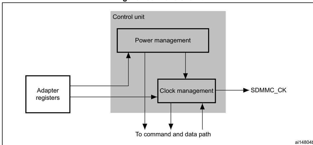
The control unit is illustrated in [Figure 485](#). It consists of a power management subunit and a clock management subunit.
