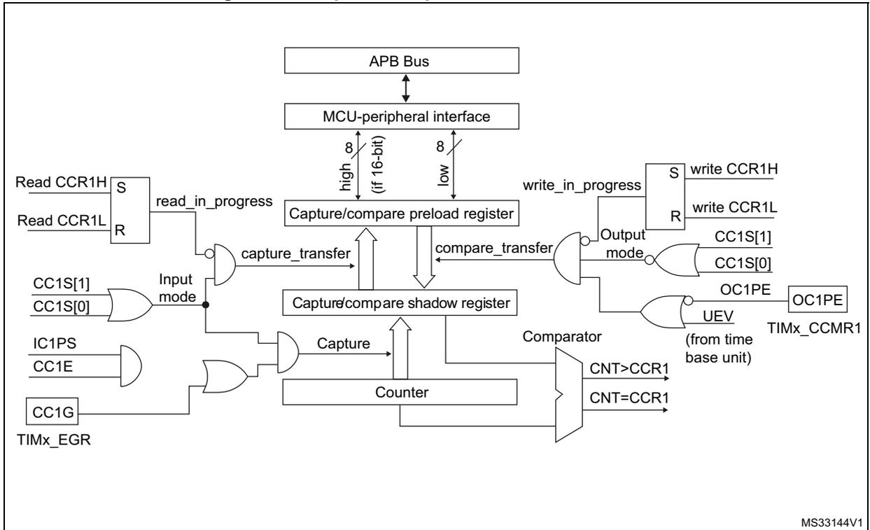
Figure 280. Output stage of capture/compare channel (channel 1)
