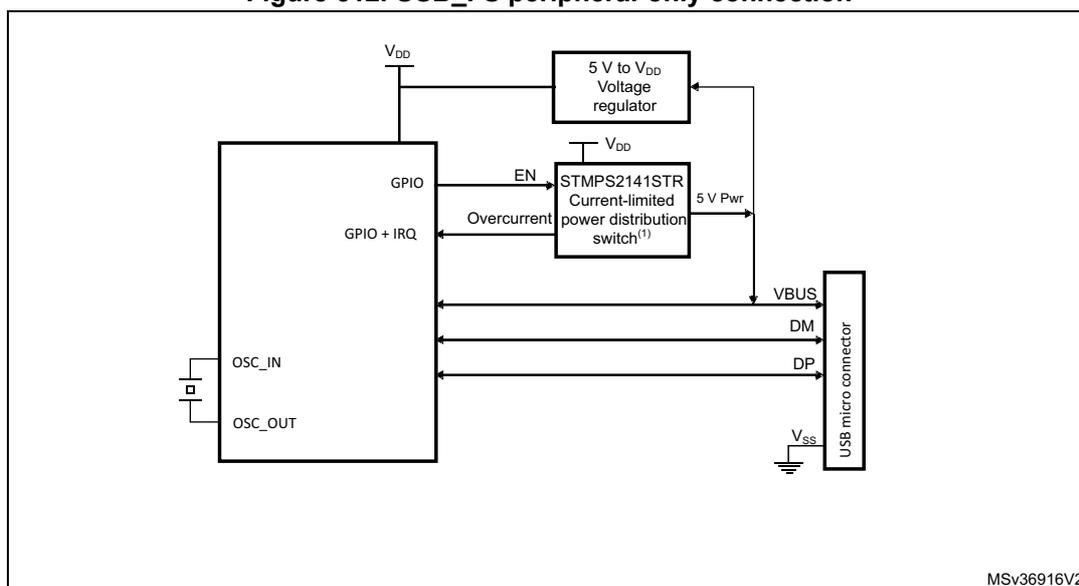
1. Use a regulator to build a bus-powered device.
