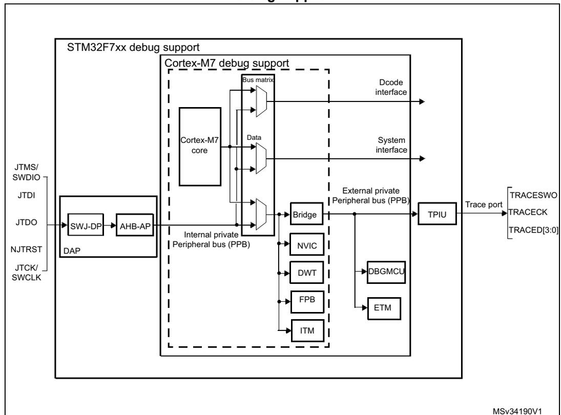
*Note:* The debug features embedded in the Cortex<sup>®</sup>-M7 with FPU core are a subset of the Arm<sup>®</sup> CoreSight Components Technical Reference Manual.
