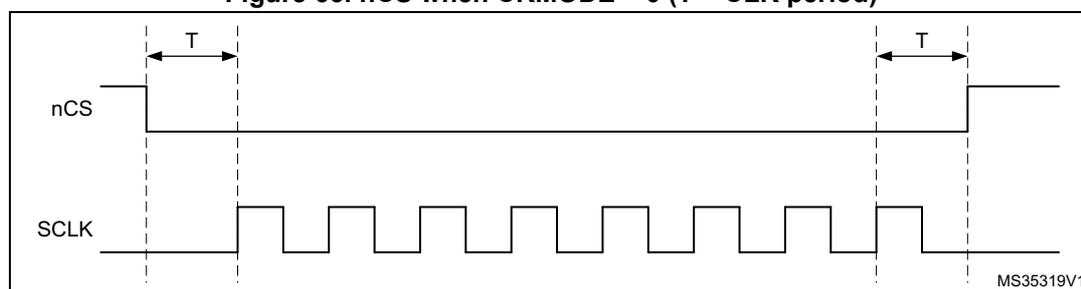
When CKMODE=1 (“mode3”, where CLK goes high when no operation is in progress) and DDRM=0 (SDR mode), nCS still falls one CLK cycle before an operation first rising CLK edge, and nCS rises one CLK cycle after the operation final rising CLK edge, as shown in [Figure 67](#).
