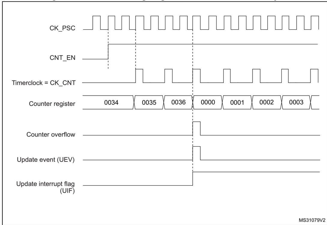
**Figure 308. Counter timing diagram, internal clock divided by 4**
