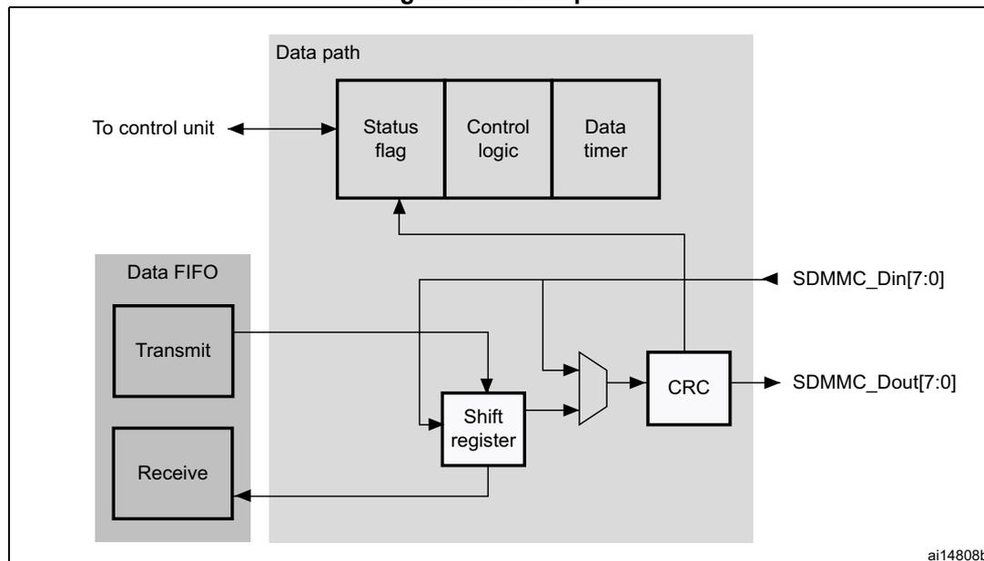
The card databus width can be programmed using the clock control register. If the 4-bit wide bus mode is enabled, data is transferred at four bits per clock cycle over all four data signals (SDMMC\_D[3:0]). If the 8-bit wide bus mode is enabled, data is transferred at eight bits per clock cycle over all eight data signals (SDMMC\_D[7:0]). If the wide bus mode is not enabled, only one bit per clock cycle is transferred over SDMMC\_D0.
