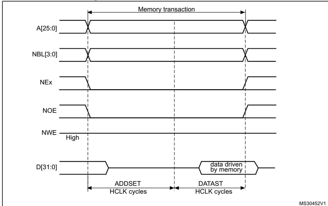
**Figure 36. Mode1 write access waveforms**
