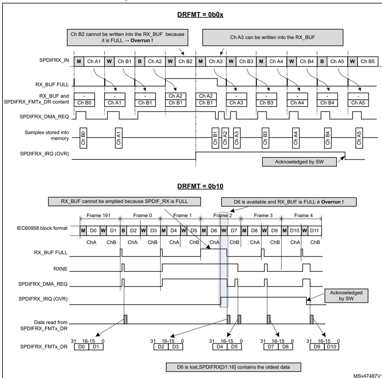
If the RXSTEO bit is set to 1, it means that stereo data are transported, then the SPDIFRX has to avoid misalignment between left and right channels. So the peripheral has to drop a second sample even if there is room inside the RX\_BUF in order to avoid misalignment. Then the incoming samples can be written normally into the RX\_BUF even if the OVR flag is still pending. Refer to [Figure 473](#).
