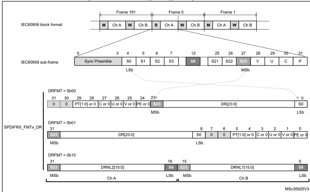
Setting DRFMT to 0b00 or 0b01, offers the possibility to have the data either right or left aligned into the SPDIFRX\_FMTx\_DR register. The status information can be enabled or forced to zero according to the way the software wants to handle them.
