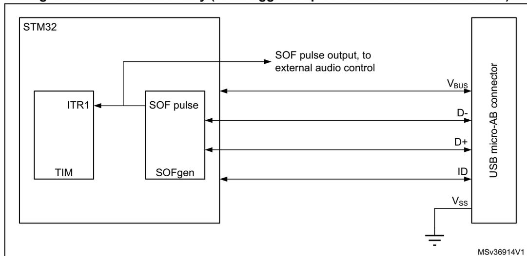
The OTG\_FS/OTG\_HS core provides means to monitor, track and configure SOF framing in the host and peripheral, as well as an SOF pulse output connectivity feature.
