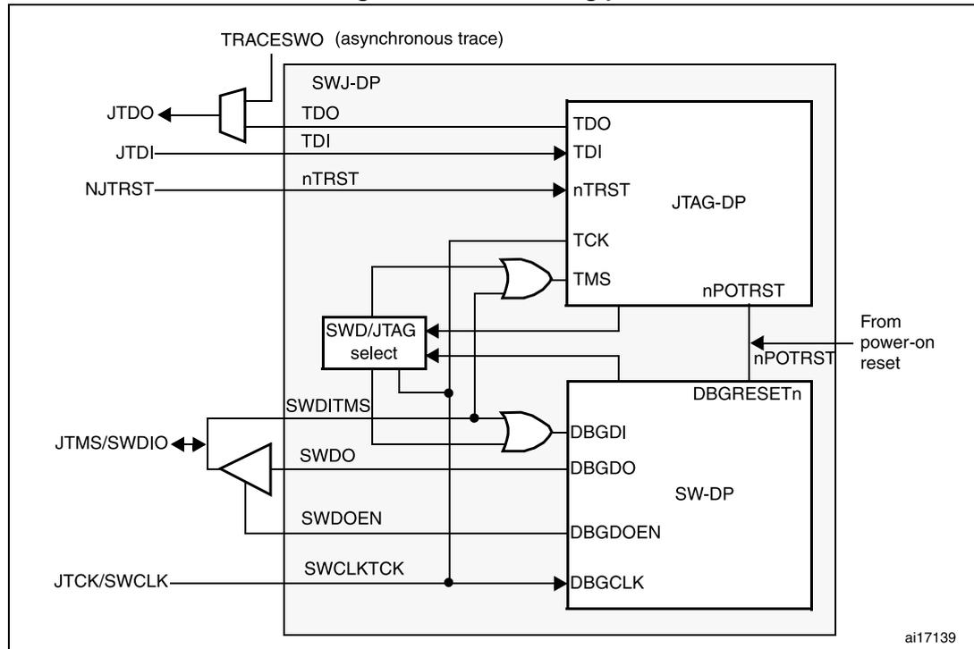
Figure 588 shows that the asynchronous TRACE output (TRACESWO) is multiplexed with TDO. This means that the asynchronous trace can only be used with SW-DP, not JTAG-DP.
