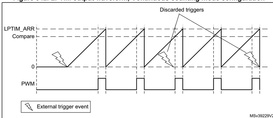
SNGSTRT and CNTSTRT bits can only be set when the timer is enabled (The ENABLE bit is set to '1'). It is possible to change “on the fly” from One-shot mode to Continuous mode.
