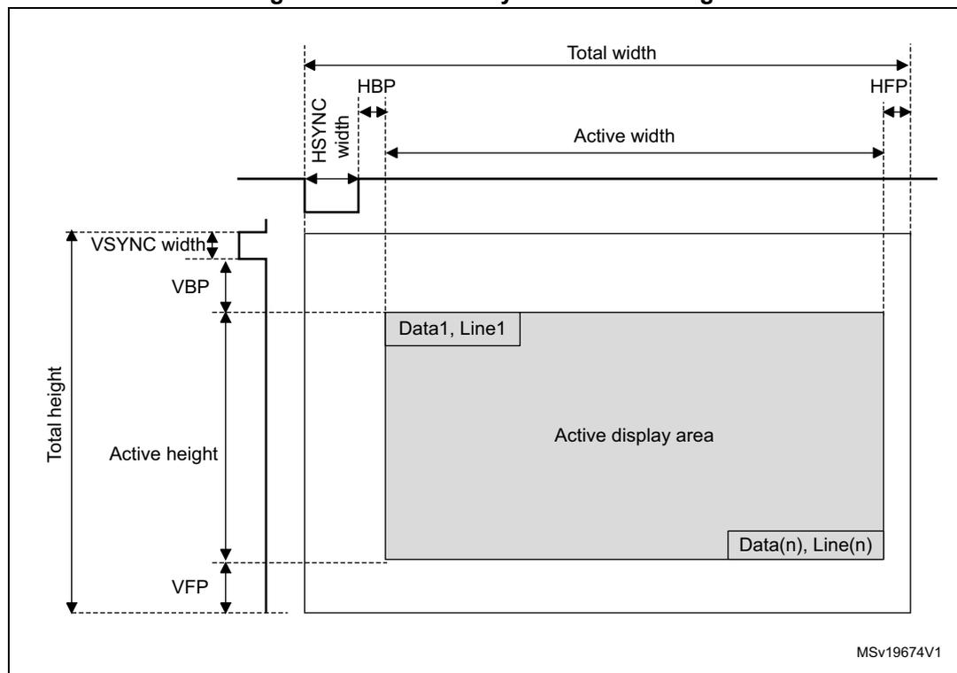
Note: The HBP and HFP are respectively the horizontal back porch and front porch period. The VBP and the VFP are respectively the vertical back porch and front porch period.
