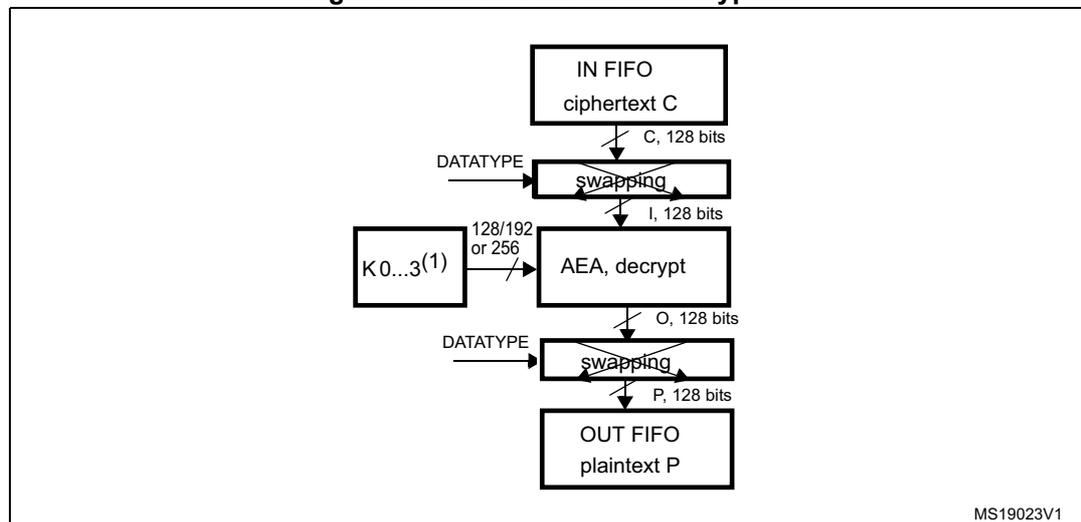
1. K: key; C: cipher text; I: input block; O: output block; P: plain text.
