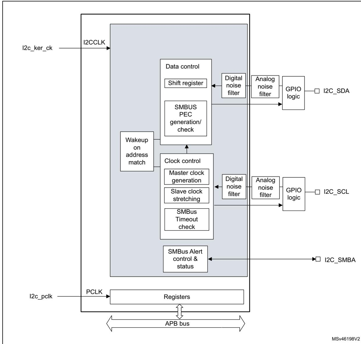
The I2C is clocked by an independent clock source which allows to the I2C to operate independently from the PCLK frequency.
