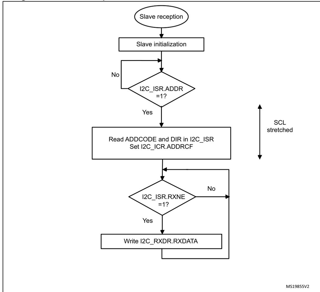
Figure 360. Transfer sequence flowchart for slave receiver with NOSTRETCH=1
