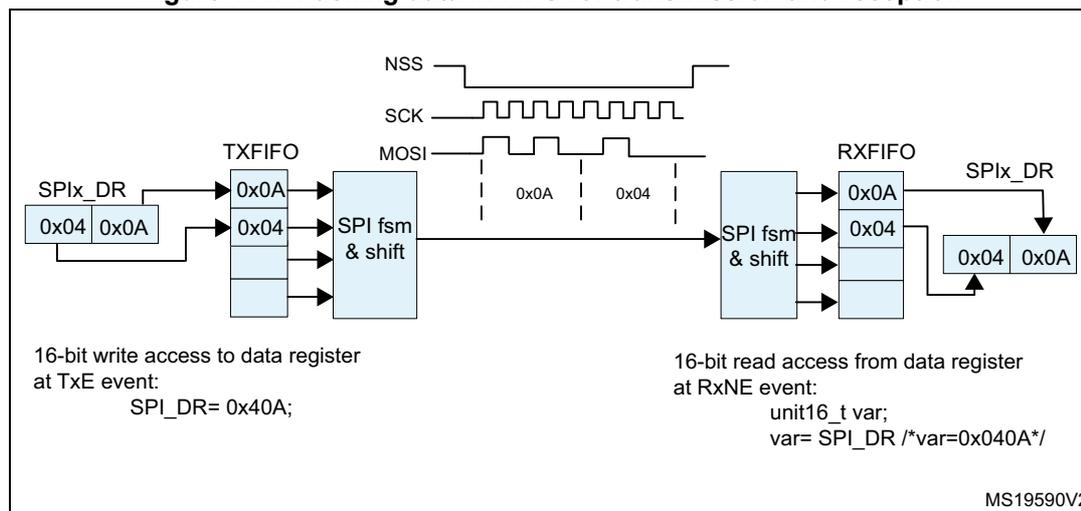
1. In this example: Data size DS[3:0] is 4-bit configured, CPOL=0, CPHA=1 and LSBFIRST =0. The Data storage is always right aligned while the valid bits are performed on the bus only, the content of LSB byte goes first on the bus, the unused bits are not taken into account on the transmitter side and padded by zeros at the receiver side.
