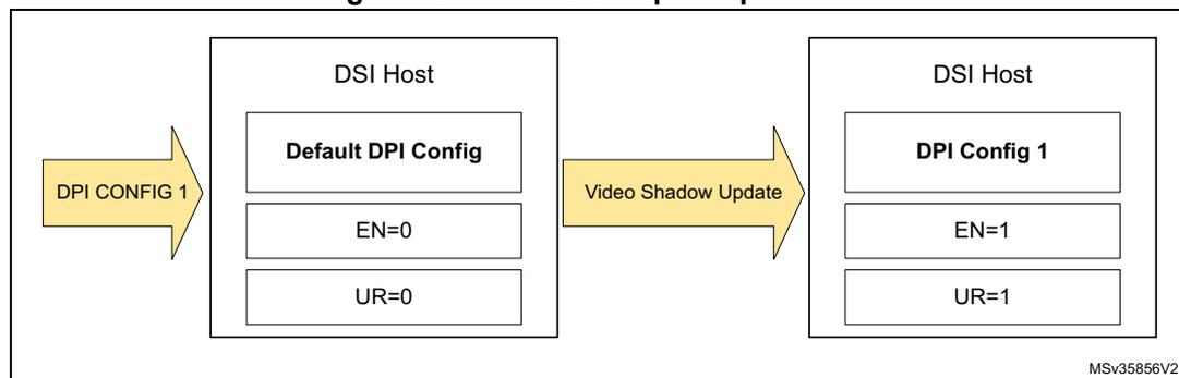
**Updating the configuration during the transmission of a frame using APB**
