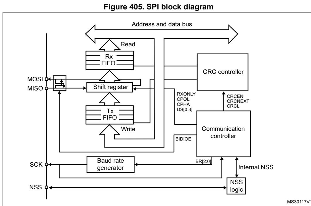
Four I/O pins are dedicated to SPI communication with external devices.
