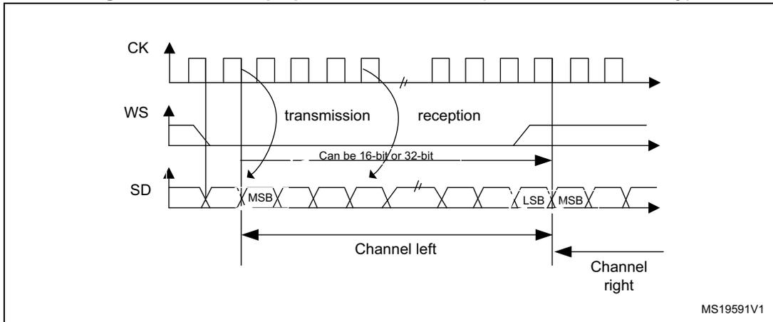
Data are latched on the falling edge of CK (for the transmitter) and are read on the rising edge (for the receiver). The WS signal is also latched on the falling edge of CK.
