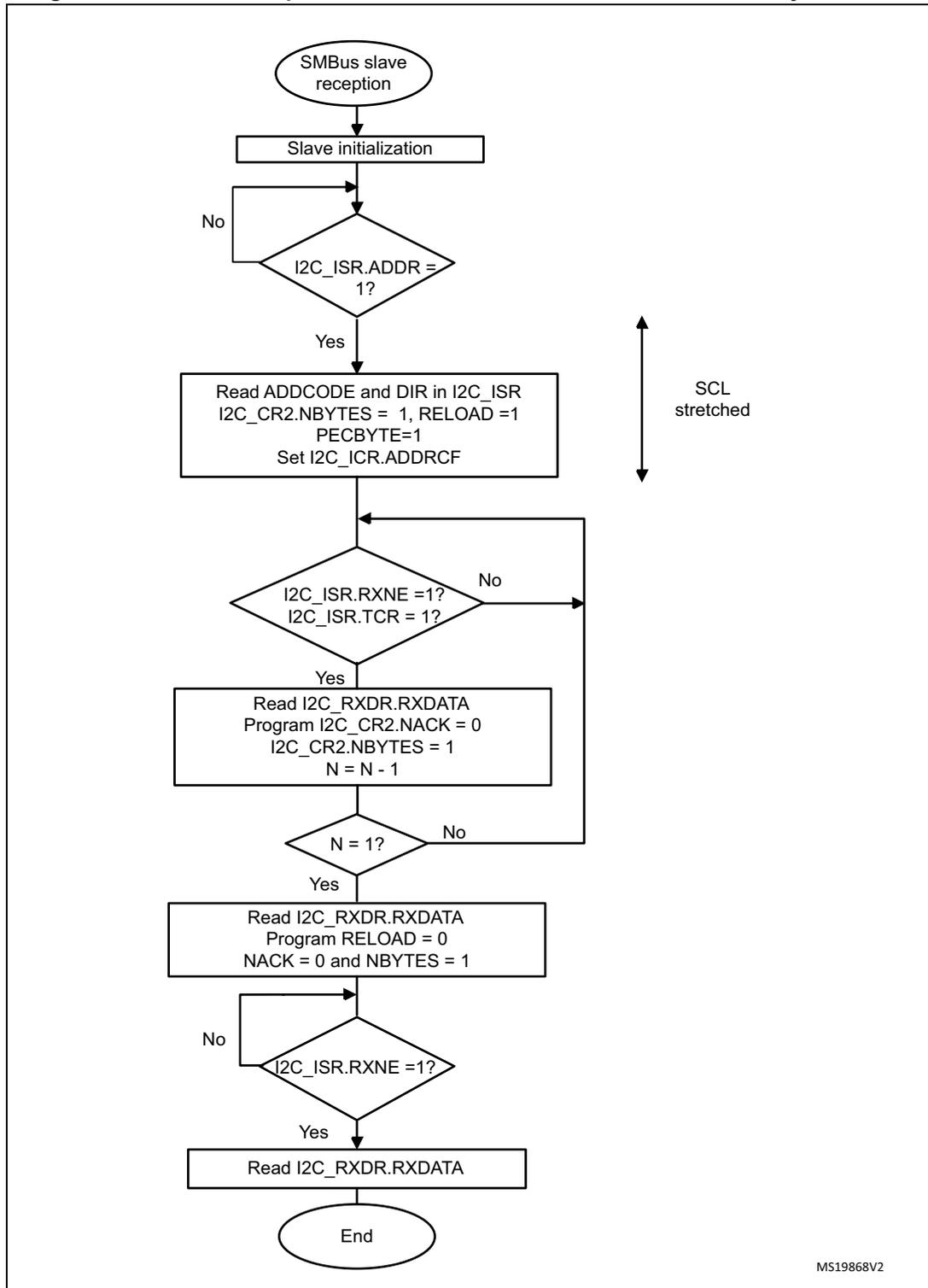
**Figure 376. Bus transfer diagrams for SMBus slave receiver (SBC=1)**
