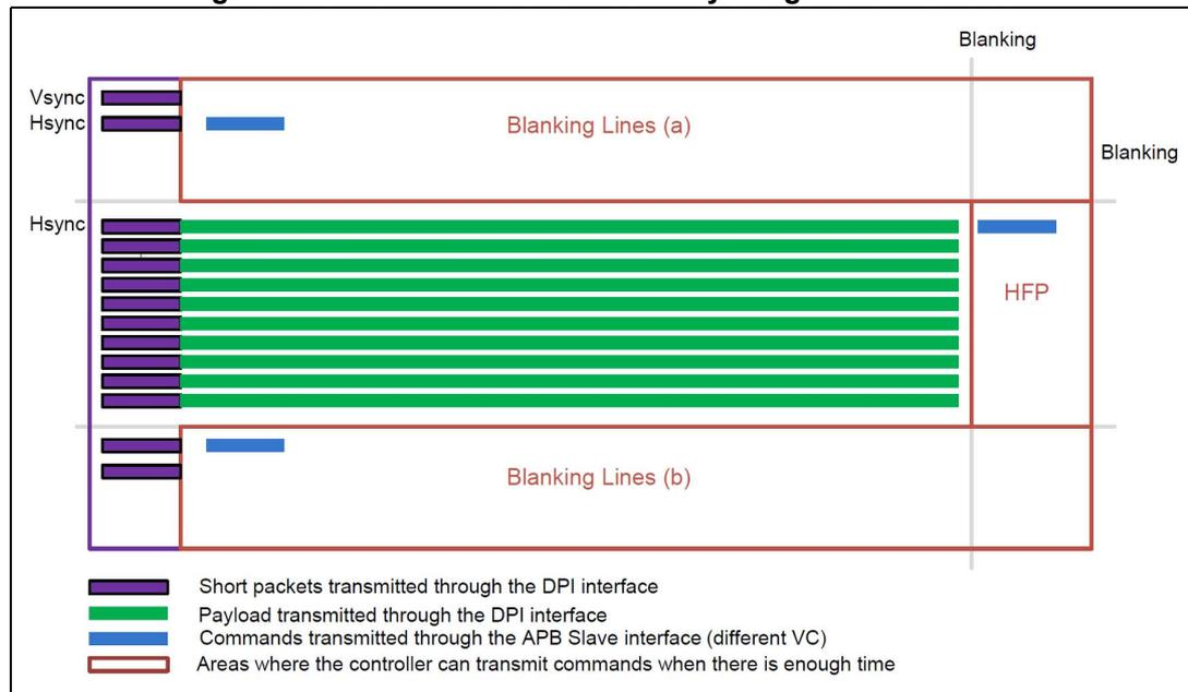
It is also possible to address the multiple displays with only the generic interface using different virtual channels. Because the generic interface is not restricted to any particular virtual channel through configuration, it is possible to issue the packets with different virtual channels. This enables the interface to time multiplex the packets to be provided to the displays with different virtual channels.
