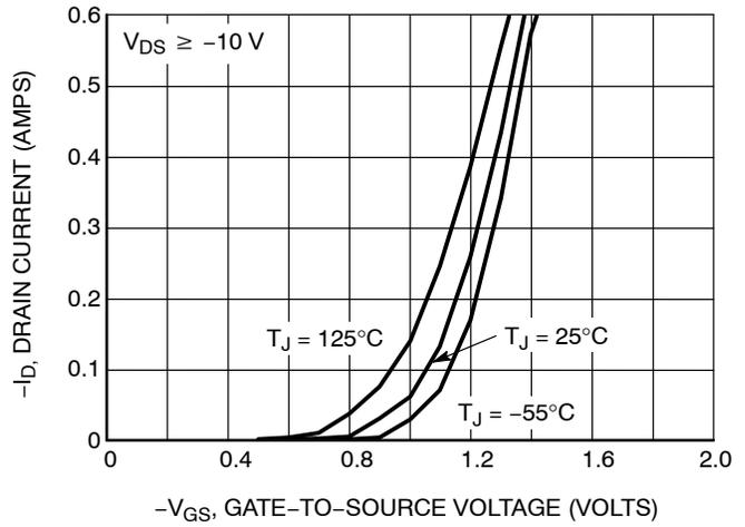
Figure 2. Transfer Characteristics
