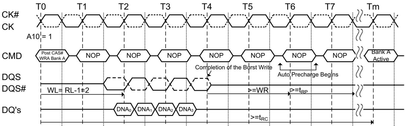
**Figure 45. Burst write with auto-precharge (WR+t<sub>RP</sub>): WL=4, WR=2, BL=4, t<sub>RP</sub>=3**
