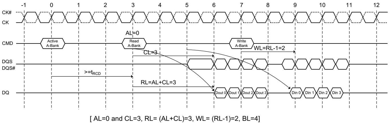
**Figure 20. Data output (read) timing**
