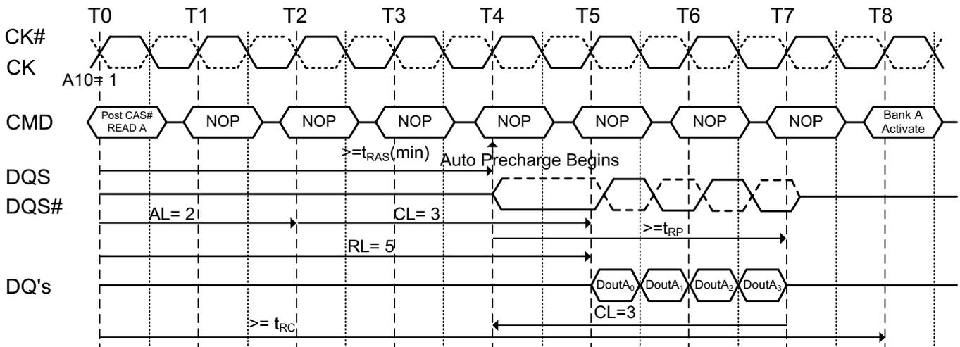
**Figure 43. Burst read operation with auto precharge followed by an activation to the same bank ( $t_{RP}$  Limit): (RL=5 (AL=2, CL=3, internal  $t_{RCD}$ =3, BL=4,  $t_{RTP} \leq 2$  clocks)**
