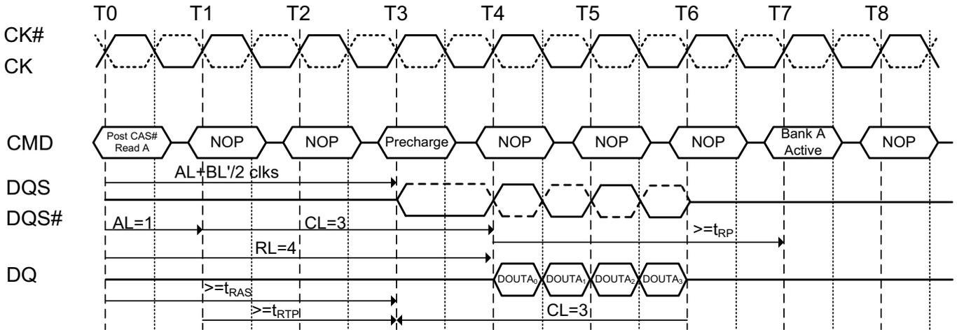
**Figure 34. Burst read operation followed by precharge:**
