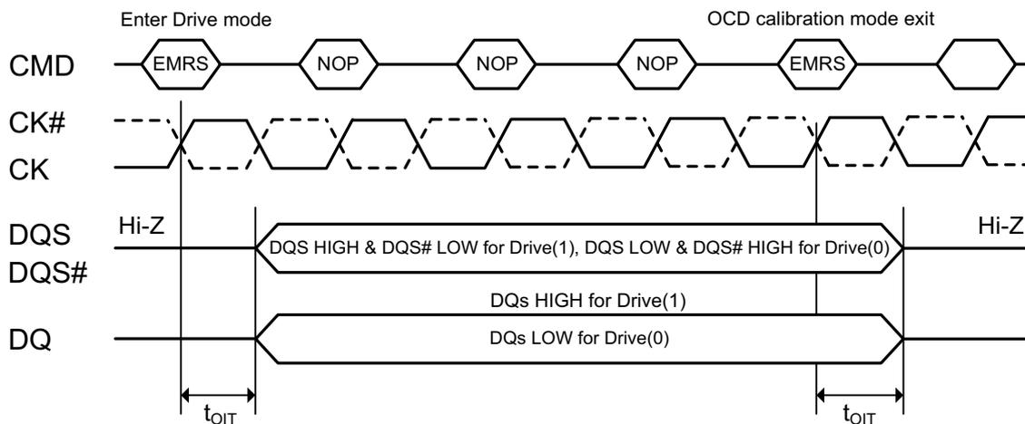
**NOTE :** Drive mode, both Drive(1) and Drive(0), is used for controllers to measure DDR2 SDRAM Driver impedance. In this mode, all outputs are driven out  $t_{OIT}$  after "enter drive mode" command and all output drivers are turned-off  $t_{OIT}$  after "OCD calibration mode exit" command.
