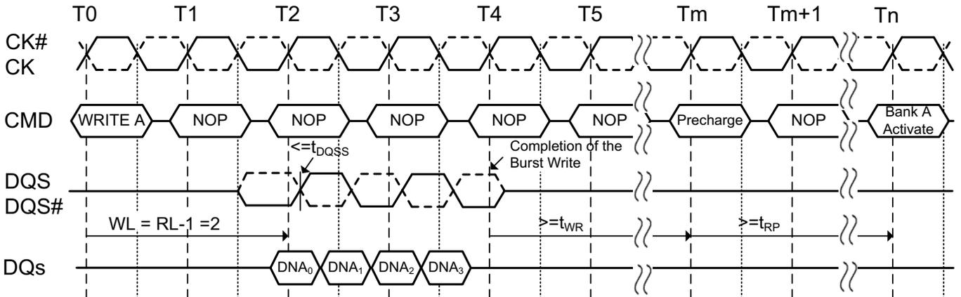
**Figure 29. Burst write followed by burst read:
