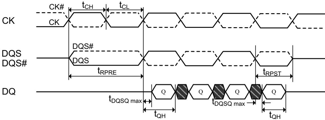
**Figure 21. Data input (write) timing**
