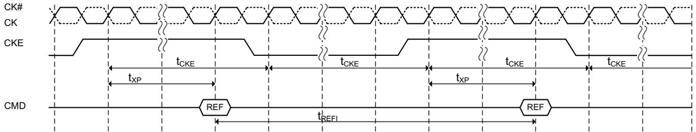
NOTE: The pattern shown above can repeat over a long period of time. With this pattern, DRAM guarantees all AC and DC timing & voltage specifications and DLL operation with temperature and voltage drift
