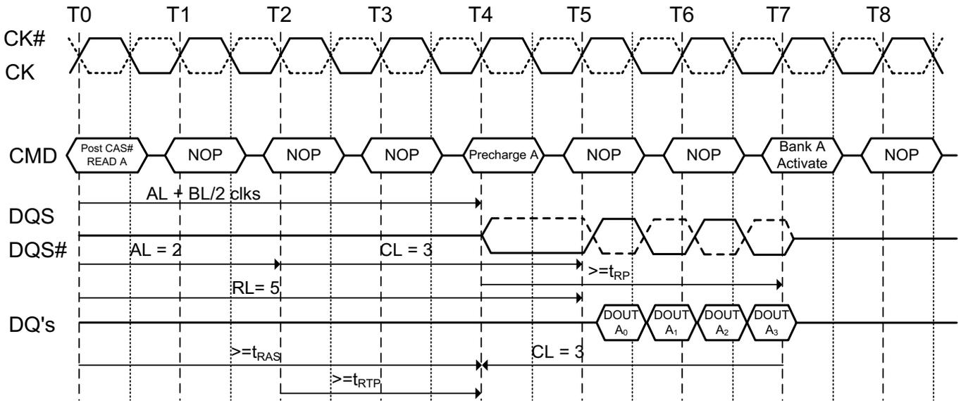
**Figure 36. Burst read operation followed by precharge:**
