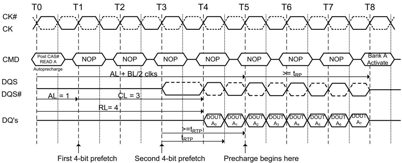
**Figure 41. Burst read operation with auto precharge:
