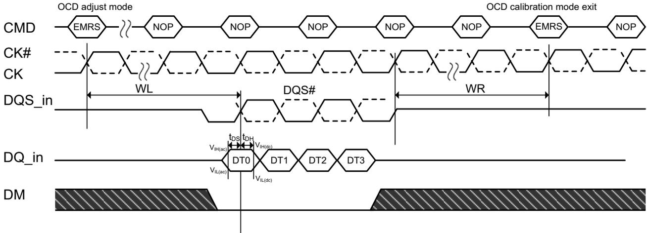
**NOTE 1:** For proper operation of adjust mode,  $WL = RL - 1 = AL + CL - 1t_{CK}$  and  $t_{DS}/t_{DH}$  should be met as shown in the figure.
