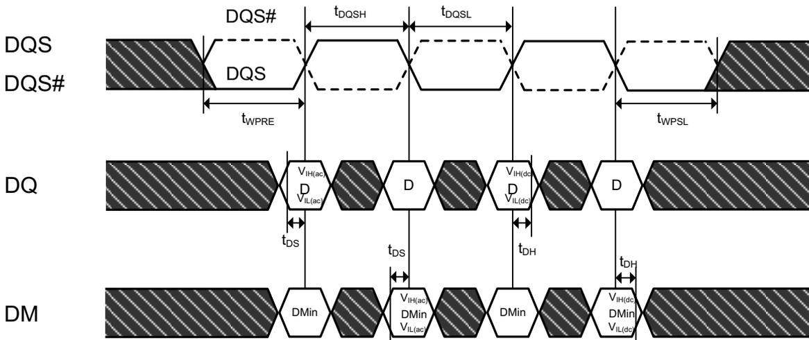
**Figure 22. Burst read operation: RL=5 (AL=2, CL=3, BL=4)**
