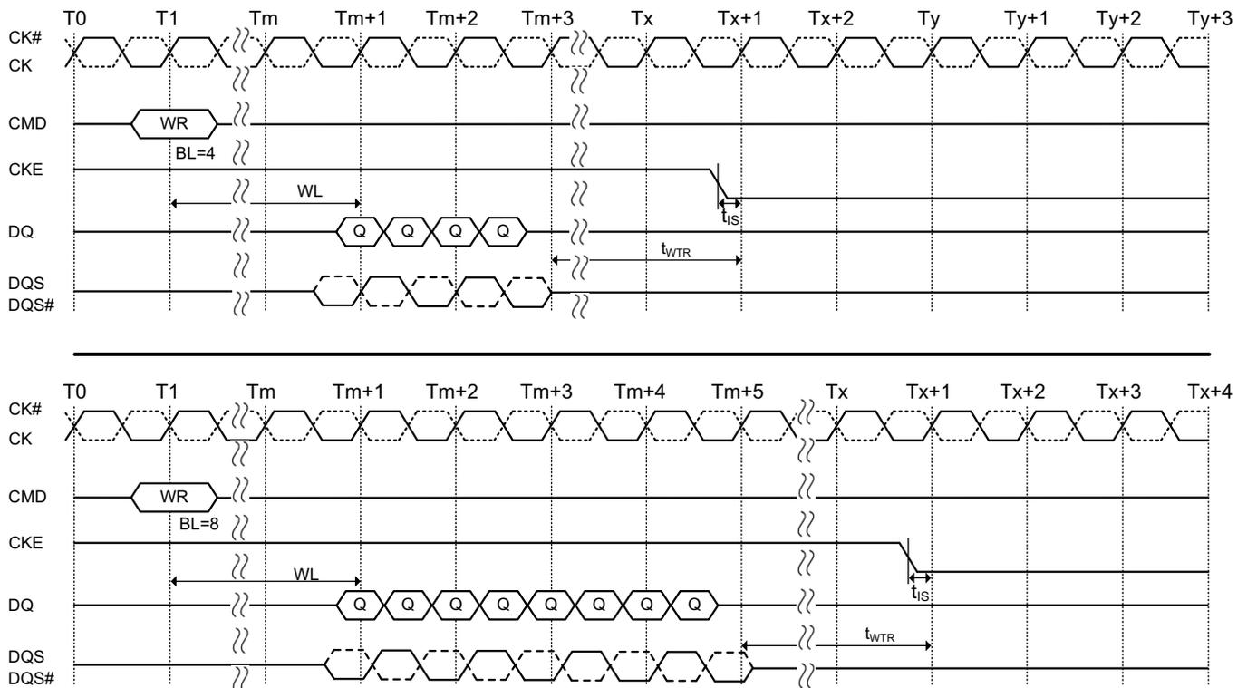
**Figure 54. Write with autoprecharge to power-down entry**
