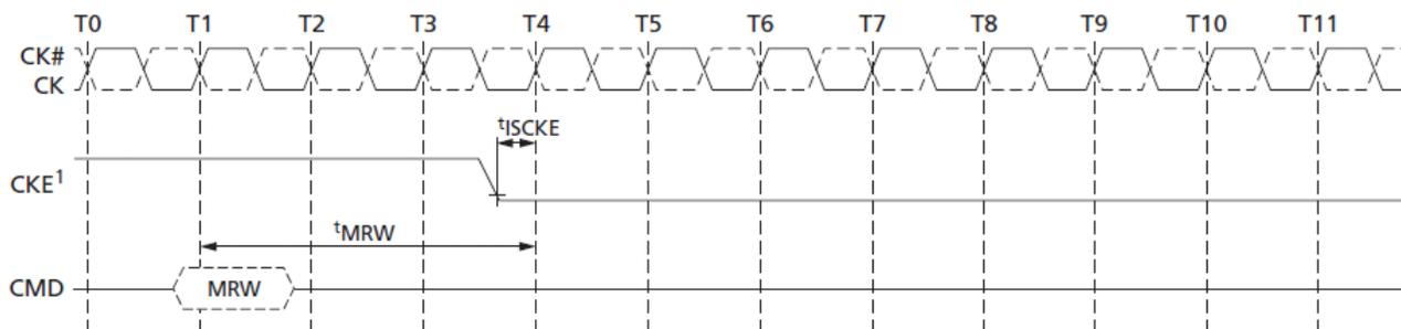
Note : 1. CKE can be registered LOW  $tMRW$  after the clock on which the MRW command is registered.
