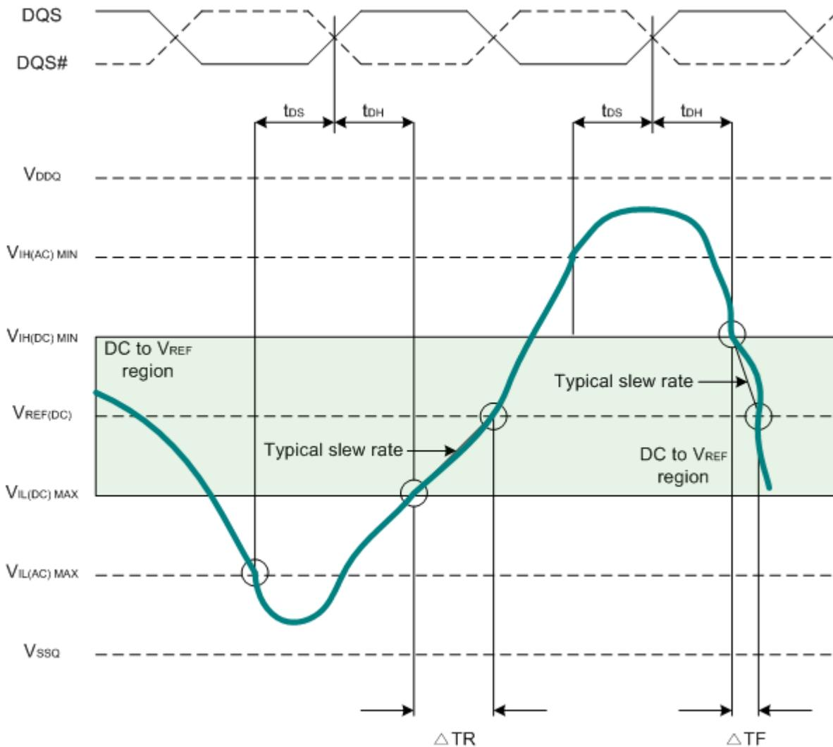
$$\text{Hold slew rate falling signal} = \frac{V_{IH(DC)min} - V_{REF(DC)}}{\Delta TF}$$
