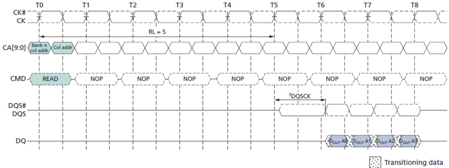
Figure 7 : Burst READ – RL = 3, BL = 8,  $t_{DQSCK} < t_{CK}$
