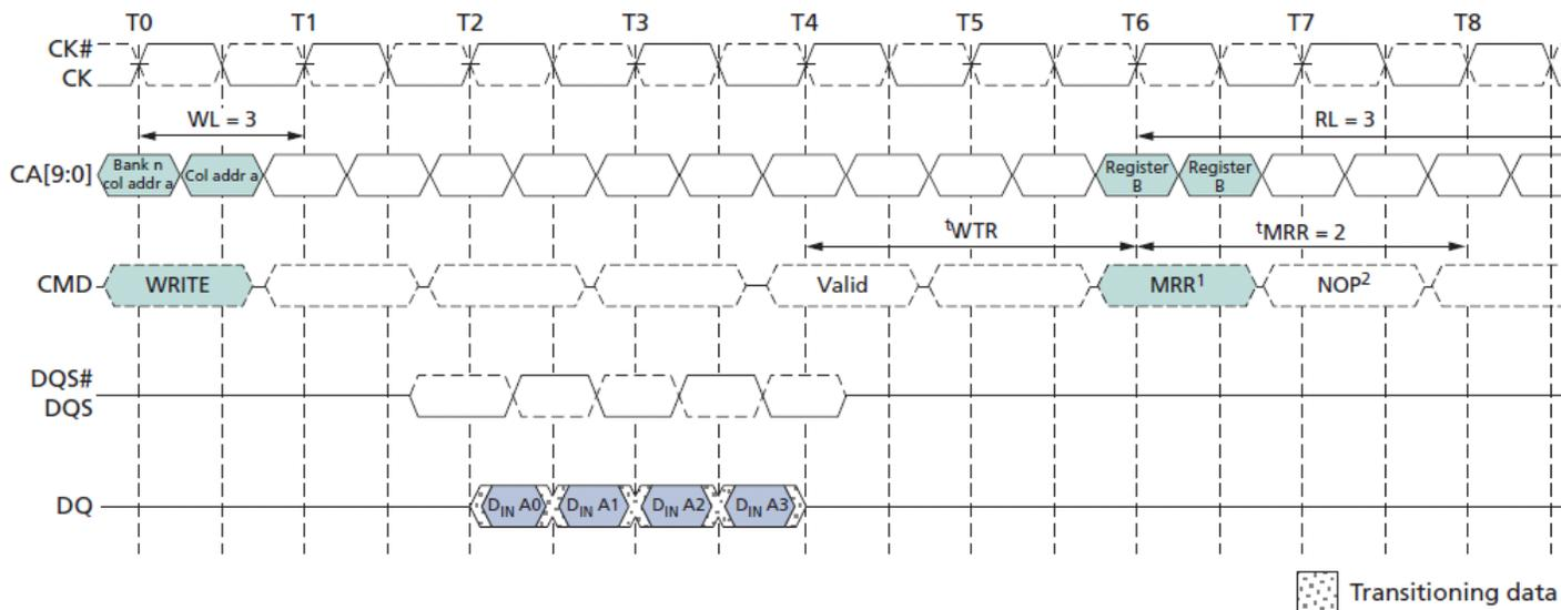
Notes : 1. The minimum number of clock cycles from the burst WRITE command to the MRR command is  $[WL+1+BL/2+RU(tWTR/tCK)]$ .
