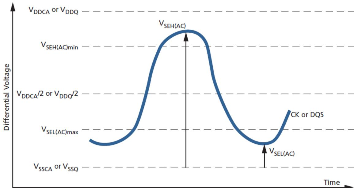
Note that while CA and DQ signal requirements are referenced to VREF, the single-ended components of differential signals also have a requirement with respect to VDDQ/2 for DQS, and VDDCA/2 for CK.
