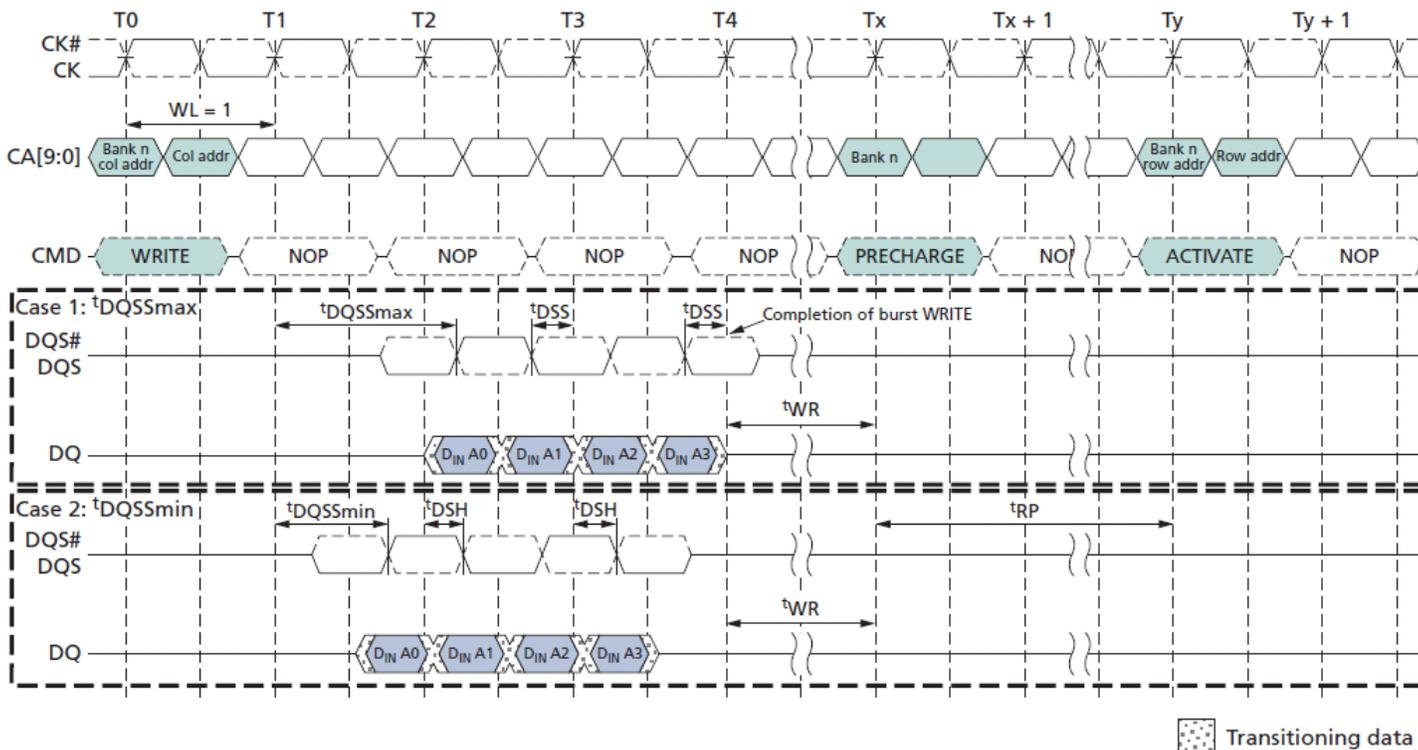
**Figure 16: Burst WRITE Followed by Burst READ – RL = 3, WL = 1, BL = 4**
