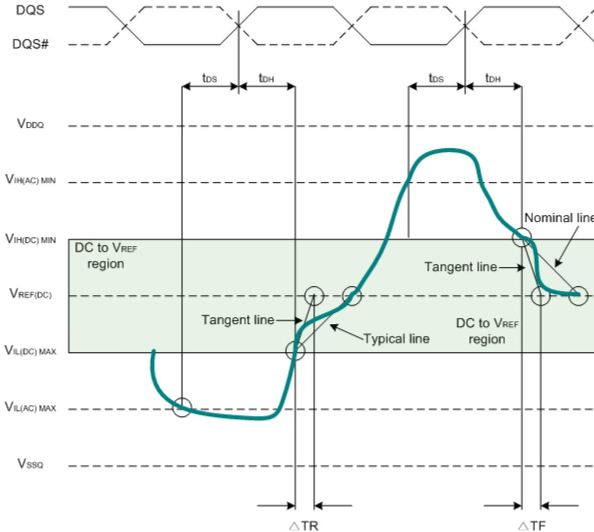
$$\text{Hold slew rate falling signal} = \frac{\text{tangent line } [V_{IH(DC)min} - V_{REF(DC)}]}{\Delta TF}$$
