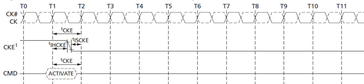
Note : 1. CKE can go LOW at  $t_{HCKE}$  after the clock on which the ACTIVATE command is registered.
