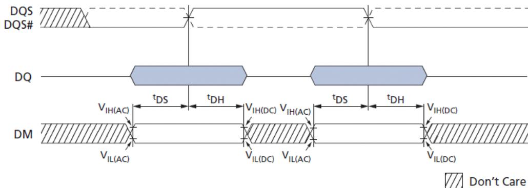
**Figure 22: Write Data Mask – Second Data Bit Masked**
