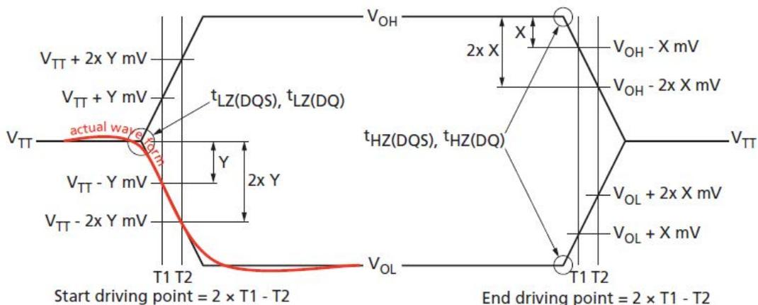
7. Measured from the point when DQS/DQS# begins driving the signal, to the point when DQS/DQS# begins driving the first rising strobe edge.
