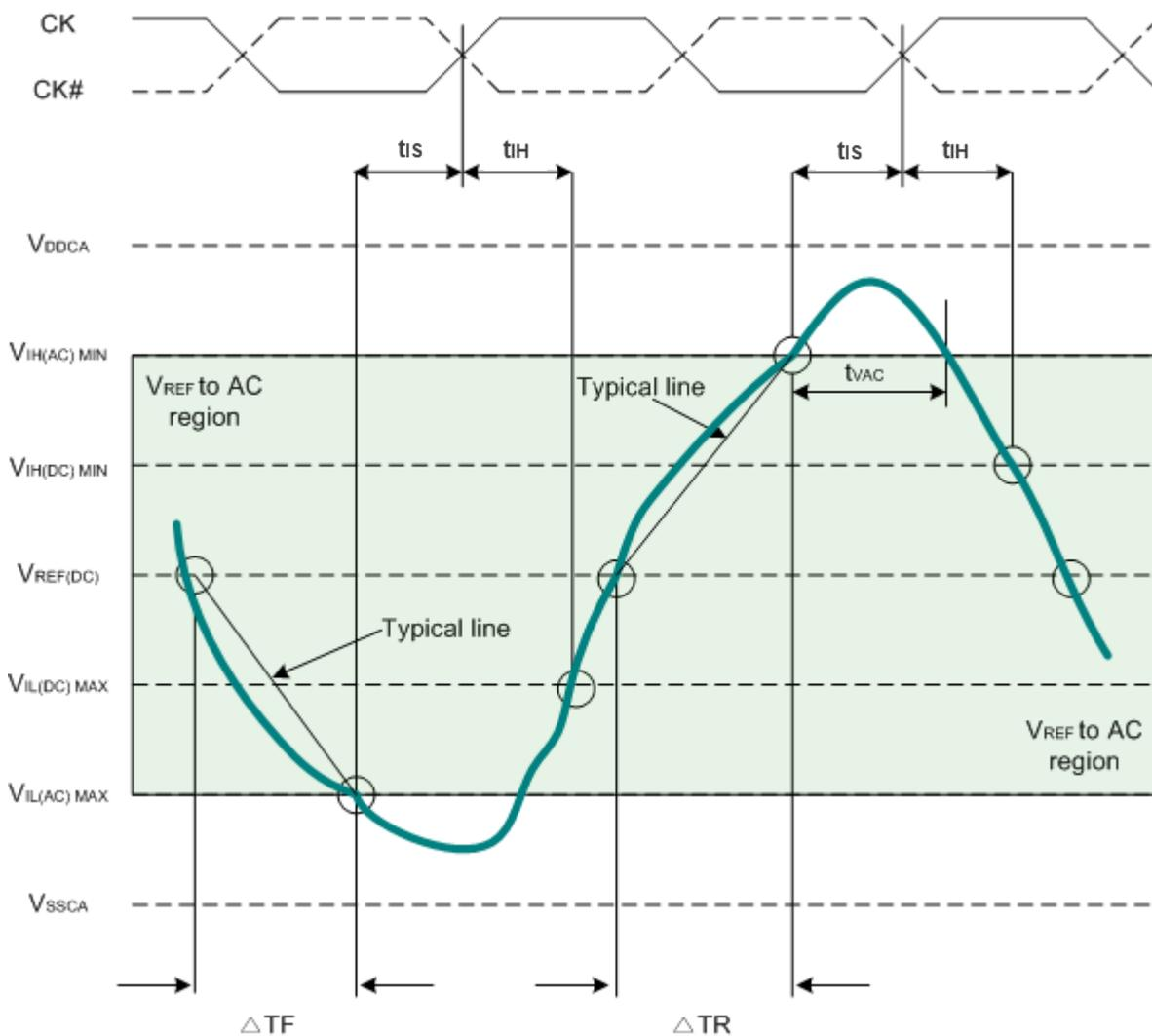
Figure 72: Typical Slew Rate – t<sub>IH</sub> for CA and CS# Relative to Clock
