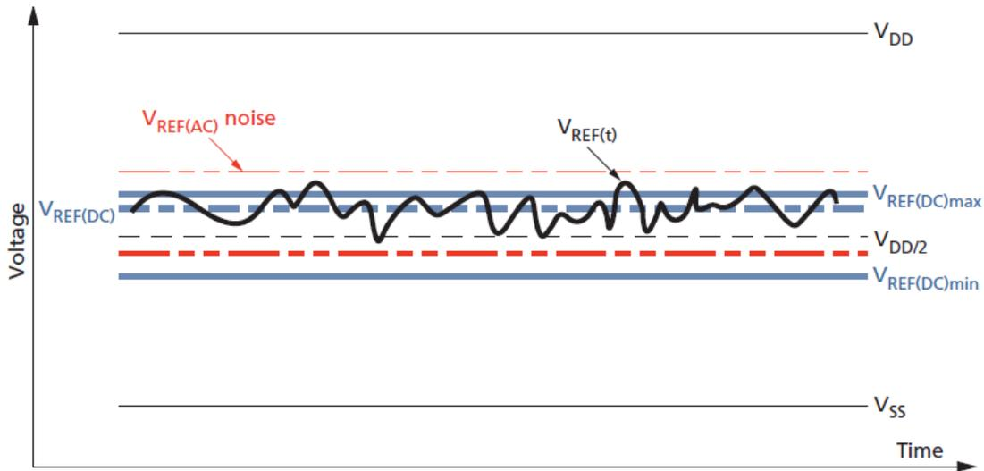
The voltage levels for setup and hold time measurements VIH(AC), VIH(DC), VIL(AC), and VIL(DC) are dependent on VREF. VREF DC variations affect the absolute voltage a signal must reach to achieve a valid HIGH or LOW, as well as the time from which setup and hold times are measured. When VREF is outside the specified levels, devices will function correctly with appropriate timing deratings as long as:
