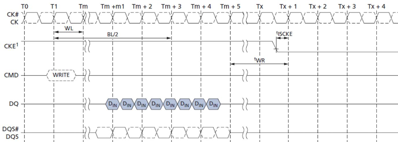
Note : 1. CKE can be registered LOW at  $(WL + 1 + BL/2 + RU(t_{WR}/CK))$  clock cycles after the clock on which the WRITE command is registered.
