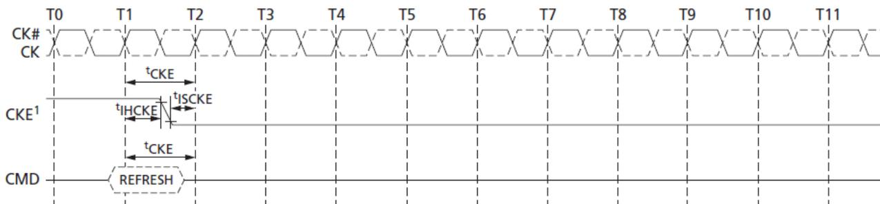
Note : 1. CKE can go LOW  $t_{HCKE}$  after the clock on which the REFRESH command is registered.
