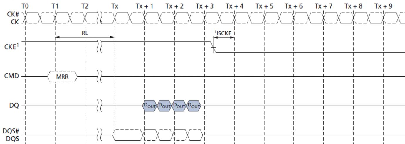
Note : 1. CKE can be registered LOW at  $(RL + RU(tDQSCK/tCK) + BL/2 + 1)$  clock cycles after the clock on which the MRR command is registered.
