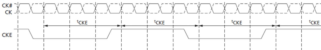
**Figure 45: REFRESH-to-REFRESH Timing in CKE Intensive Environments**
