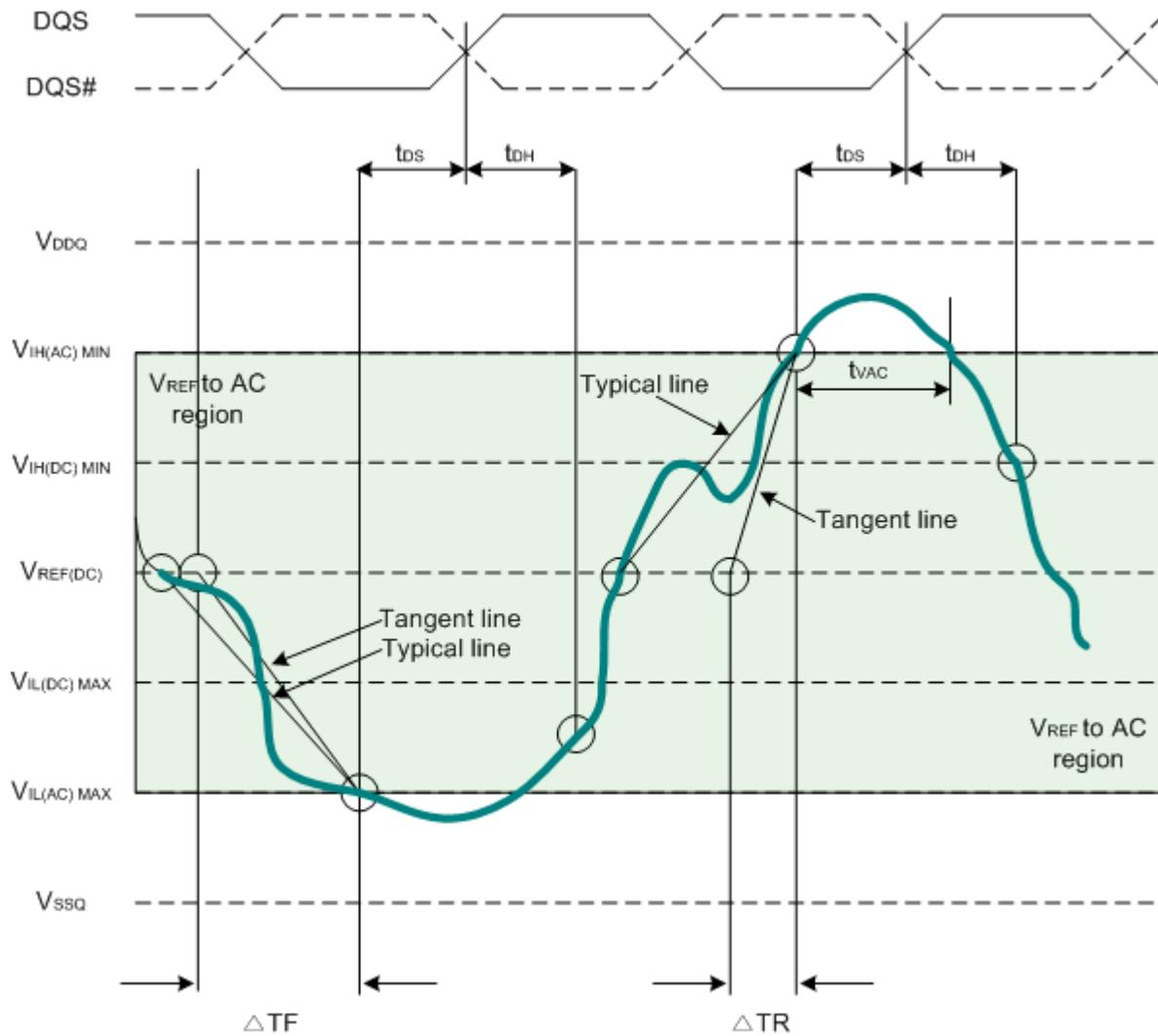
$$\text{Setup slew rate falling signal} = \frac{\text{tangent line } [V_{REF(DC)} - V_{IL(AC)max}]}{\Delta TF}$$
