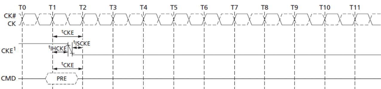
Note : 1. CKE can go LOW  $t_{HCKE}$  after the clock on which the PRECHARGE command is registered.
