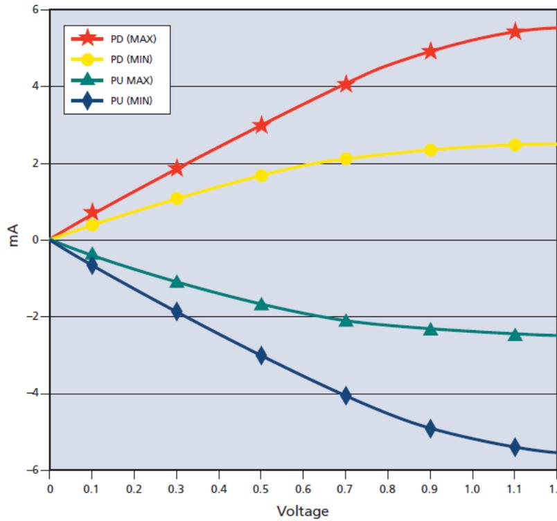
Figure 69: Output Impedance = 240 Ohms, I-V Curves After Calibration
