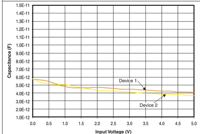
Figure 3. Capacitance vs Input Voltage at T<sub>A</sub> = 27°C
