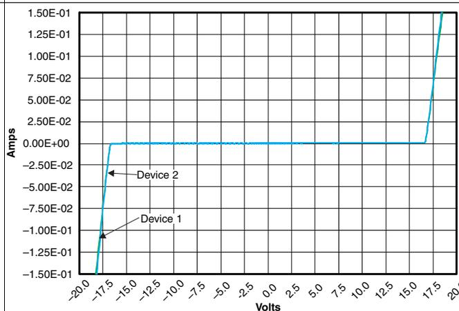
Figure 4. Diode Breakdown Voltage Data at T<sub>A</sub> = 27°C
