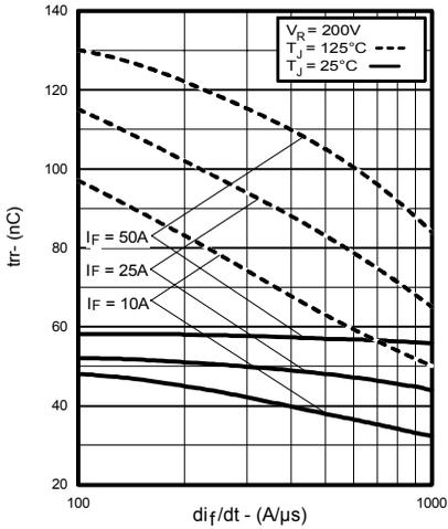
**Fig. 5 - Typical Reverse Recovery vs.  $di_f/dt$**
