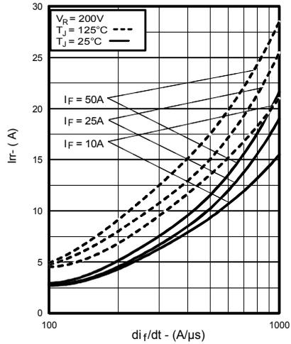
**Fig. 6 - Typical Recovery Current vs.  $di_f/dt$**
