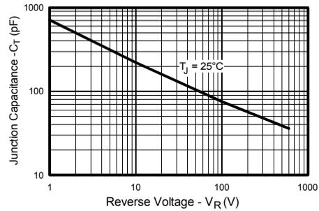
**Fig. 3 - Typical Junction Capacitance vs. Reverse Voltage**
