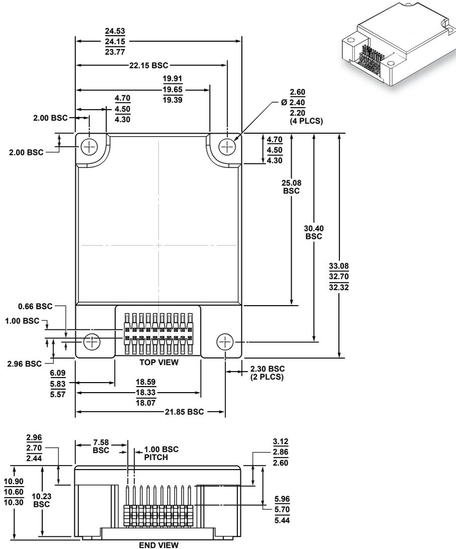
Figure 25. 20-Lead Module with Connector Interface (ML-20-1)
