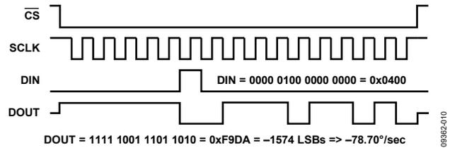
Figure 12. Example SPI Read, Second 16-Bit Sequence
