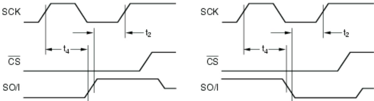
Figure 12. Input Data Timing Diagram
