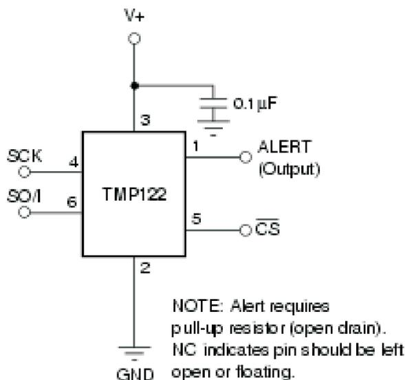
Figure 1. Typical Connections
