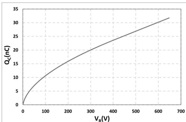
Fig. 6 Typical Total Capacitive Charge
