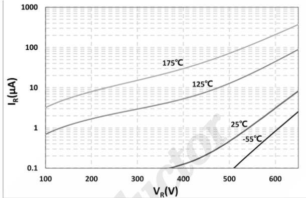
Fig. 2 Reverse Characteristics
