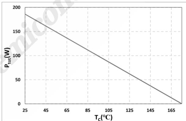
Fig. 4 Typical Power Derating
