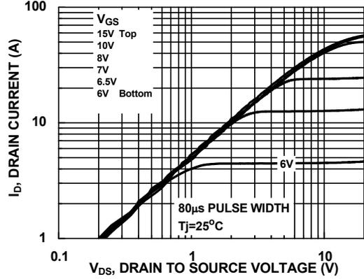
Figure 8. Saturation Characteristics
