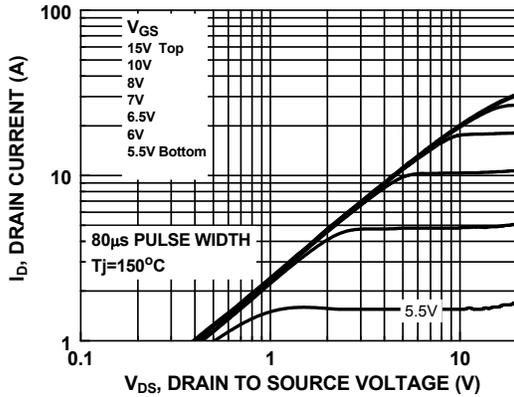
Figure 9. Saturation Characteristics
