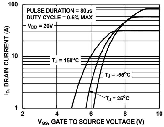
Figure 6. Transfer Characteristics
